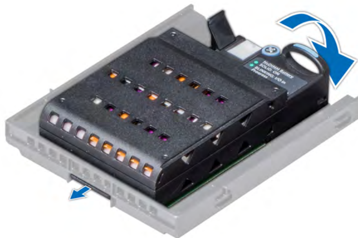
Figure 45. Installing NVDIMM-N battery into the bracket
