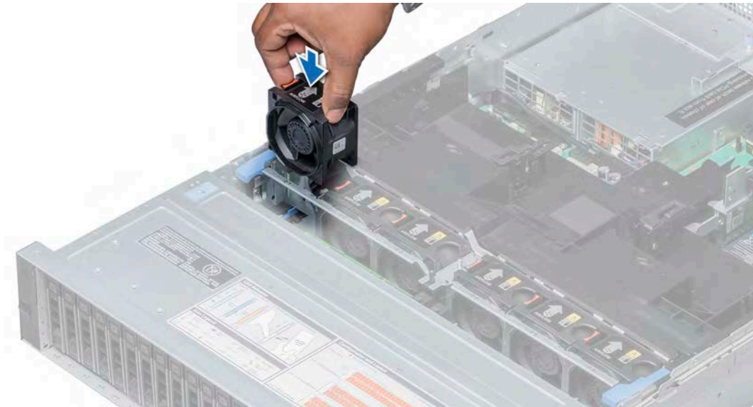
Figure 37. Installing cooling fan
