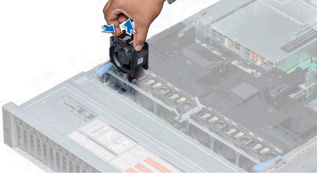
Figure 36. Removing cooling fan
