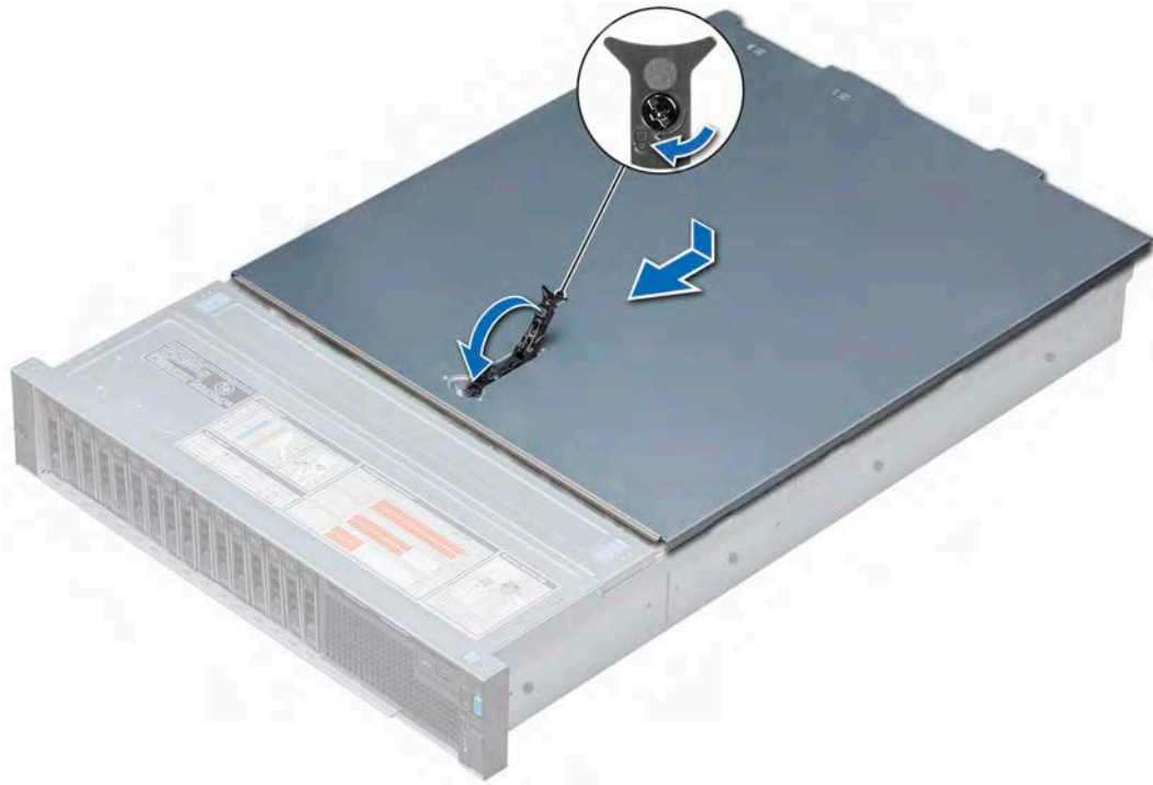
Figure 27. Installing system cover
