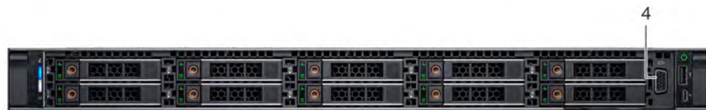
Figure 4. Front view of 10 x 2.5 inch drive system
