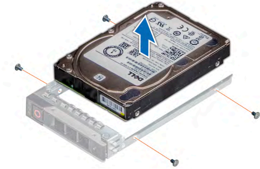
Figure 79. Removing the drive from the drive carrier
