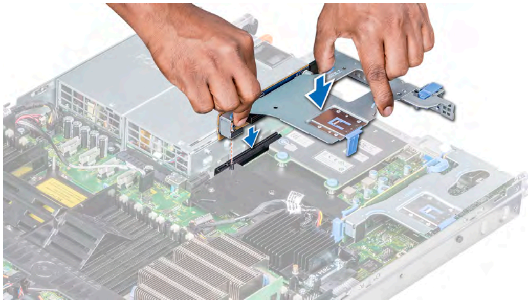
Figure 53. Installing the expansion riser 2B
