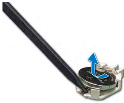
Figure 98. Removing the system battery
