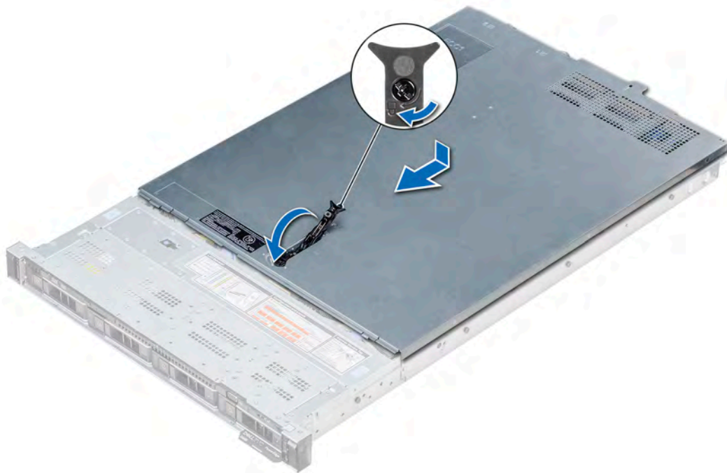
Figure 24. Installing the system cover
