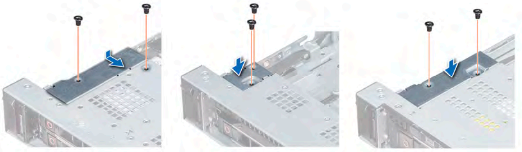
Figure 113. Installing the cable cover
