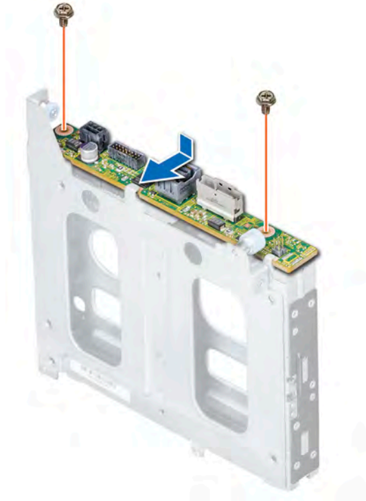
Figure 88. Installing the 2.5 inch drive rear backplane
