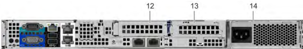
Figure 13. Back view of the system with 2 risers
