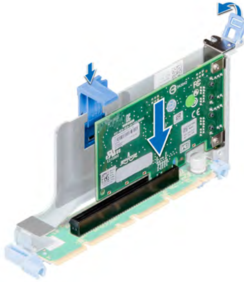
Figure 62. Installing an expansion card into the expansion riser 1B
