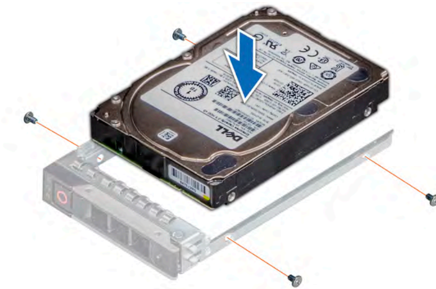
Figure 80. Installing a drive into the drive carrier
