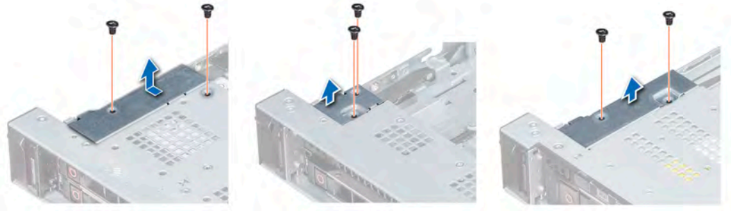
Figure 110. Removing the cable cover
