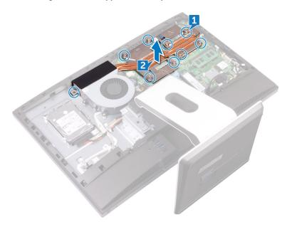
NOTE: Computers that ship with only integrated graphics processors are shipped with 5 captive screws
