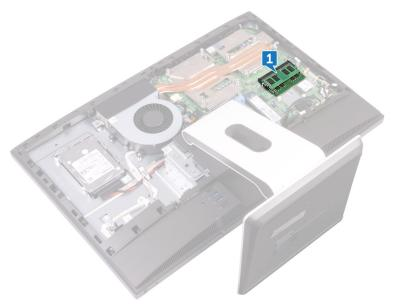
2 Using your fingertips, spread apart the securing clips at each end of the memory-module slot until the memory module pops up.
