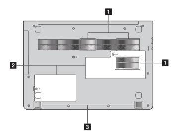
**1 Ventilation slots** Dissipate internal heat.
