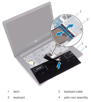
**5** Lift the keyboard, along with the cable, off the palm-rest assembly.
