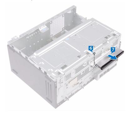
Remove the three screws (M2xL2) that secure the optical-drive bracket to the optical drive.
