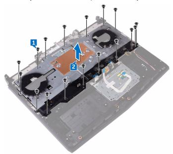
3 Lift the keyboard at an angle and remove it from the tabs on the palm-rest assembly.
