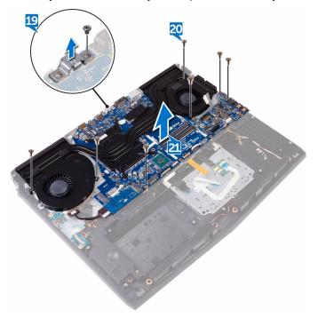
22 Remove the <u>heat-sink assembly</u>.
