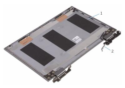
display back-cover and antenna 2 antenna cables assembly
