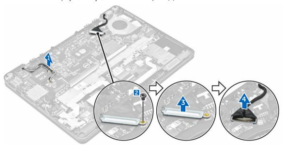
**4.** Disconnect speaker cable [1], LED board cable [2], touchpad and system board cable [3,4], and power connector port cable [5].
