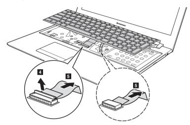
Note: Select models do not have the keyboard backlight cable (the dashed area).
