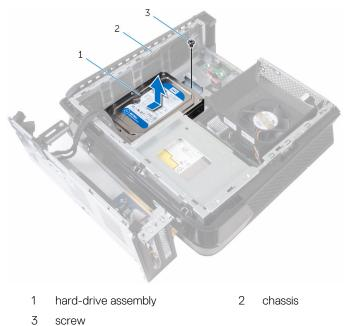
7 Remove the screws that secure the hard-drive bracket to the hard-drive assembly.
