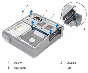
**3** Lift the riser cage from the chassis and remove the graphics-card power cables from the routing guide on the riser cage.
