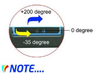
The built-in rotating camera must be returned to its original position for the display panel to close properly.
