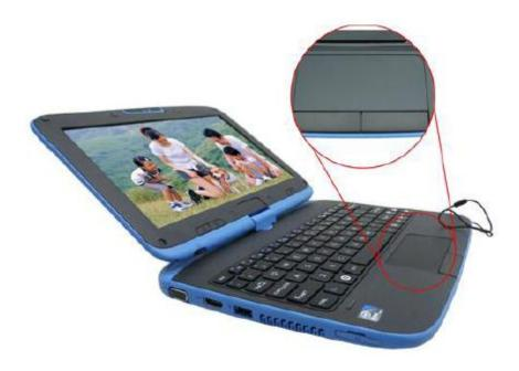
The touchpad is a rectangular electronic panel located just below your keyboard. You can use the static-sensitive panel of the touchpad and slit it to move the cursor. You can use the buttons below the touchpad as left and right mouse buttons.
