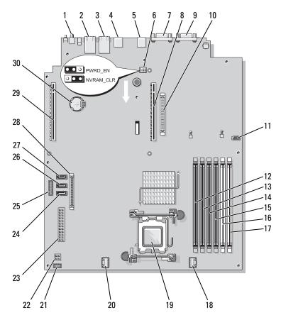
Figure 6-1. System Board Connectors
