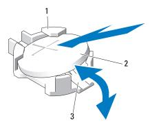
1 positive side of battery connector 2 system battery
