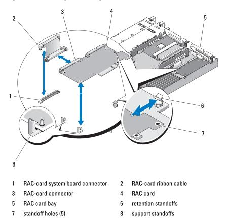
Figure 3-14. Removing and Installing a RAC Card
