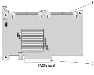
1 SAS6ir card cable connectors 2 center riser connector
