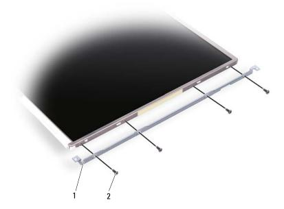
1 display panel bracket (1 left, 1 right) 2 screw (8 total; 4 on each side)
