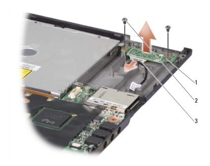
1 wireless sniffer board 2 M2 x3-mm screw (2) 3 wireless sniffer board cable connector
