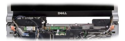
**9** Make note of the cable routing and carefully dislodge the Mini-Card antenna cables from their routing guides and pull the cables with their connectors through the system board so that they are clear of the computer base.
