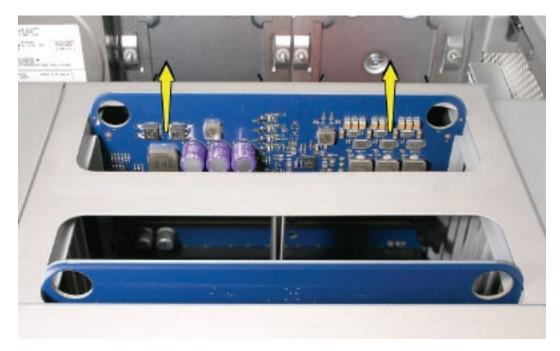
4. Open the ejectors on the DIMM slot by pushing them out to the sides, and remove the DIMM from the riser card.
