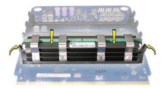
2. Insert the replacement riser card into position in the memory cage, pushing slightly until the card is seated in its logic board memory slot.
