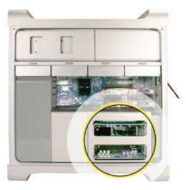
3. Holding the memory riser card by the two finger holes, pull it out of the memory cage and place the card DIMM-side-up on a soft, clean cloth.
