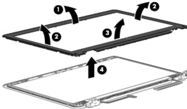
**20.** If it is necessary to replace the display panel:
