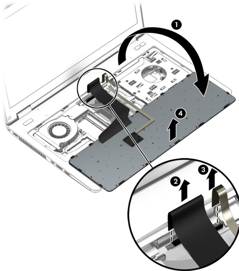
Reverse this procedure to install the keyboard.
