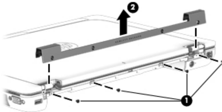
9. Remove the two Torx T8M2.5×4.5 screws that secure the display assembly to the base enclosure.
