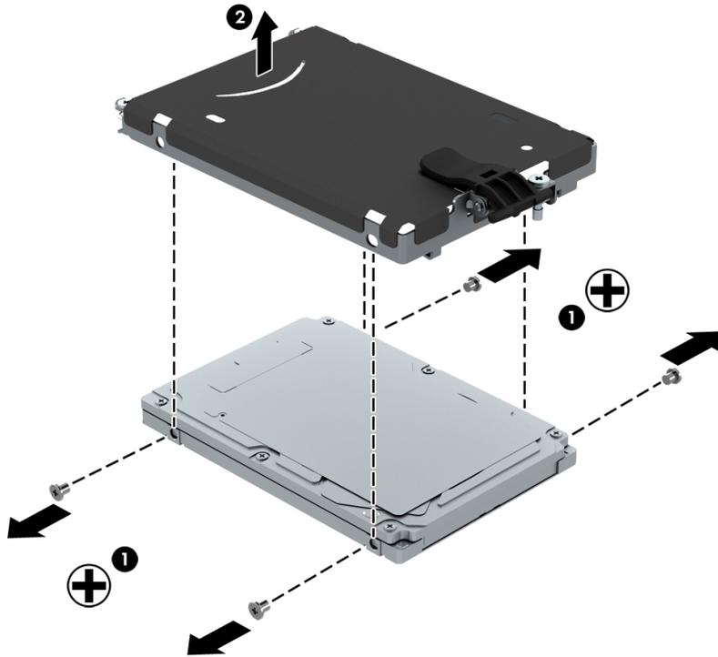
Reverse this procedure to install the hard drive.
