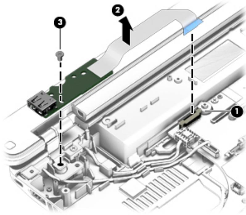
4. Remove the USB board and cable.
