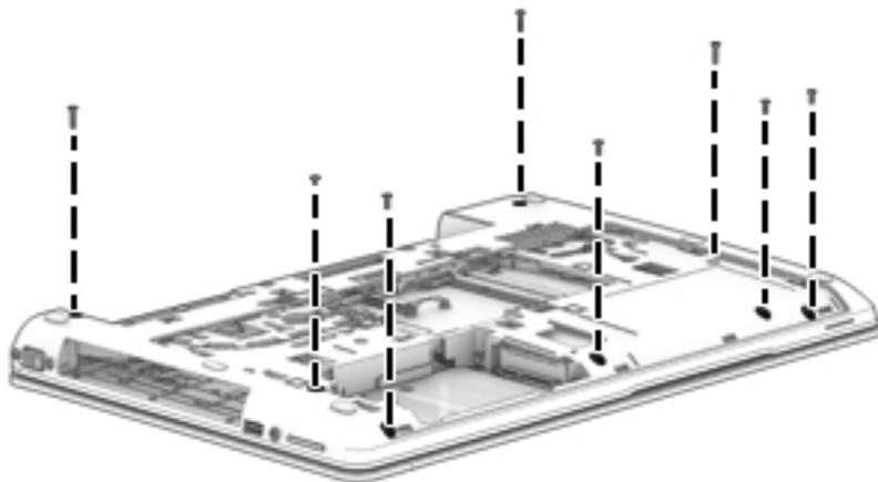
4. Remove the following screws that secure the top cover to the computer:
