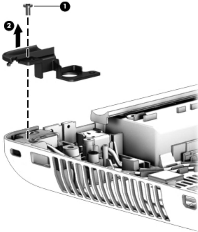
3. Remove the Phillips PM2.0×5.5 screw (1) that secures the security cable lock bracket to the base enclosure.
