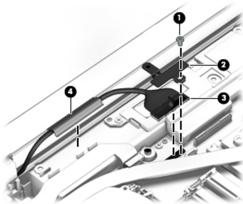
16. Release the wireless antenna cables from the routing channels built into the base enclosure.
