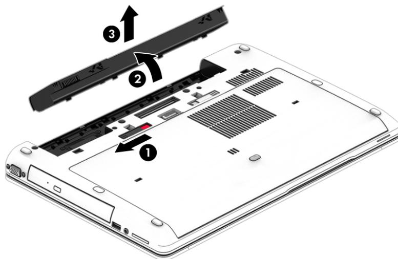
Reverse this procedure to install the battery.
