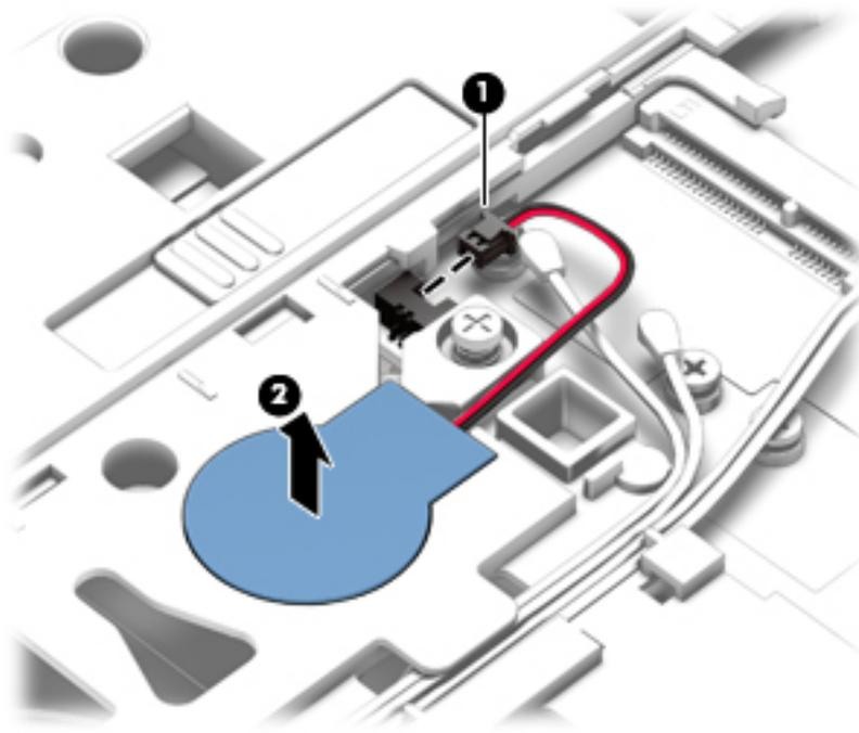
3. Remove the RTC battery and cable.
