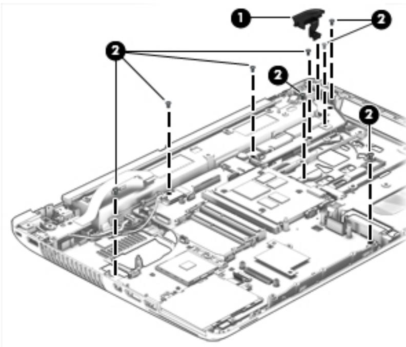
5. Lift up on the left side of the system board **(1)** until it rests at an angle.
