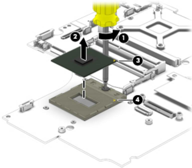
Reverse this procedure to install the processor.
