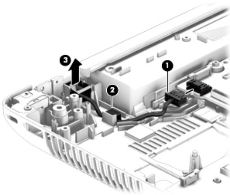
4. Remove the power connector cable.
