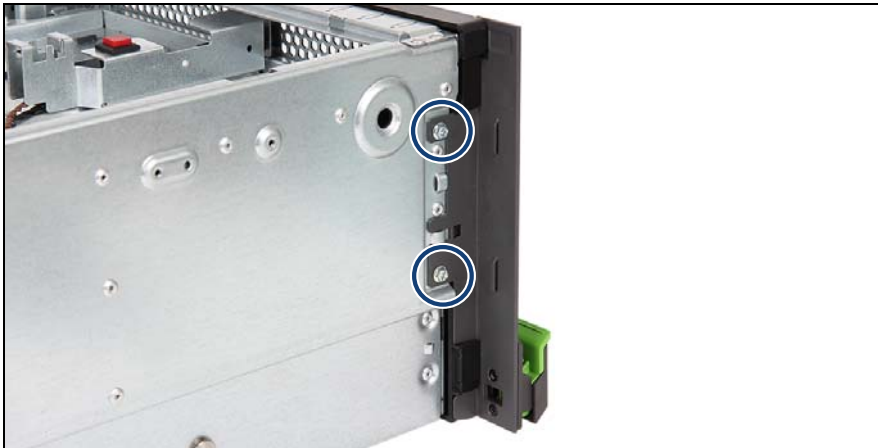
Figure 7: Removing the rack front cover (A)
