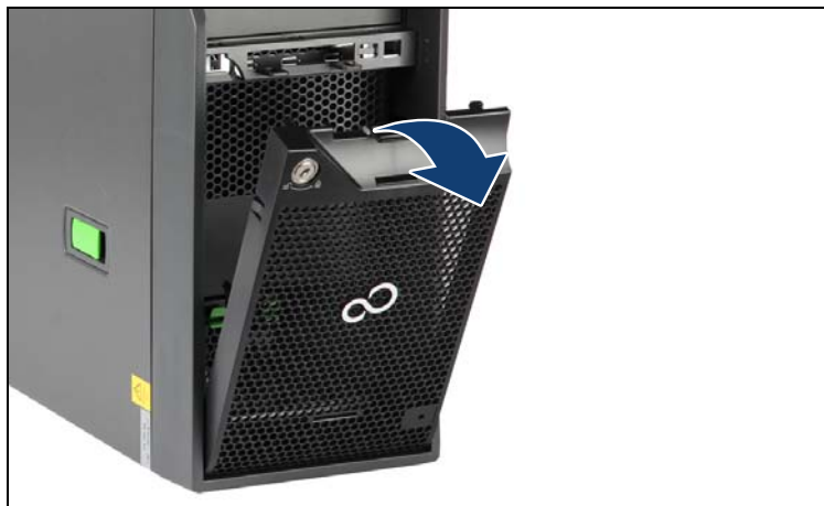
Figure 13: Removing the HDD bay cover
