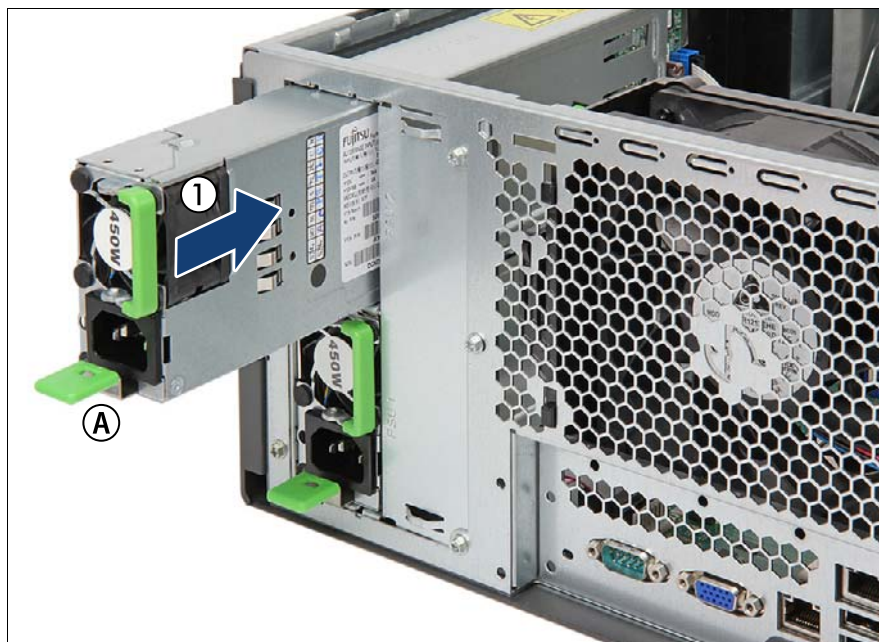
Figure 48: Installing a hot-plug PSU
