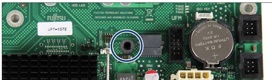
Figure 260: Removing the UFM (B)
