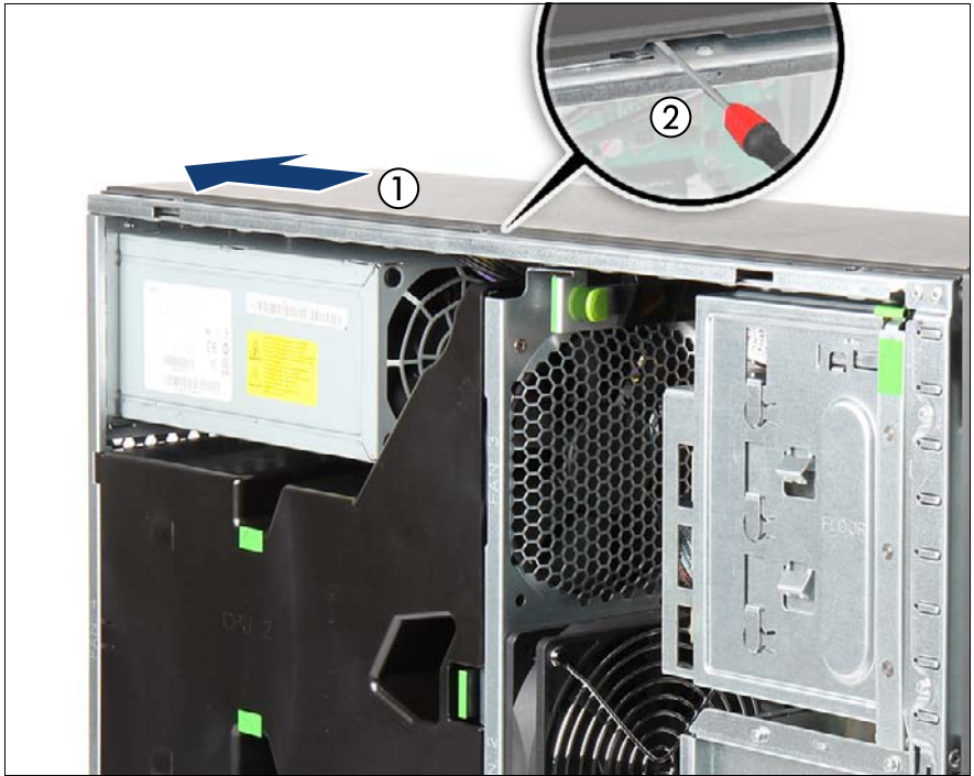
Figure 288: Removing the right side cover (B)
