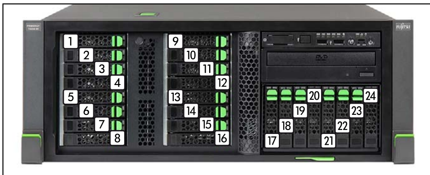
Figure 67: Naming scheme with 24 2.5-inch HDDs (6 SAS backplanes)
