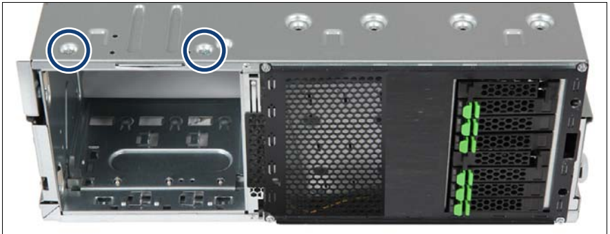
Figure 296: Securing the accessible drive cage (B)
