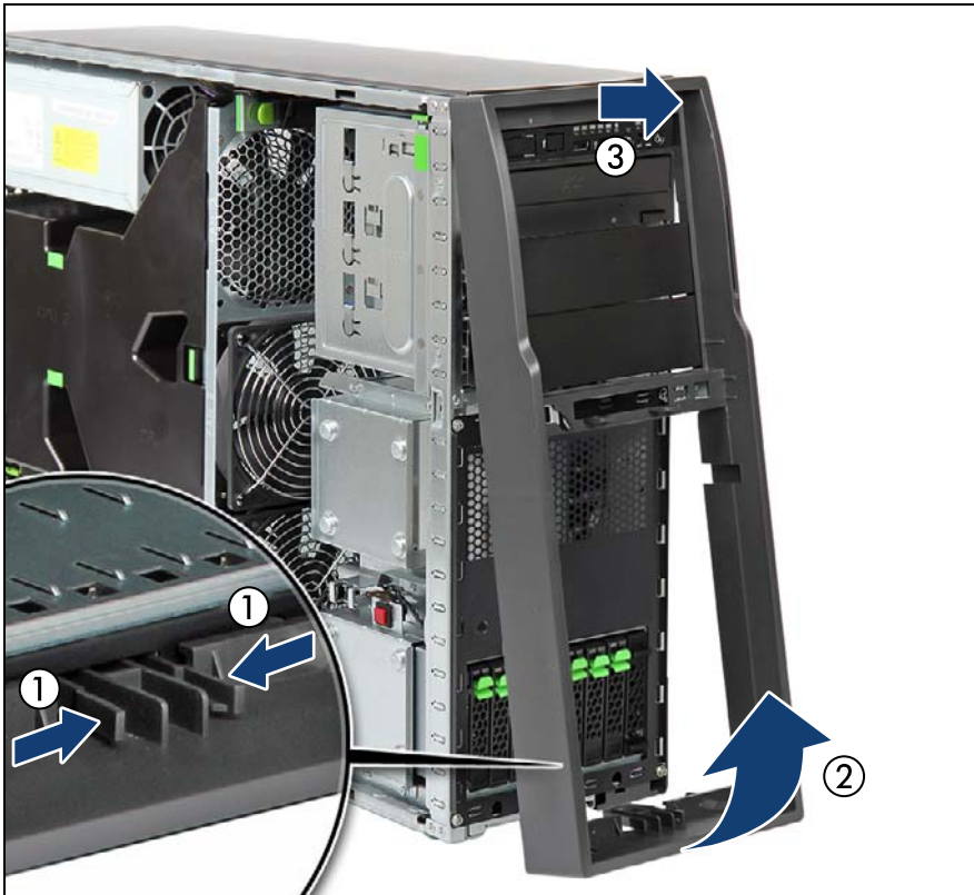
Figure 15: Removing the front cover (tower server)
