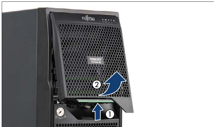
Figure 12: Removing the accessible drive bay cover
