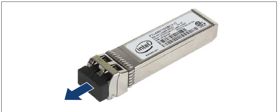
Figure 148: Removing the protective optical port plug
