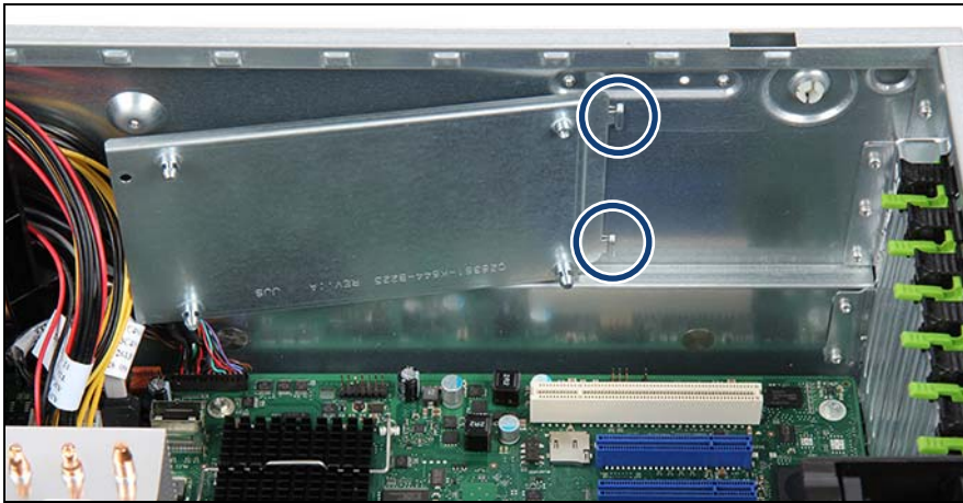
Figure 122: Installing the carrier (A)
