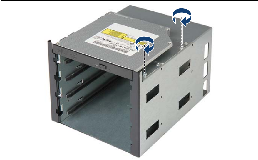
Figure 239: Installing the slimline ODD on the HDD extension box (B)
