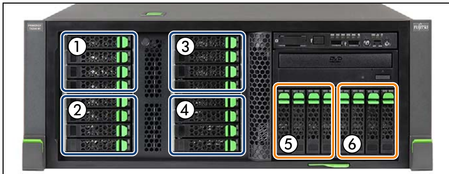
Figure 60: 2.5-inch SAS backplanes - maximum configuration, rack version
