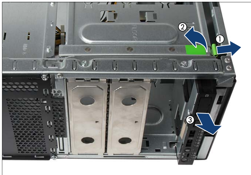
Figure 247: Removing the front panel module
