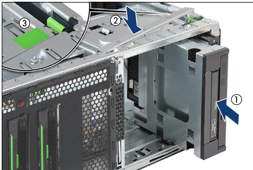
Figure 226: Inserting the Multibay box
