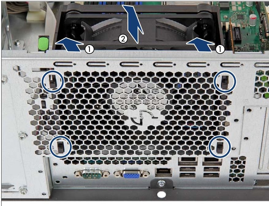
Figure 138: Removing the rear fan (B)
