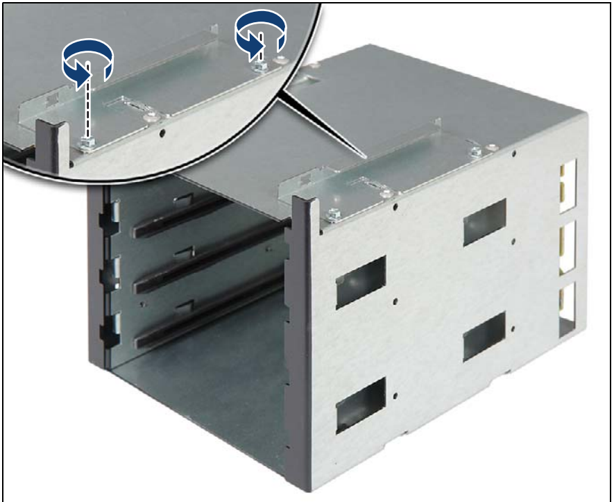
Figure 235: Removing the slimline ODD mounting bracket
