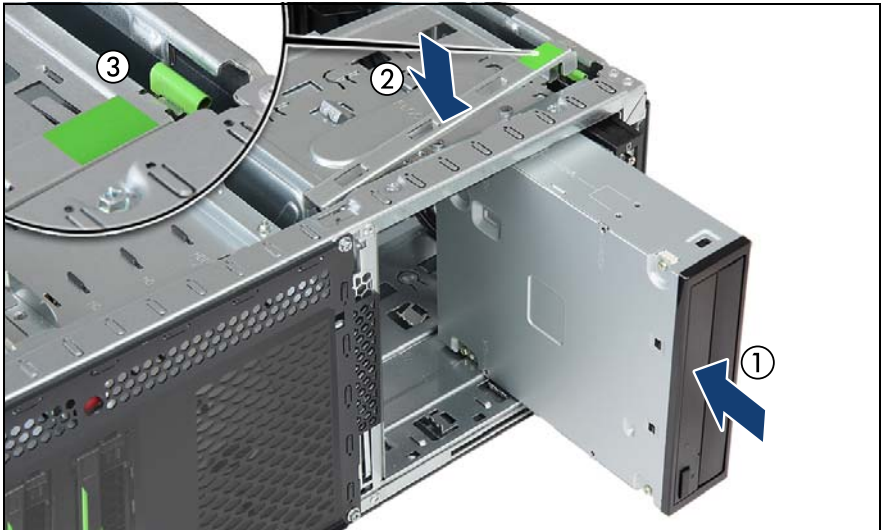
Figure 216: Inserting the accessible drive
