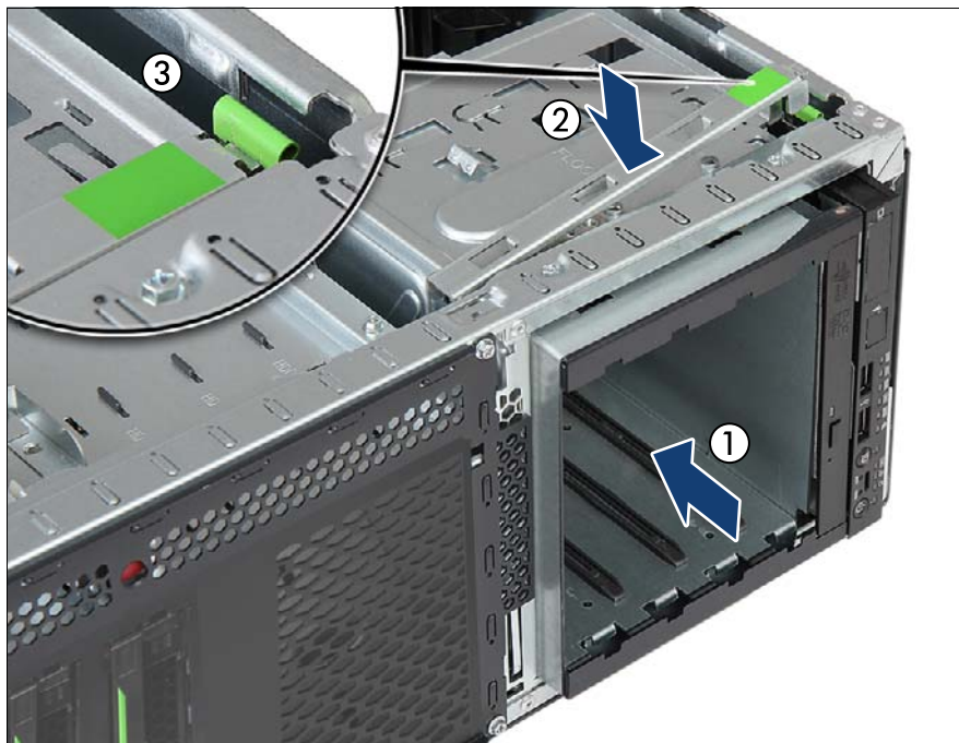
Figure 116: Inserting the HDD extension box (example 4x 3.5-inch HDD extension box)
