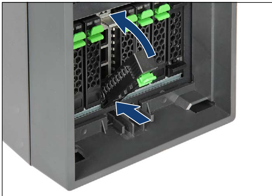
Figure 70: Inserting the 2.5-inch HDD / SSD module
