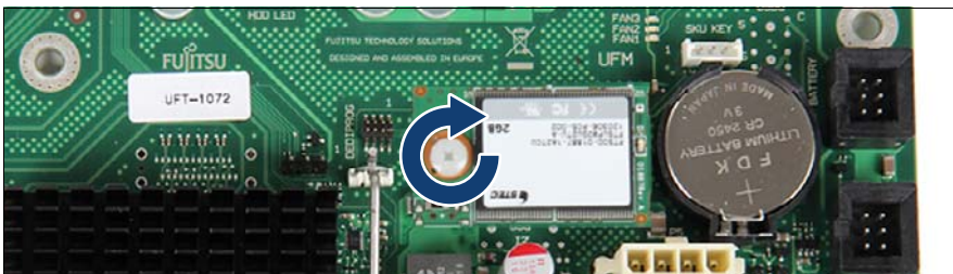
Figure 263: Installing the UFM (B)
