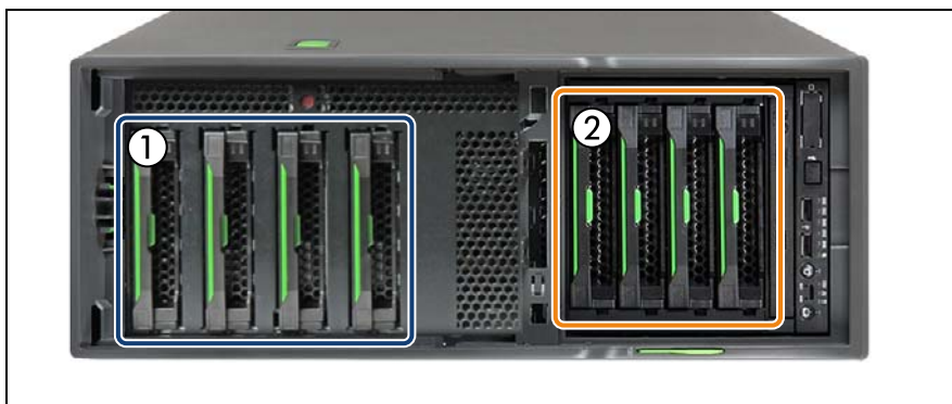
Figure 88: 3.5-inch SAS backplanes - maximum configuration, tower server
