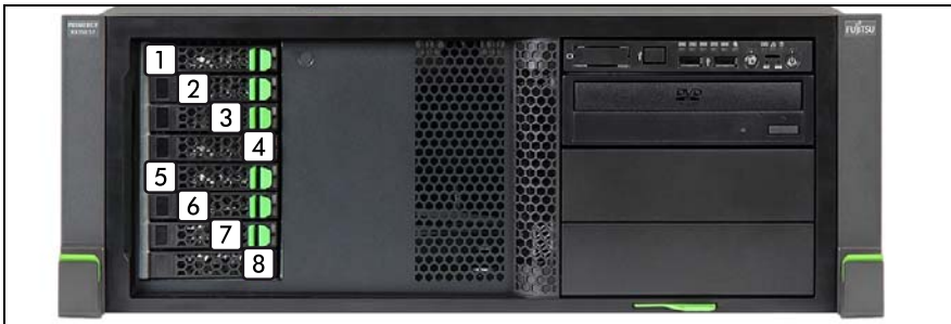
Figure 63: Naming scheme with 8 2.5-inch HDDs (2 SAS backplanes)
