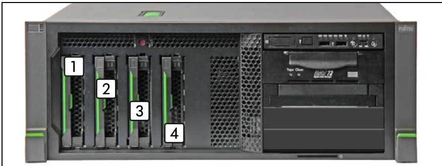
Figure 90: Naming scheme with 4 3.5-inch HDDs (1 SAS backplane)
