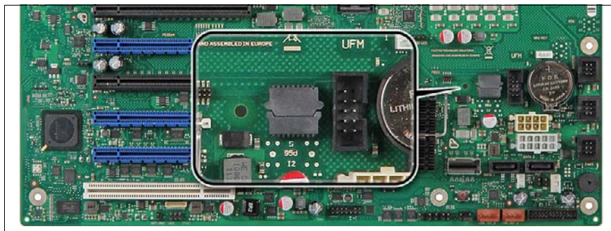
Figure 257: UFM mounting location
