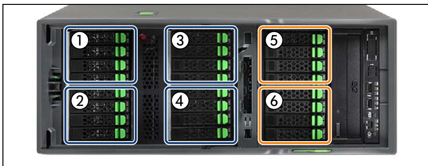
Figure 61: 2.5-inch SAS backplanes - maximum configuration, tower version
