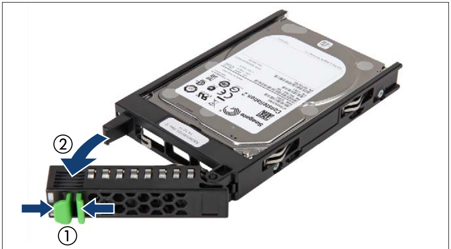
Figure 69: Opening the 2.5-inch HDD / SSD module locking lever
