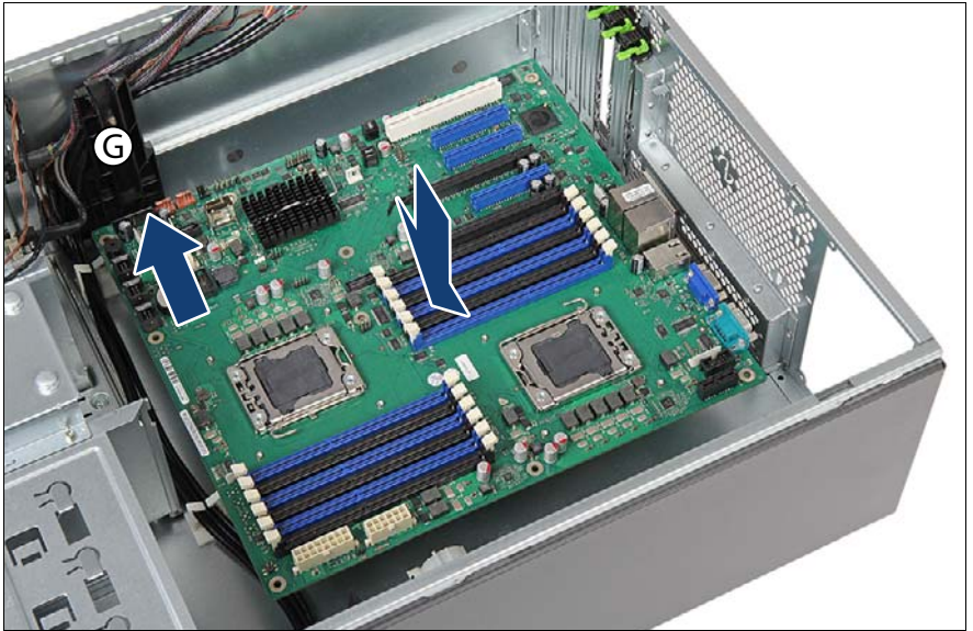
Figure 283: Installing the system board (A)
