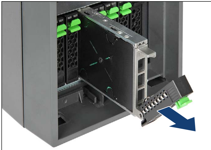
Figure 71: Removing a 2.5-inch HDD / SSD module
