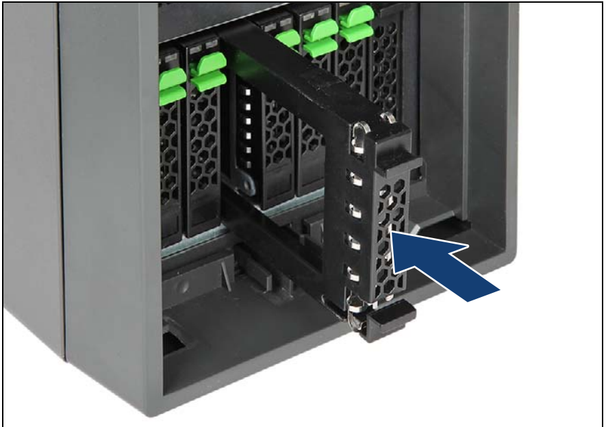
Figure 72: Installing a 2.5-inch HDD / SSD dummy module
