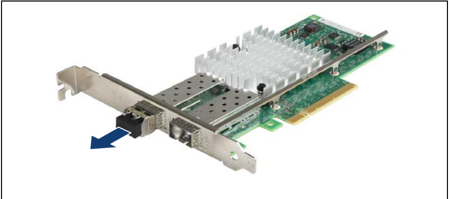
Figure 154: Removing the protective optical port plug
