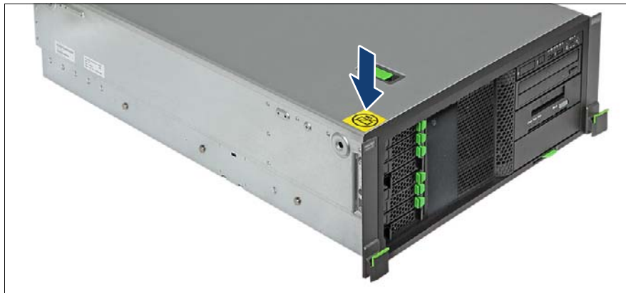
Figure 300: Attaching the caution label
