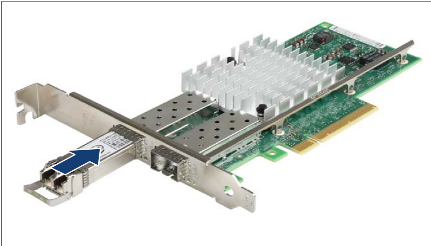
Figure 150: Inserting the SFP+ transceiver module
