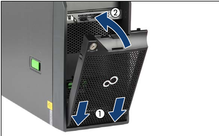
Figure 25: Installing the HDD bay cover
