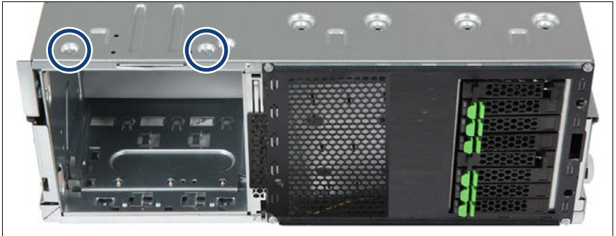
Figure 290: Detaching the accessible drive cage (A)
