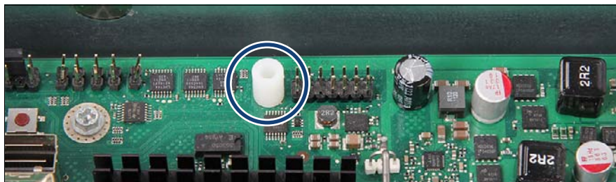
Figure 267: Installing the TPM spacer
