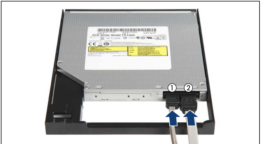
Figure 222: Mounting the slimline ODD in the installation frame (B)
