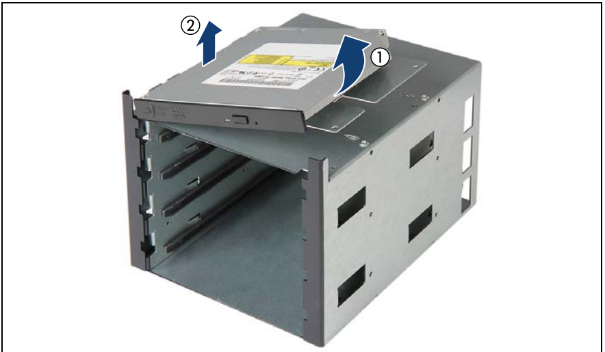
Figure 243: Removing the slimline ODD from the extension box (B)
