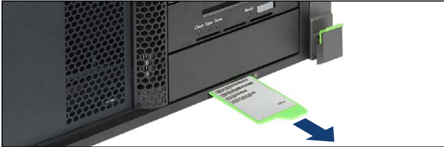
Figure 6: Removing the ID card (rack server)
