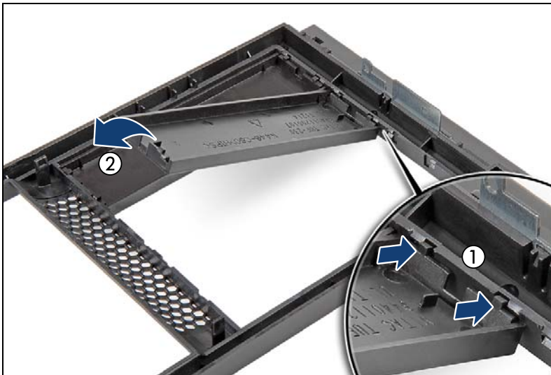
Figure 299: Installing accessible drive dummy covers
