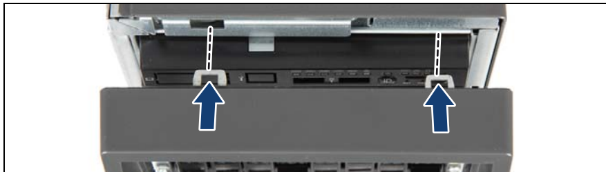
Figure 22: Installing the front cover (tower server) (A)
