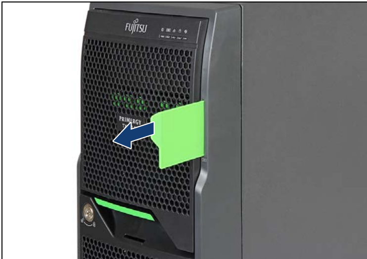
Figure 14: Removing the ID card (tower server)
