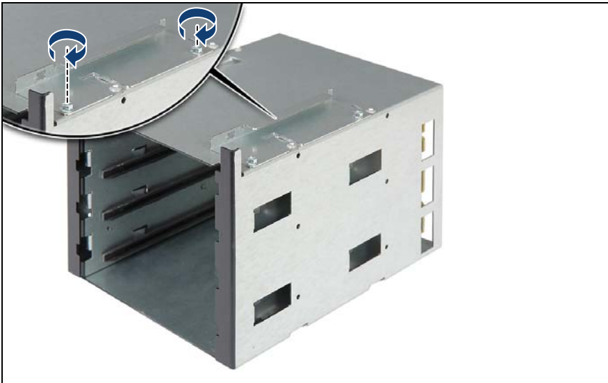
Figure 245: Reinstalling the slimline ODD mounting frame on the HDD expansion box
