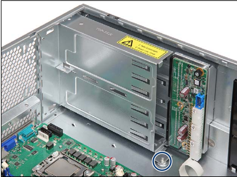
Figure 54: Securing the PSU cage (A)
