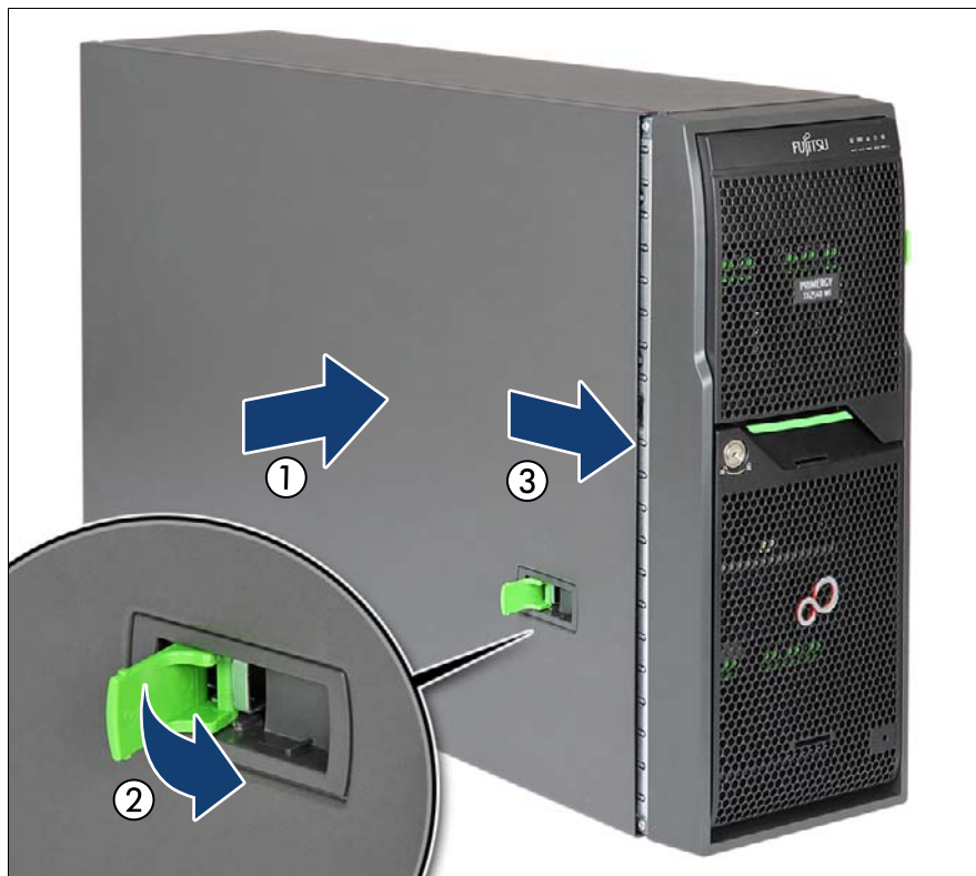
Figure 26: Installing the side cover (tower server)
