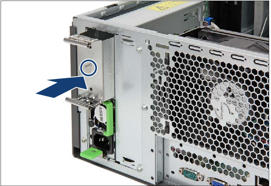
Figure 50: Installing a PSU dummy cover
