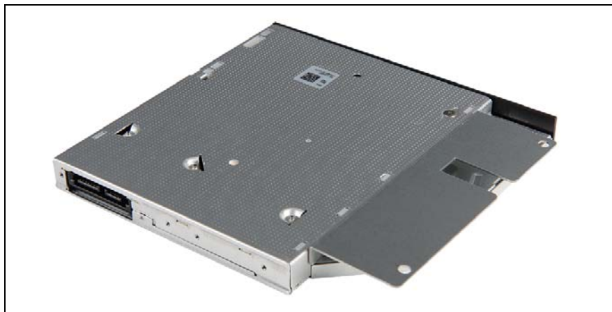
Figure 237: Installing the slimline ODD mounting bracket on the ODD (B)
