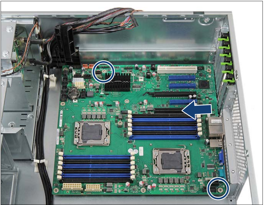
Figure 281: Removing the system board (B)
