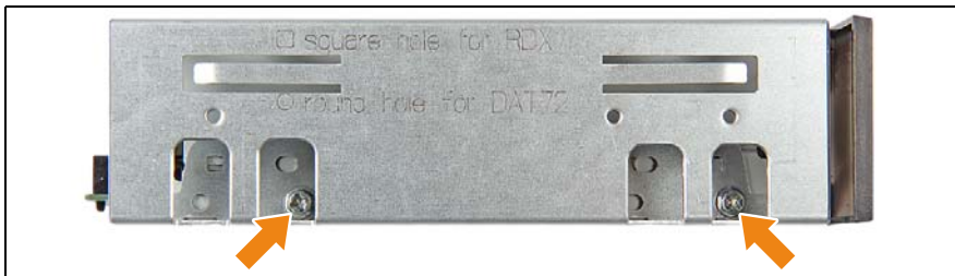
Figure 212: Securing mounting brackets to a DAT72 backup drive
