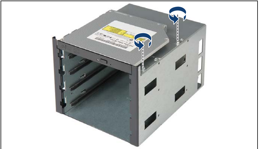
Figure 242: Removing the slimline ODD from the extension box (A)
