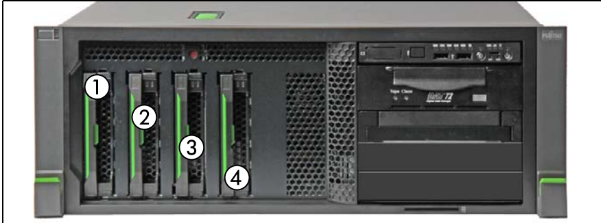
Figure 89: Mounting order with up to 4 3.5-inch HDDs (1 SAS backplane)
