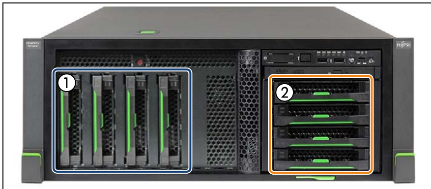
Figure 87: 3.5-inch SAS backplanes - maximum configuration, rack server
