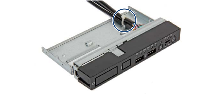
Figure 249: Front panel module - cable tie
