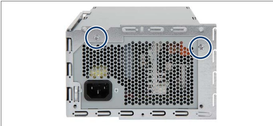
Figure 40: Removing the installation frame (A)
