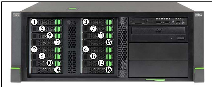
Figure 64: Mounting order with up to 16 2.5-inch HDDs (4 SAS backplanes)
