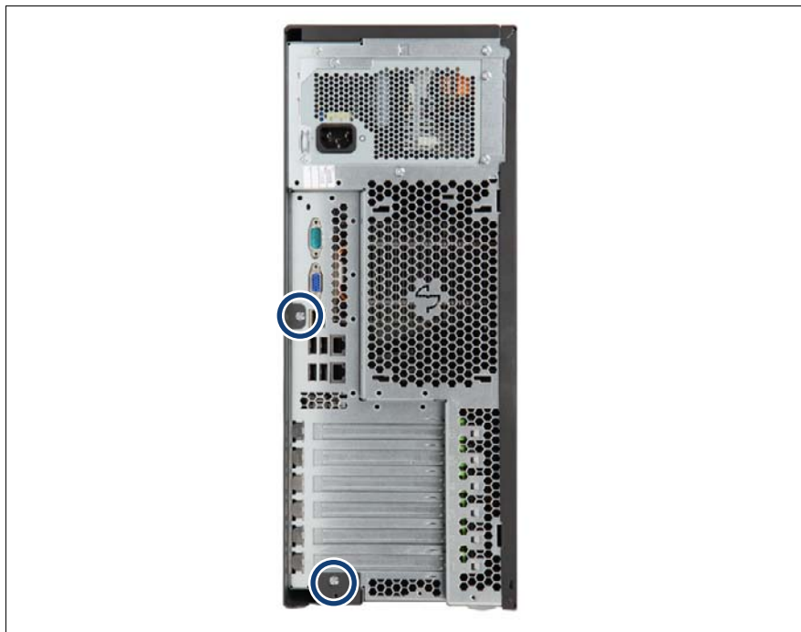
Figure 287: Removing the right side cover (A)
