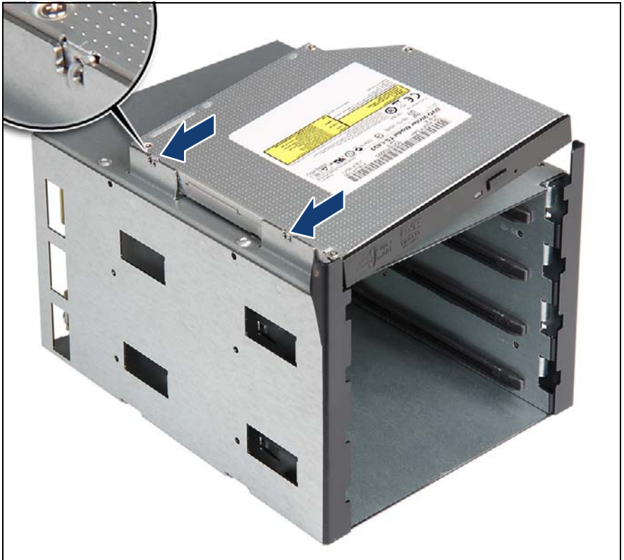
Figure 238: Installing the slimline ODD on the HDD extension box
