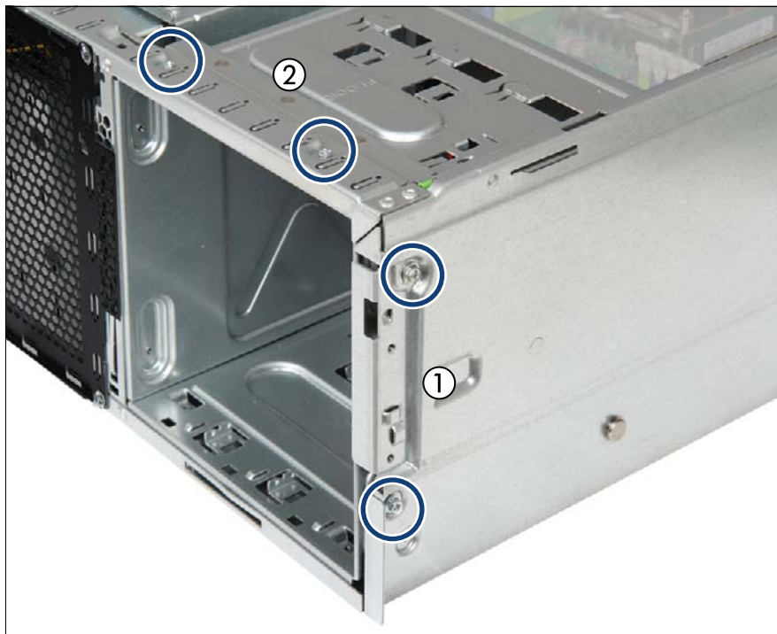
Figure 291: Detaching the accessible drive cage (B)
