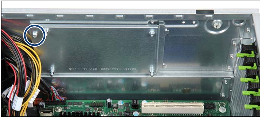
Figure 123: Installing the carrier (B)
