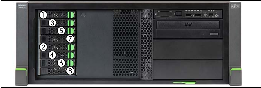
Figure 62: Mounting order with up to 8 2.5-inch HDDs (2 SAS backplanes)
