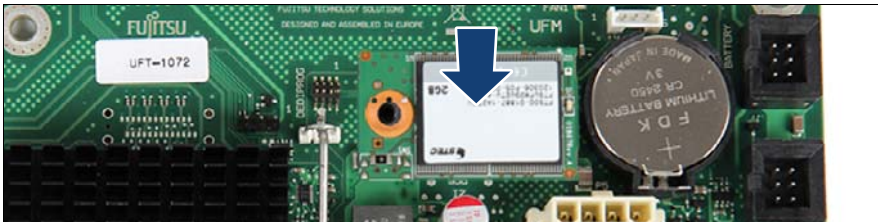
Figure 262: Installing the UFM (A)
