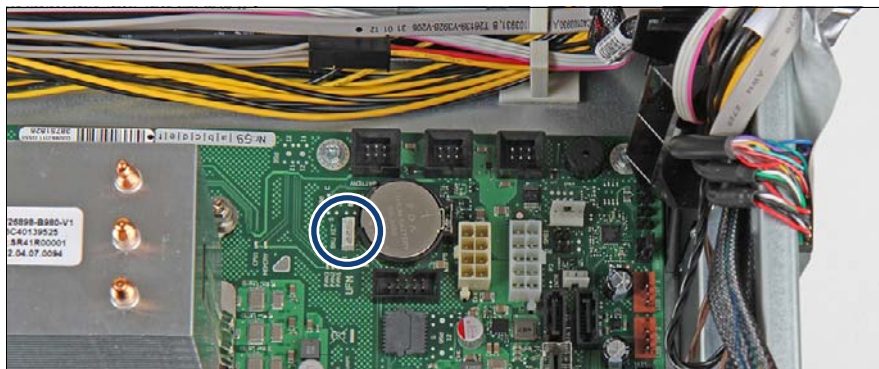
Figure 277: Onboard SAS enabling key mounting location
