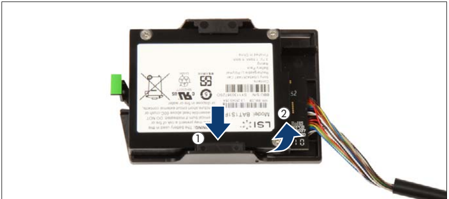
Figure 178: Removing the BBU from the holder
