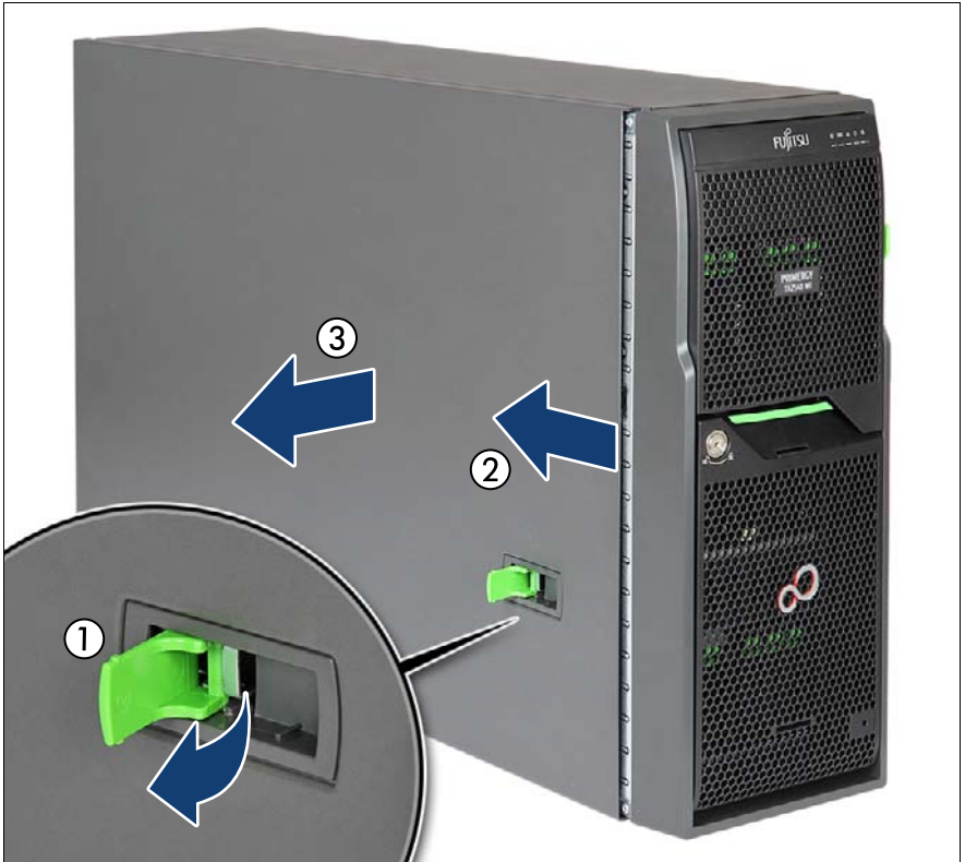
Figure 11: Removing the side cover (tower server)
