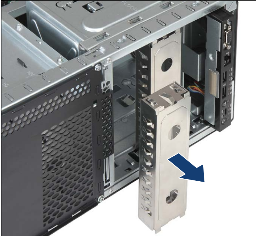
Figure 111: Removing an accessible drive filler cover
