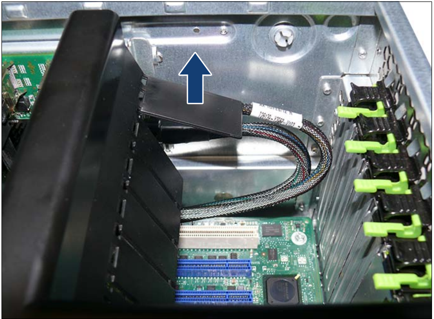
Figure 128: Preparing system air duct
