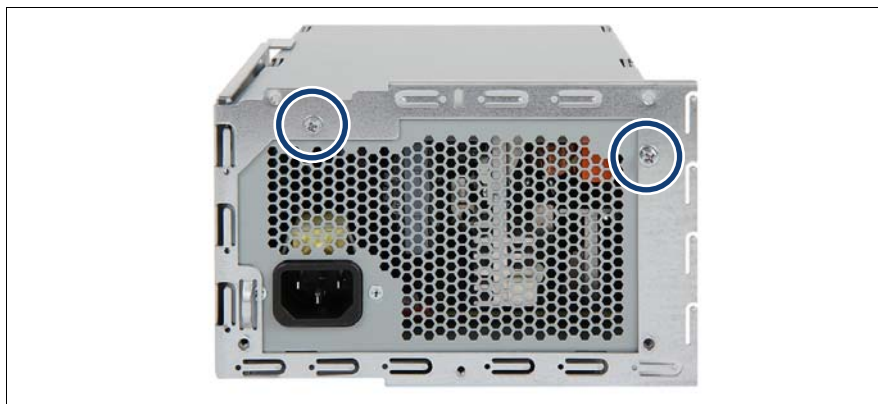
Figure 43: Installing the installation frame (B)
