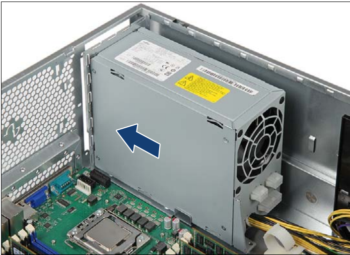
Figure 45: Installing PSU in the chassis (B)
