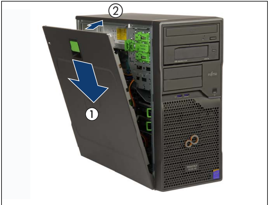
Figure 14: Installing the side cover
