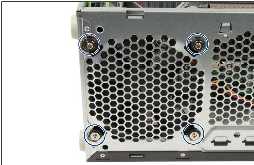
Figure 53: Fastening the screws of the system fan 2
