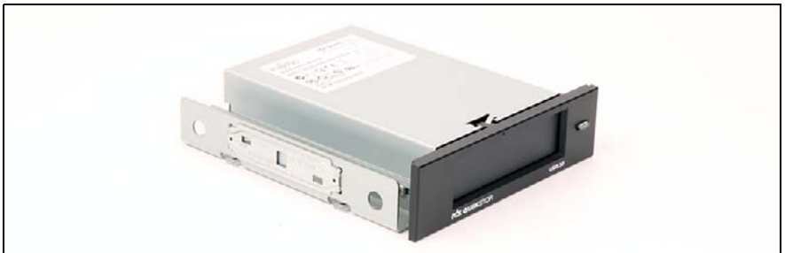
Figure 119: Attaching the fixation plate to the backup drive (B)
