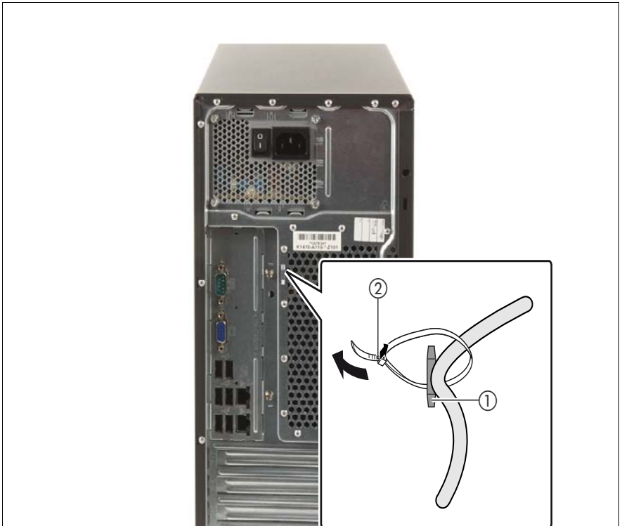
Figure 3: Removing the power cord from the PSU cable tie
