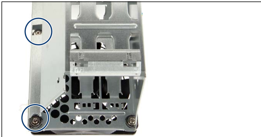
Figure 62: Installing the system fan 1
