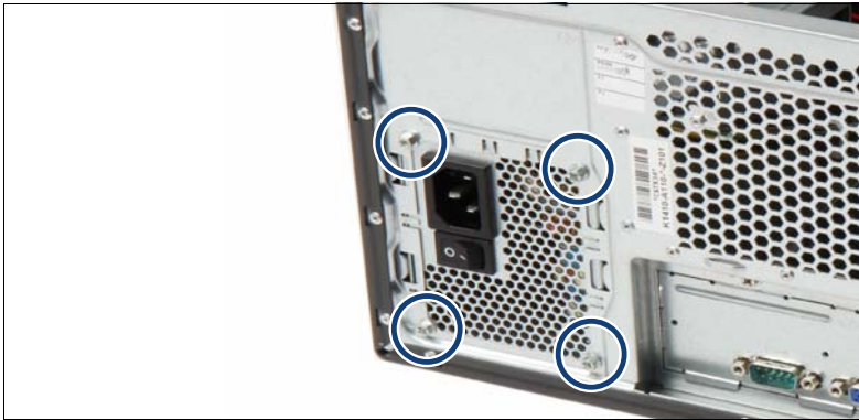
Figure 30: Securing the PSU
