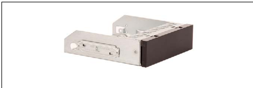
Figure 124: Attaching the fixation plate to the dummy drive for bay 2
