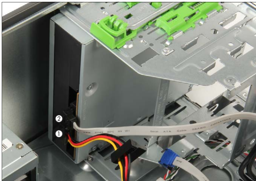
Figure 11: Connecting cables to the optical disk drive
