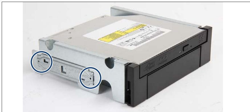
Figure 114: Attaching the fixation plate to the slide-in unit
