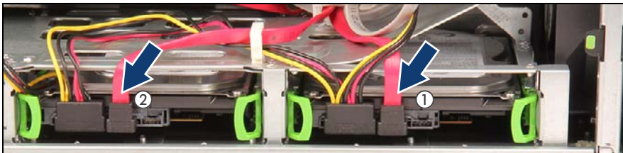
Figure 39: Connecting SATA cables to HDD1 and HDD2
