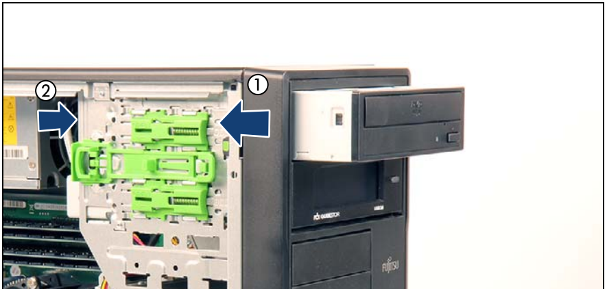
Figure 122: Removing the slide-in unit
