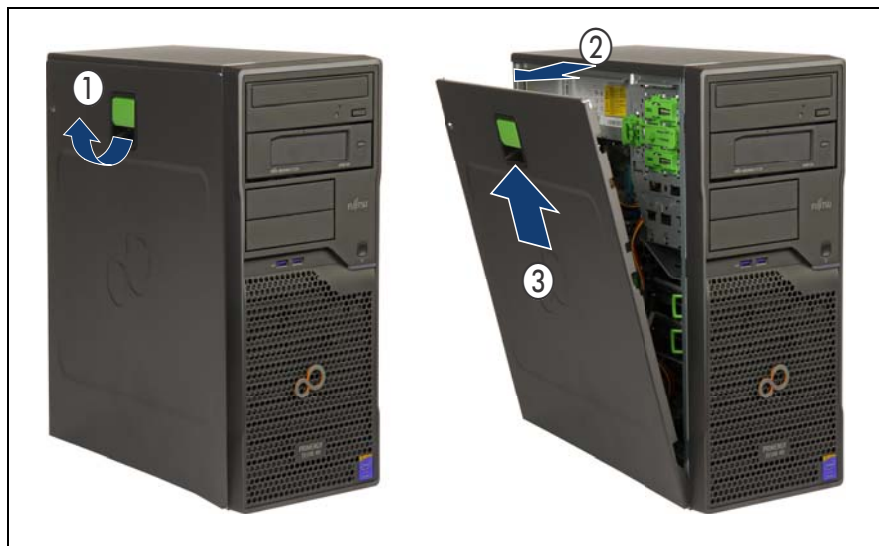
Figure 4: Removing the cover
