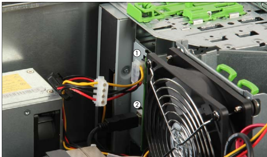
Figure 13: Connecting cables to the backup drive
