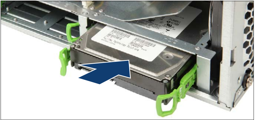
Figure 36: Inserting the 3.5-inch HDD
