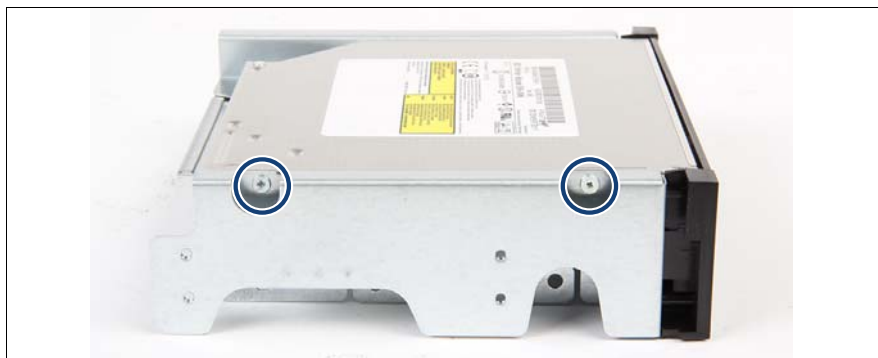
Figure 113: Mounting the slimline ODD in the slide-in unit (B)
