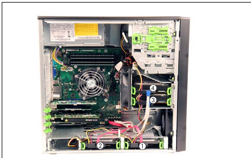
Figure 32: 3.5-inch HDD mounting order
