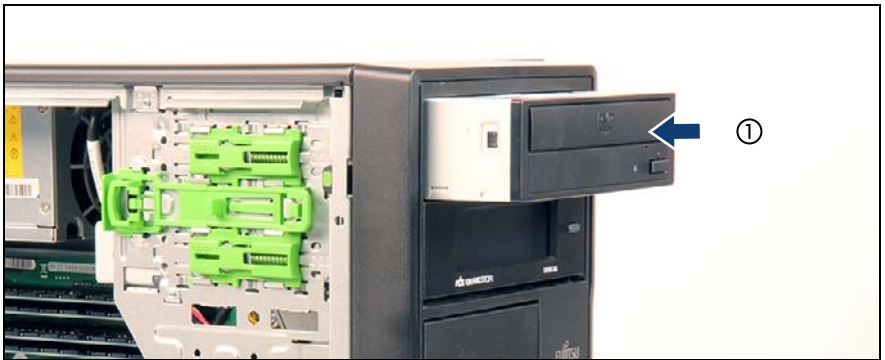
Figure 115: Installing the slide-in unit
