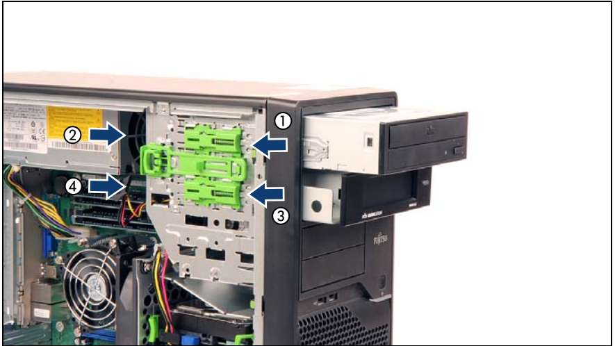
Figure 7: Removing the optical disk drive and the backup drive
