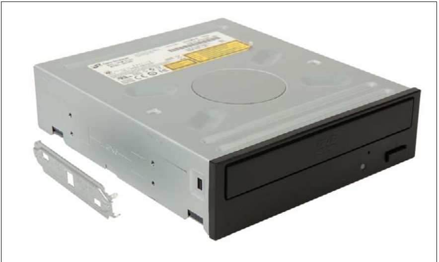
Figure 108: Attaching the fixation plate to the optical disk drive (A)
