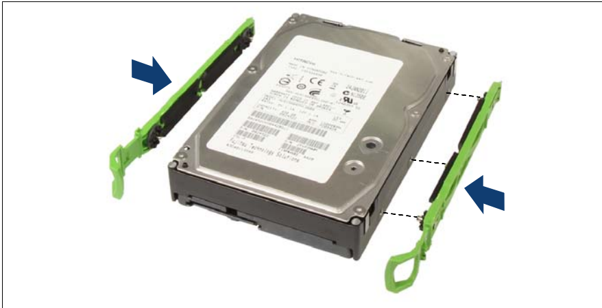
Figure 34: Aligning the Easyclick rails
