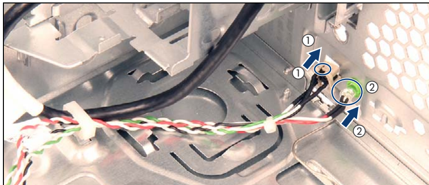
Figure 137: Installing the On/Off button
