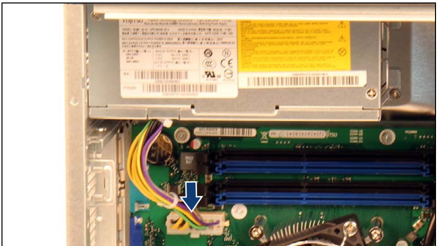
Figure 31: Connecting power cable
