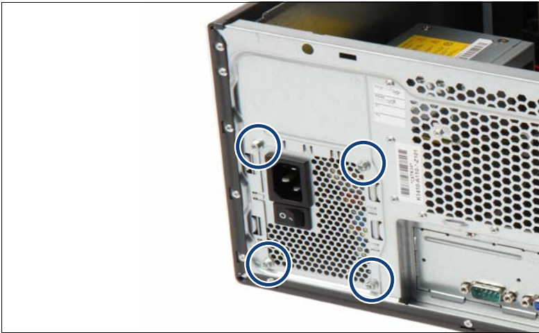
Figure 26: Detaching the PSU
