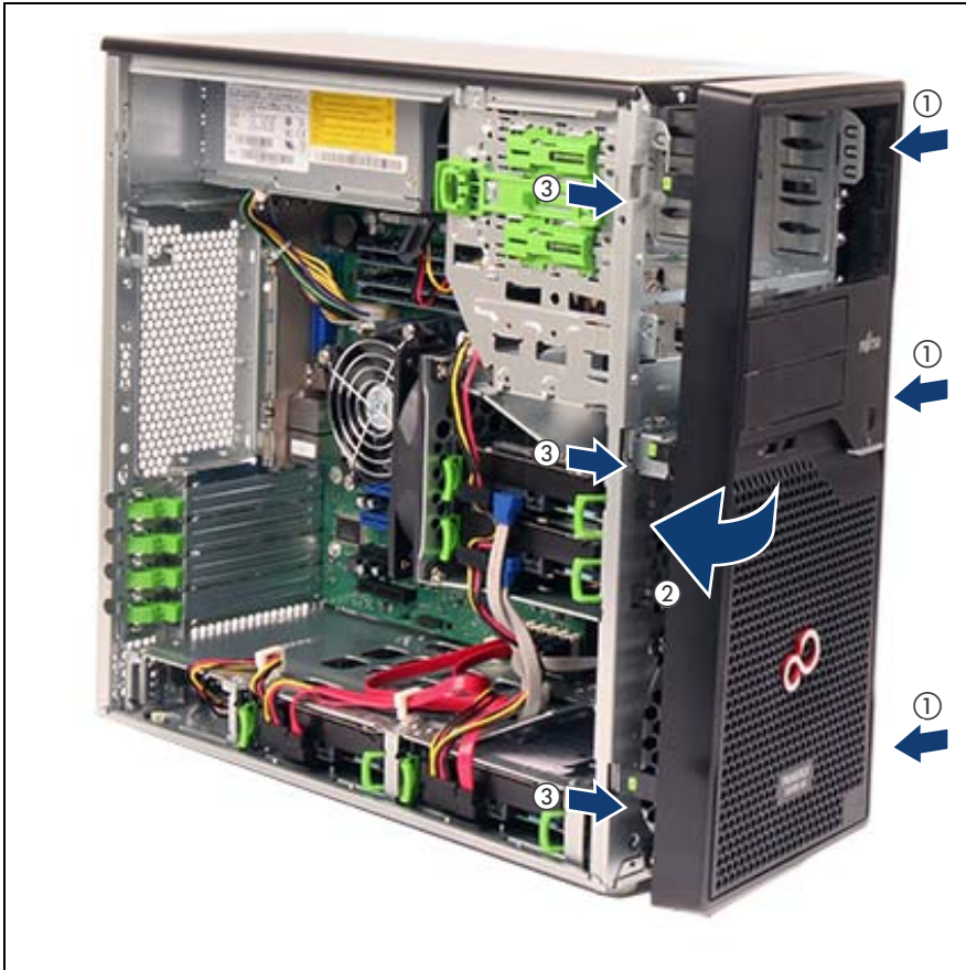
Figure 9: Installing the front cover
