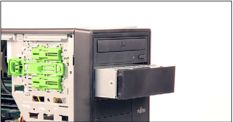
Figure 125: Installing the dummy drive in bay 2
