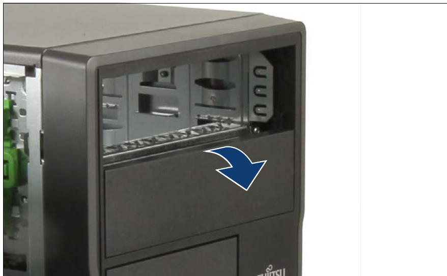
Figure 104: Removing the dummy cover of bay 2
