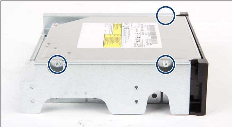
Figure 129: Removing the slimline ODD from the slide-in unit (A)
