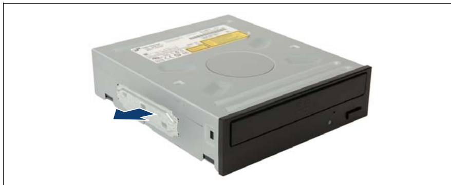
Figure 126: Removing the fixation plate
