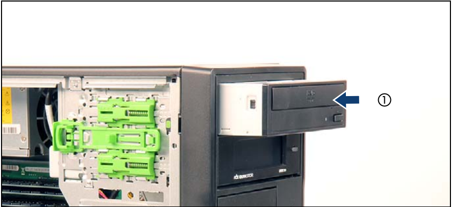
Figure 10: Installing the optical disk drive
