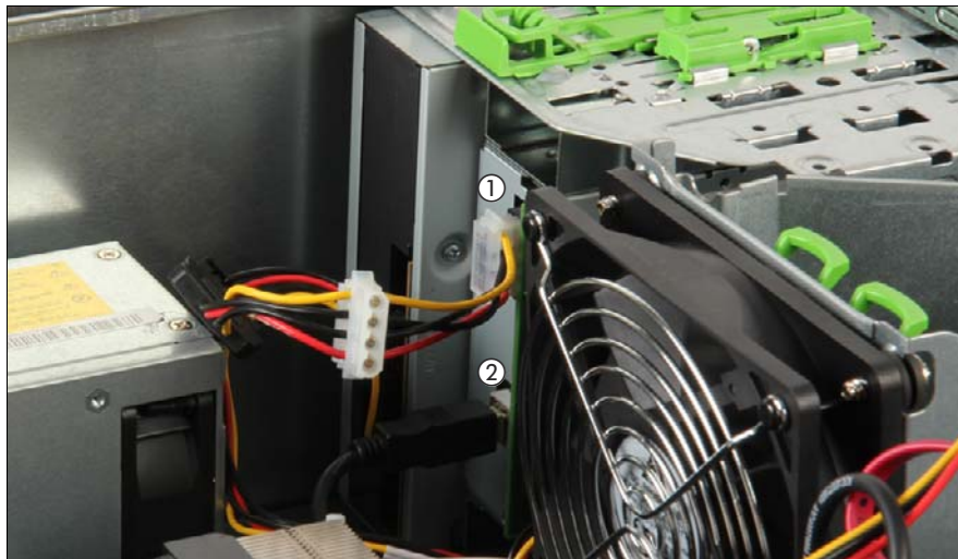
Figure 6: Disconnecting cables from the backup drive
