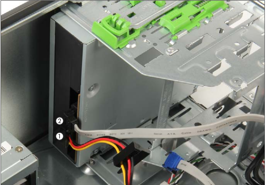
Figure 5: Disconnecting cables from the optical disk drive
