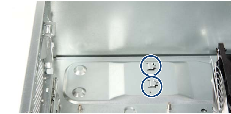
Figure 28: Hooks for fastening the PSU
