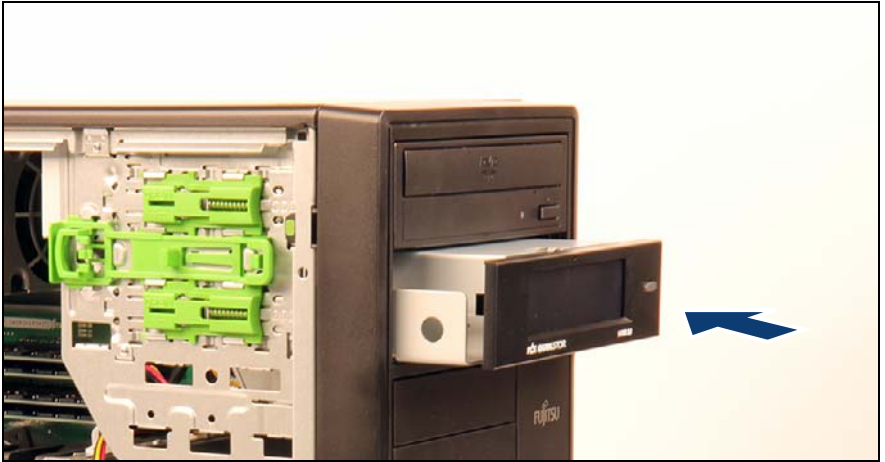
Figure 12: Installing the backup drive
