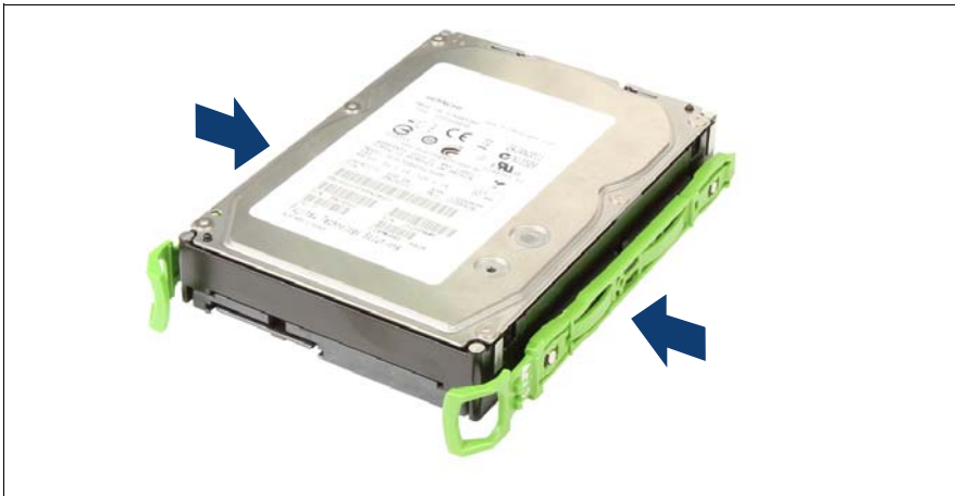
Figure 35: Attaching the Easyclick rails
