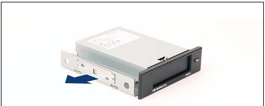
Figure 131: Removing the fixation plate
