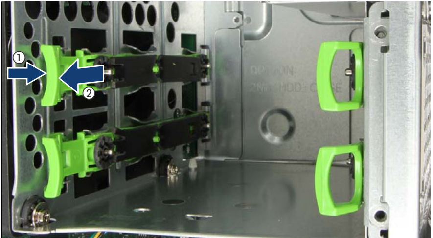
Figure 33: Removing the Easyclick rails out of the bay
