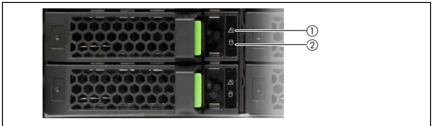
Figure 10: Indicators on the 3.5 inch HDD modules
