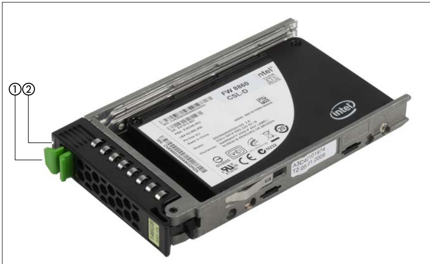
Figure 11: Indicators on the SSD modules
