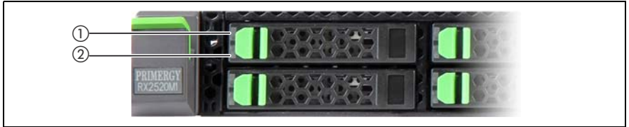
Figure 9: Indicators on the 2.5 inch HDD modules
