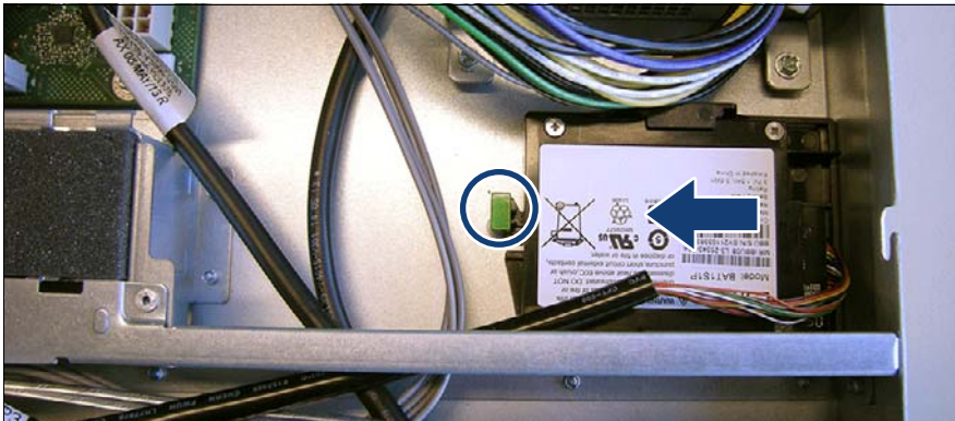
Figure 132: Removing the BBU with the holder
