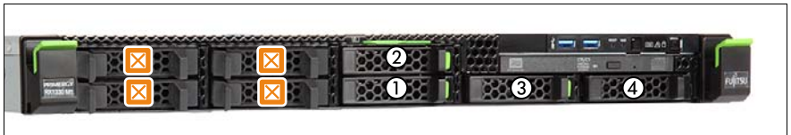
Figure 48: Mounting order with up to four 2.5-inch HDDs/SSDs
