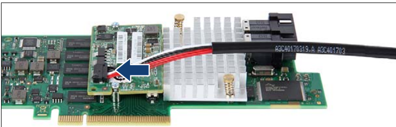
Figure 115: Connecting the FBU adapter cable
