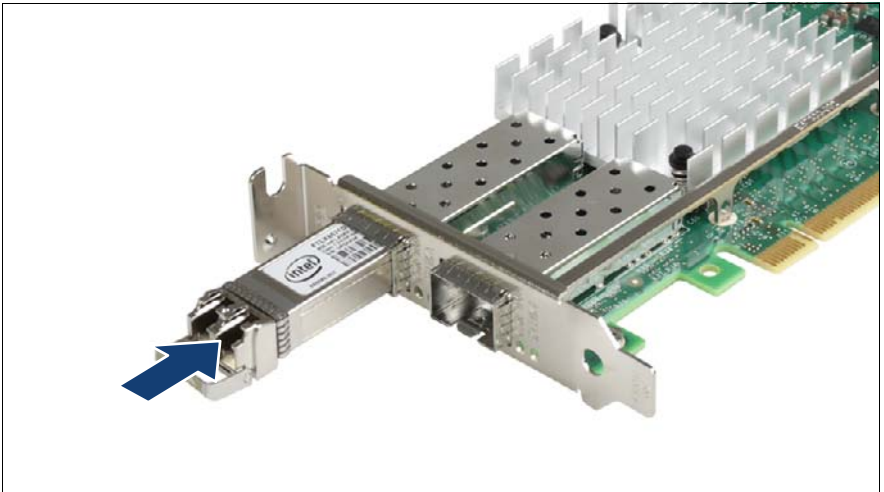
Figure 98: Inserting the SFP+ transceiver module
