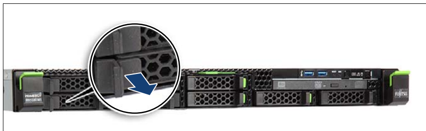
Figure 54: Removing dummy lock
