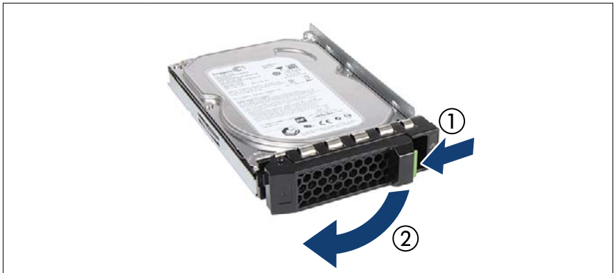
Figure 79: Opening the 3.5-inch HDD module locking lever
