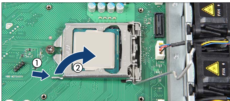
Figure 144: Opening the holder
