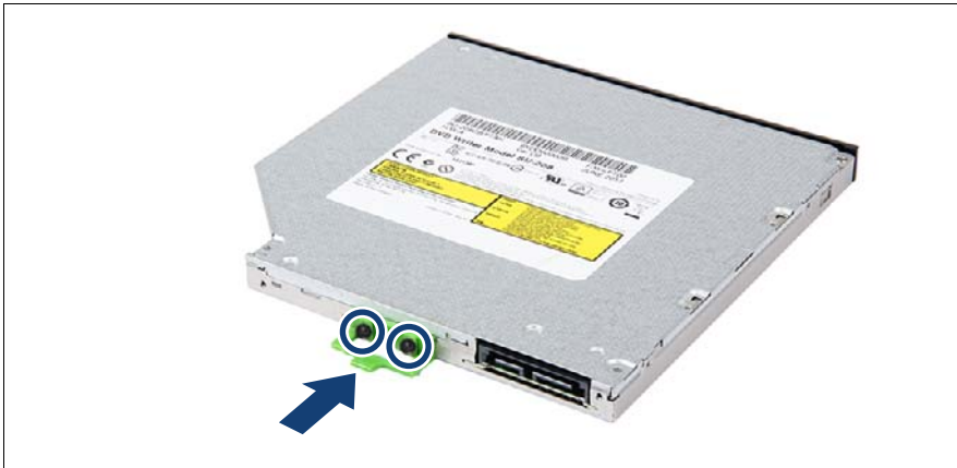
Figure 158: Installing the ODD latch on the ODD
