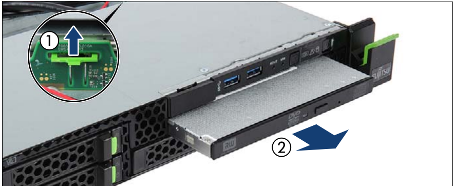
Figure 162: Removing the ODD
