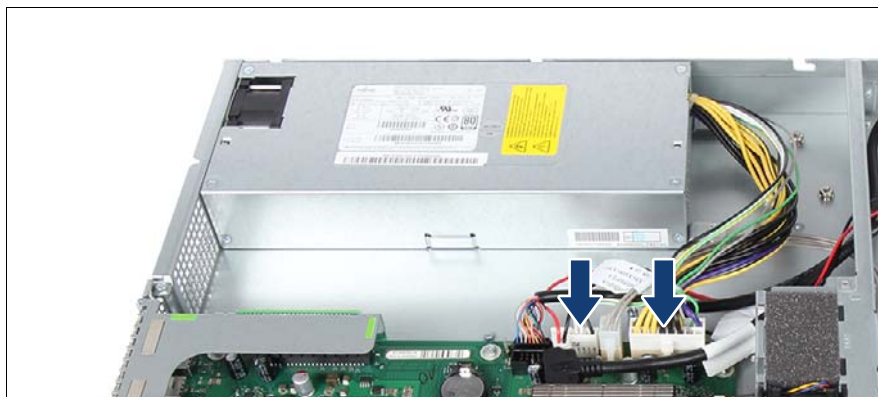
Figure 25: Connecting the power cables
