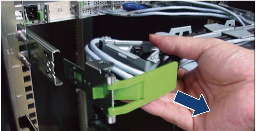
Figure 32: Removing the CMA stopper
