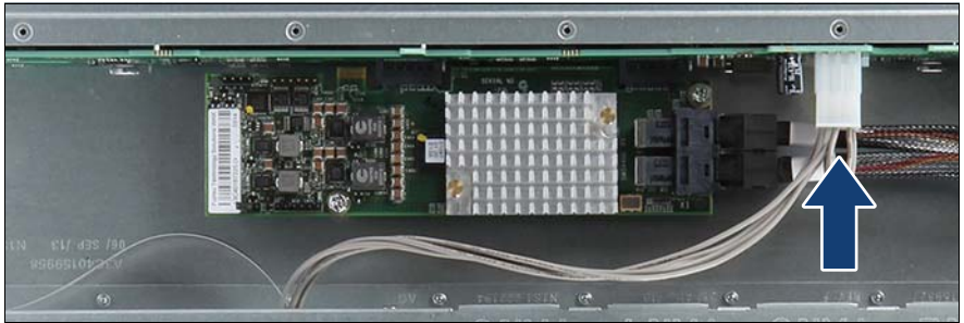
Figure 74: Connecting power cable to the HDD backplane
