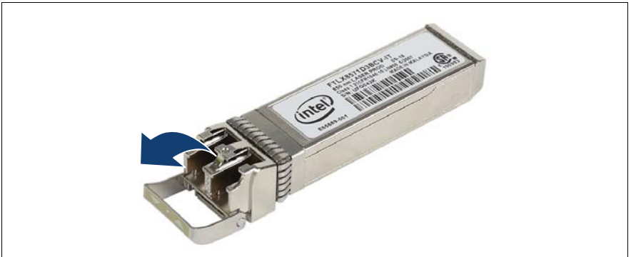
Figure 97: Unlatching the locking bail
