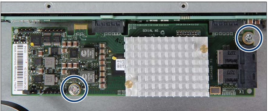
Figure 67: Removing the SAS expander board (A)
