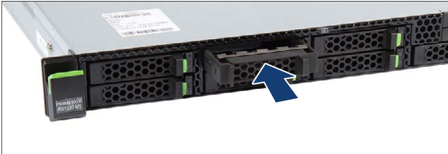
Figure 58: Installing a 2.5-inch dummy module
