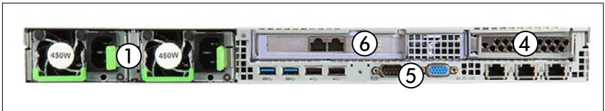
Figure 221: Rear side (redundant power supply and full height riser module)
