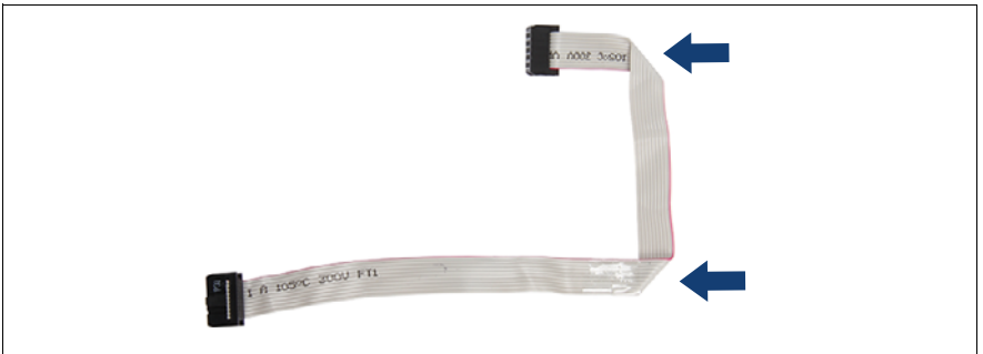
Figure 43: Folding the flat cable
