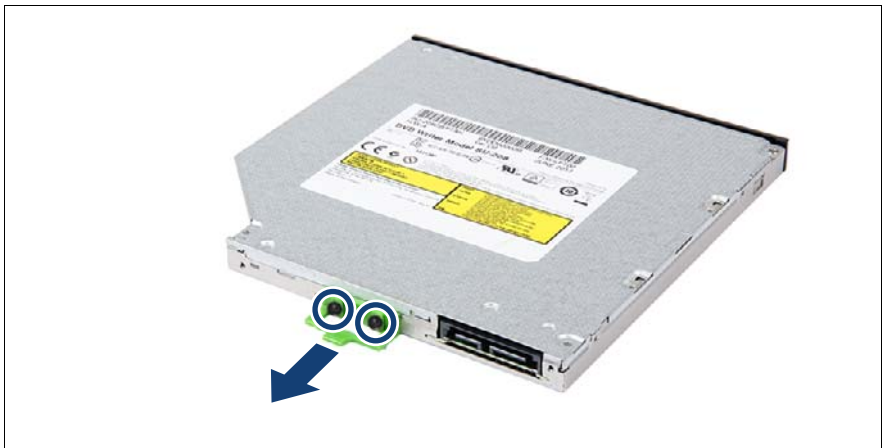
Figure 163: Removing the ODD latch from the ODD
