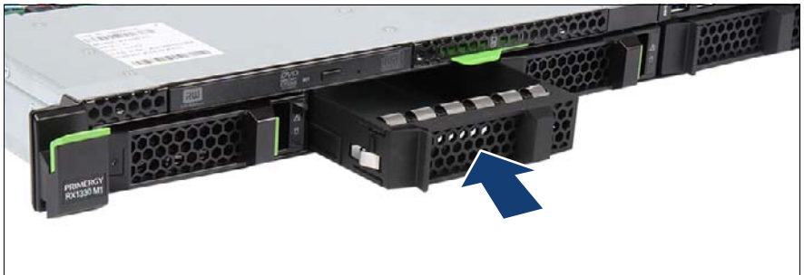
Figure 81: Installing the 3.5-inch dummy module
