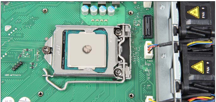
Figure 149: Applying the thermal paste
