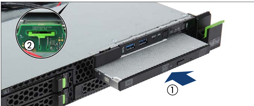
Figure 159: Installing the ODD
