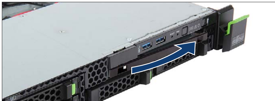
Figure 164: Installing the dummy cover
