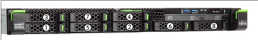
Figure 50: Mounting order with up to eight HDD/SSD bays
