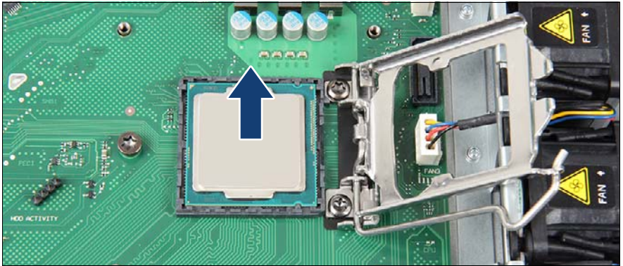
Figure 145: Removing the processor
