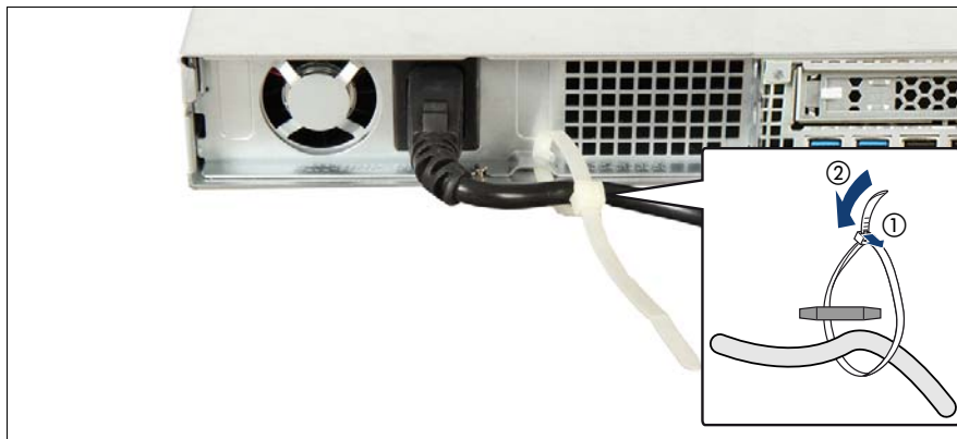
Figure 2: Unlocking the cable tie of a standard power supply unit
