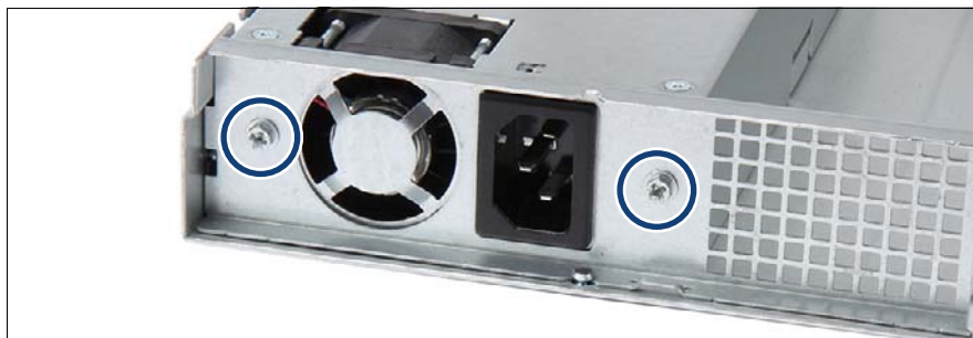
Figure 22: Removing the screws
