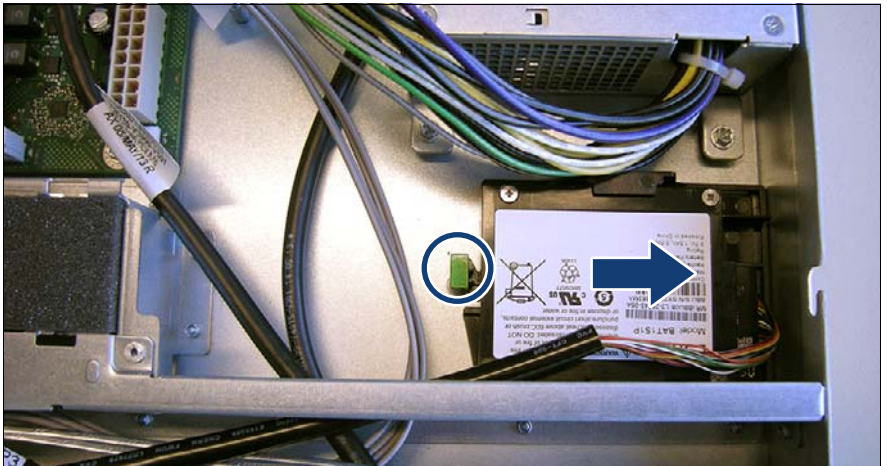
Figure 125: Installing the BBU with the holder
