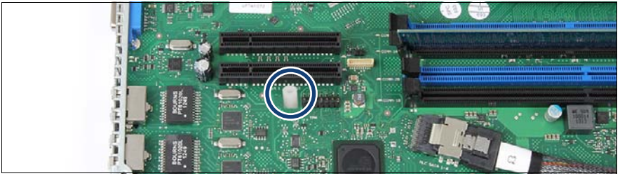
Figure 195: Inserting the TPM spacer on the system board
