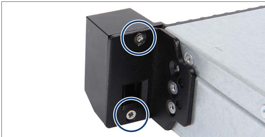
Figure 178: Removing the front panel on QRL (A)
