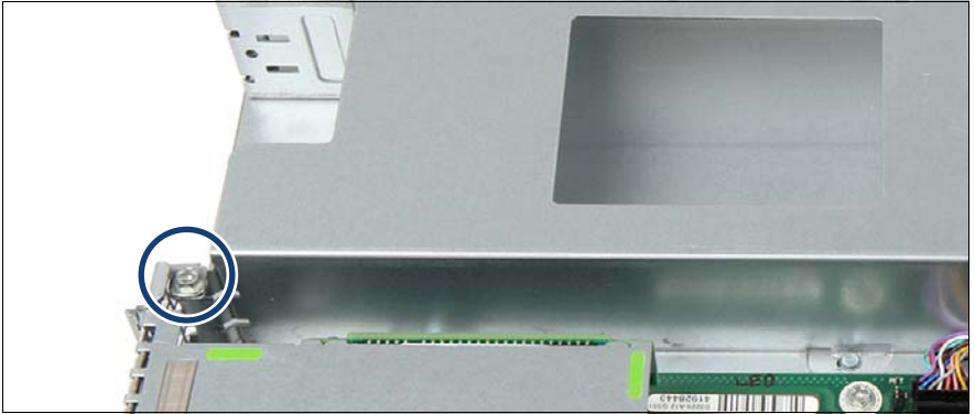
Figure 42: Fastening the PSU cage
