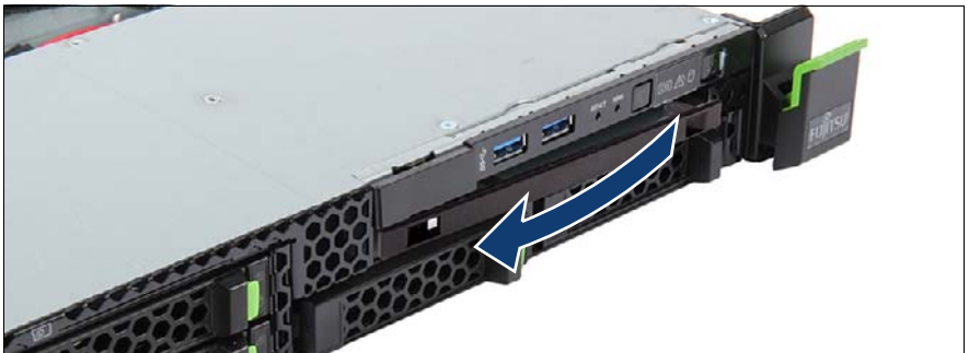
Figure 157: Removing the dummy cover
