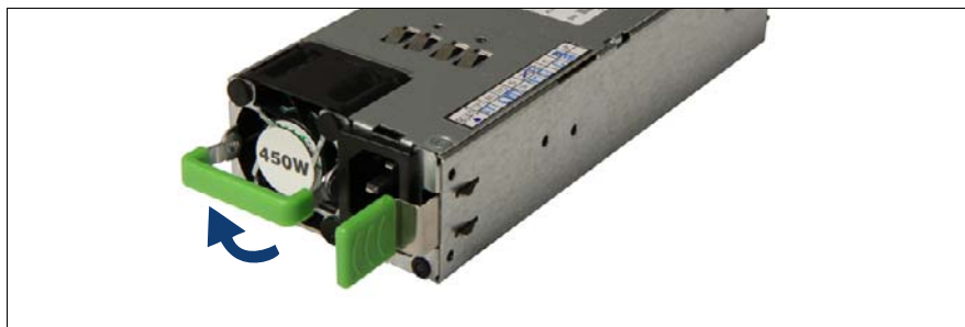
Figure 28: Folding up the handle
