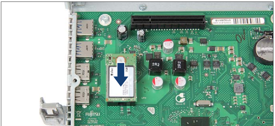
Figure 186: Installing the UFM
