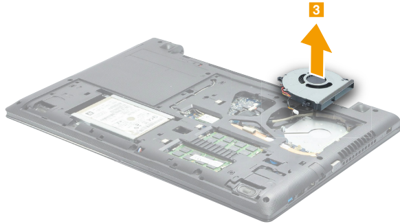
Figure 7. Removal steps of fan assembly (continued)
