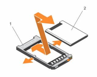
Figure 58. Removing and installing a 1.8 hard drive into a hard drive carrier
