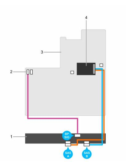
Figure 65. Cabling diagram—3.5 inch (x8) SAS/SATA backplane—(option 1)
