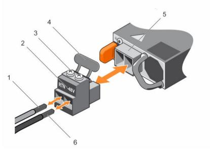
Figure 48. Assembling the DC input power wires
