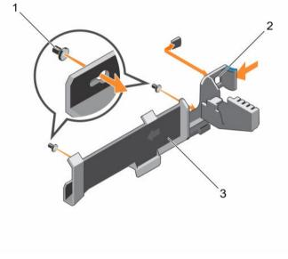
Figure 27. Removing and installing the cable retention bracket
