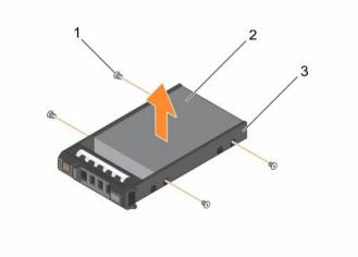
Figure 56. Removing and installing a hard drive into a hard drive carrier
