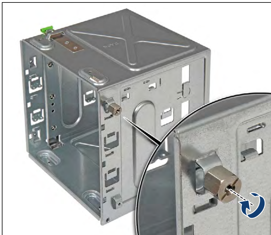
Figure 563: Converting the accessible drive cage (B)
