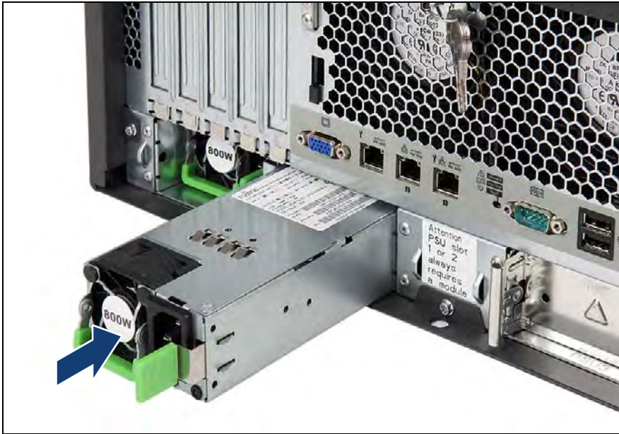
Figure 78: Installing a PSU module
