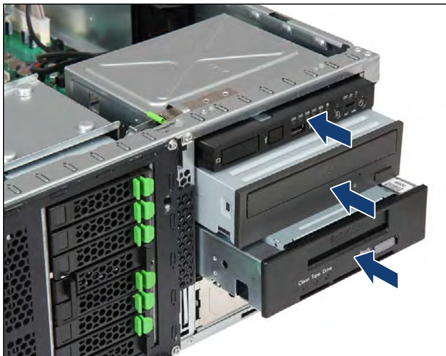
Figure 571: Reinstalling accessible drives
