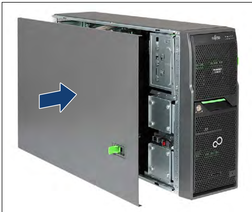
Figure 56: Mounting the side cover (tower server) (A)
