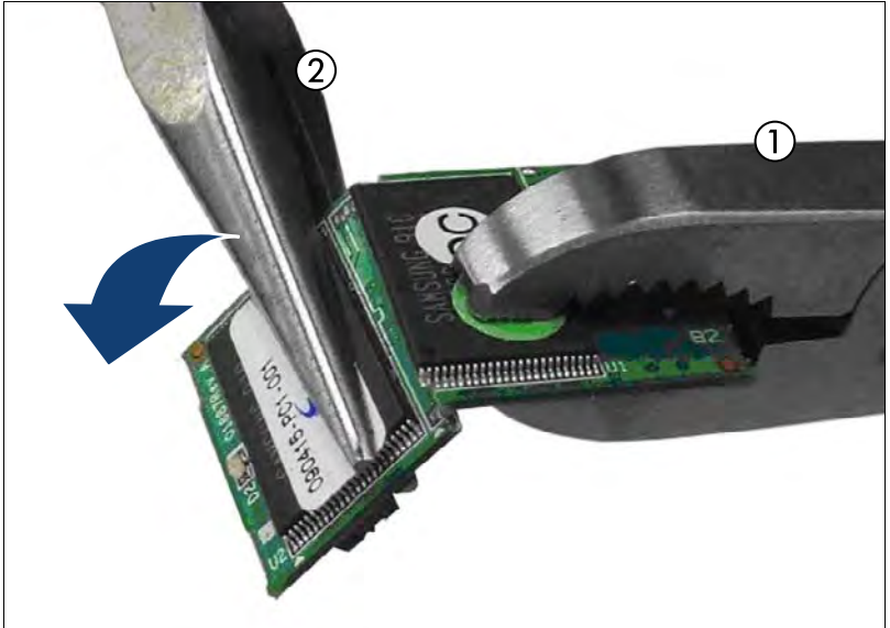
Figure 516: Destroying the defective UFM board
