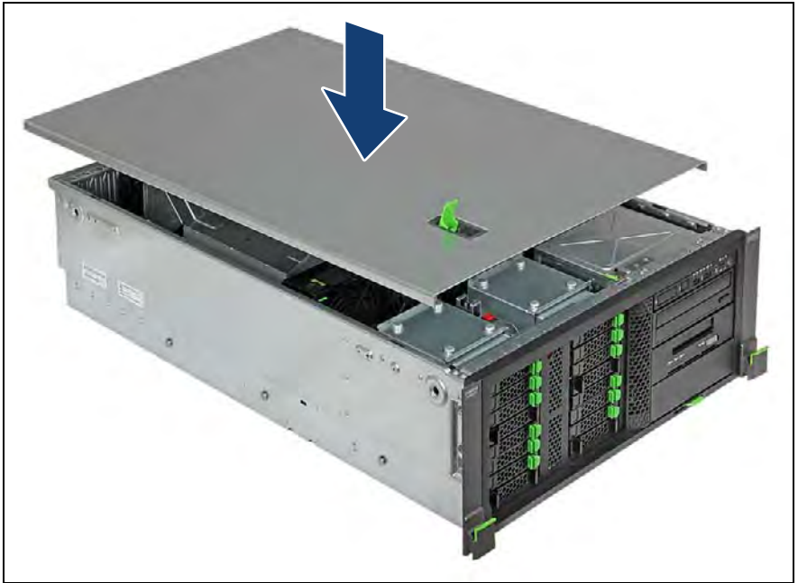
Figure 49: Mounting the top cover (rack server) (A)
