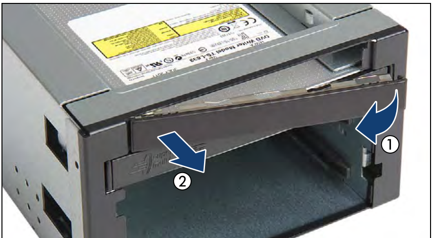
Figure 444: Removing the LSD dummy cover plate (B)
