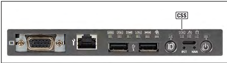
Figure 5: CSS error indicator in front panel
