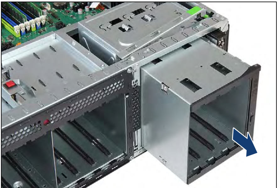
Figure 203: Removing the HDD extension box
