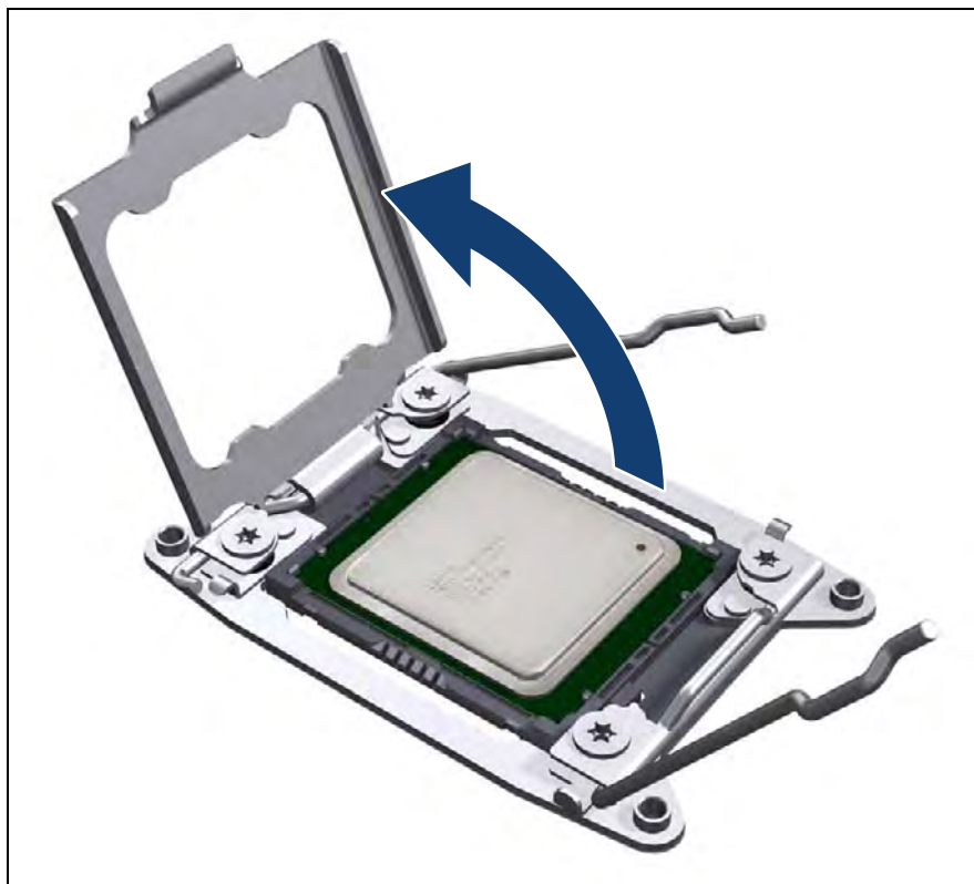
Figure 378: Opening the load plate (B)
