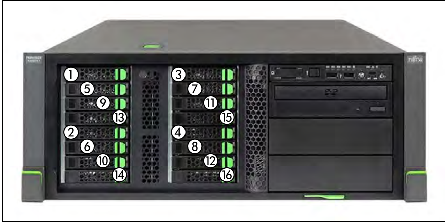
Figure 99: Mounting order: up to 16x 2.5-inch SAS 2.0 HDDs / SSDs
