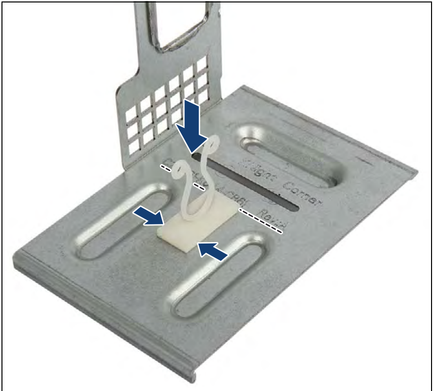
Figure 273: Preparing the GPGPU / coprocessor card mounting bracket
