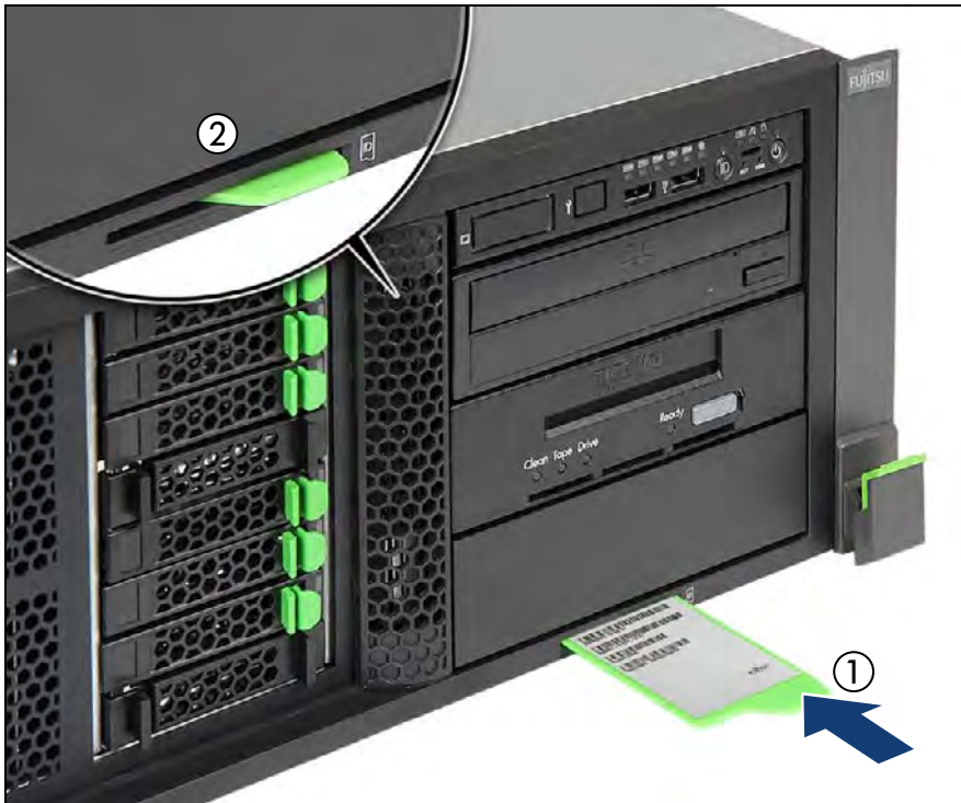
Figure 48: Installing the ID card (rack server)
