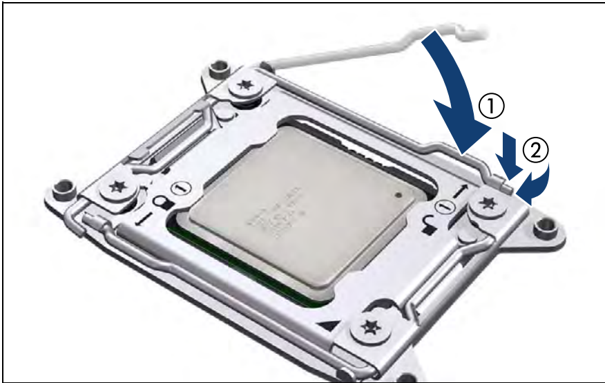
Figure 393: Closing socket release lever 1
