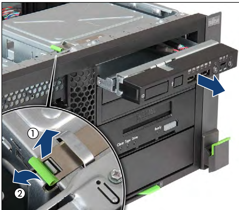
Figure 471: Removing the front panel module (rack systems)
