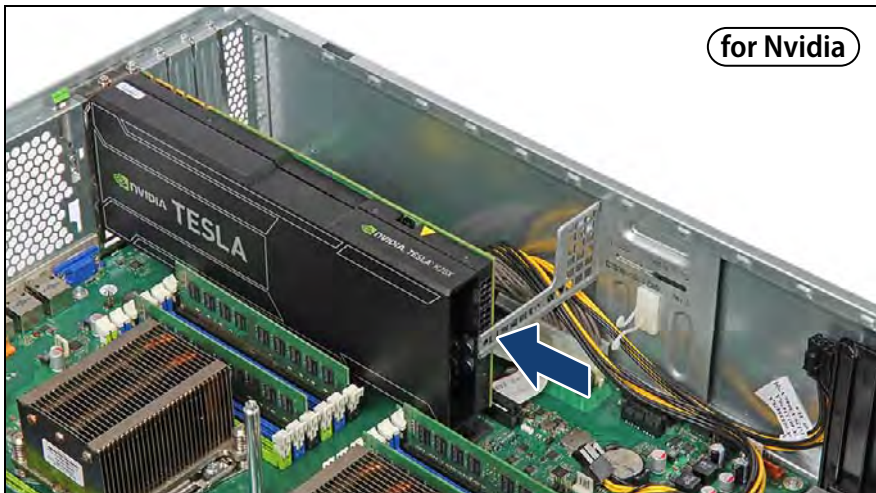
Figure 286: Securing the GPGPU card (Nvidia) (B)
