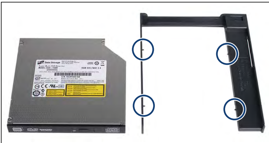
Figure 439: Mounting the slimline ODD in the installation frame (A)
