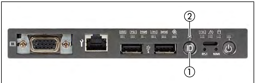
Figure 2: ID button and ID indicator on front panel
