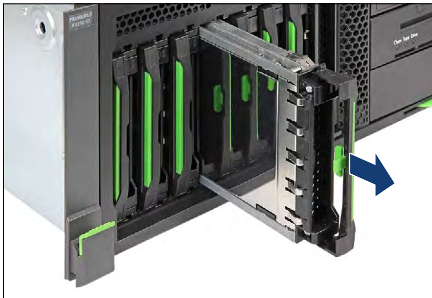
Figure 166: Removing a 3.5-inch HDD module
