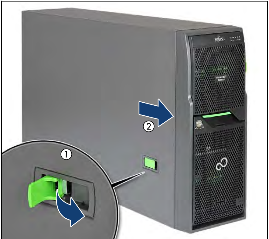
Figure 57: Mounting the side cover (tower server) (B)
