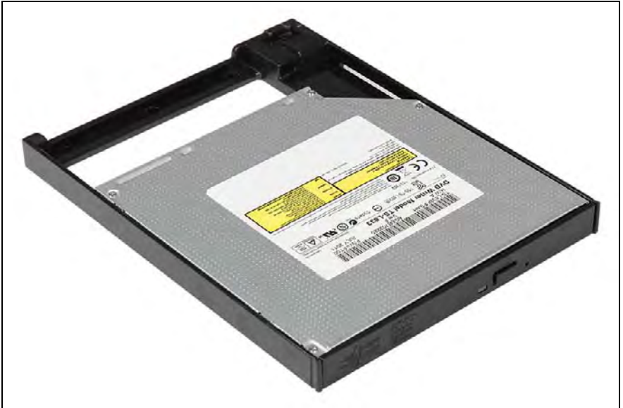
Figure 440: Mounting the slimline ODD in the installation frame (B)
