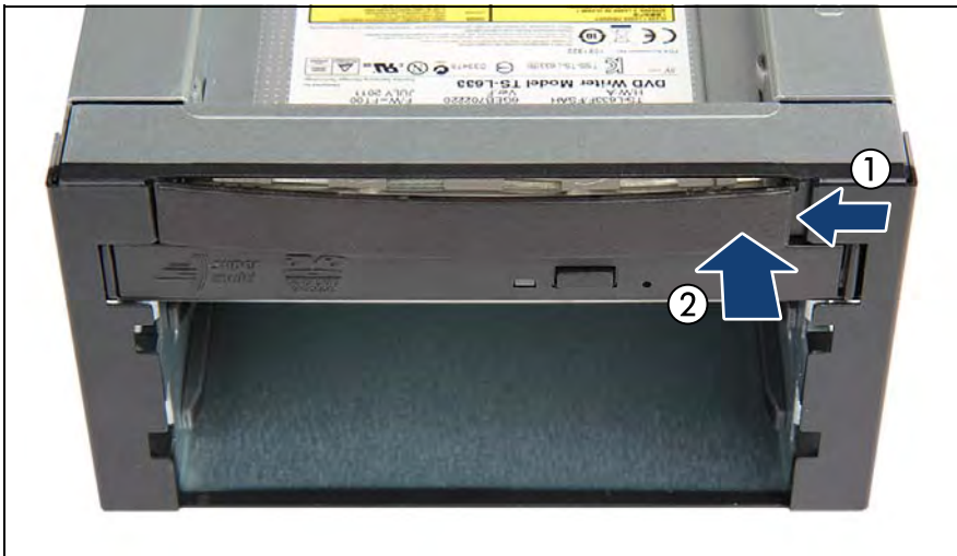
Figure 453: Mounting the slimline ODD dummy insert in the installation frame
