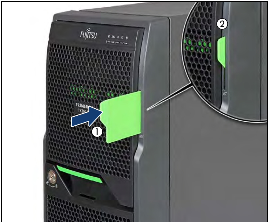
Figure 55: Installing the ID card (rack server)
