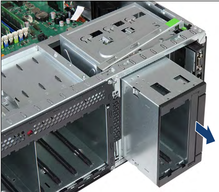
Figure 200: Removing the HDD extension box
