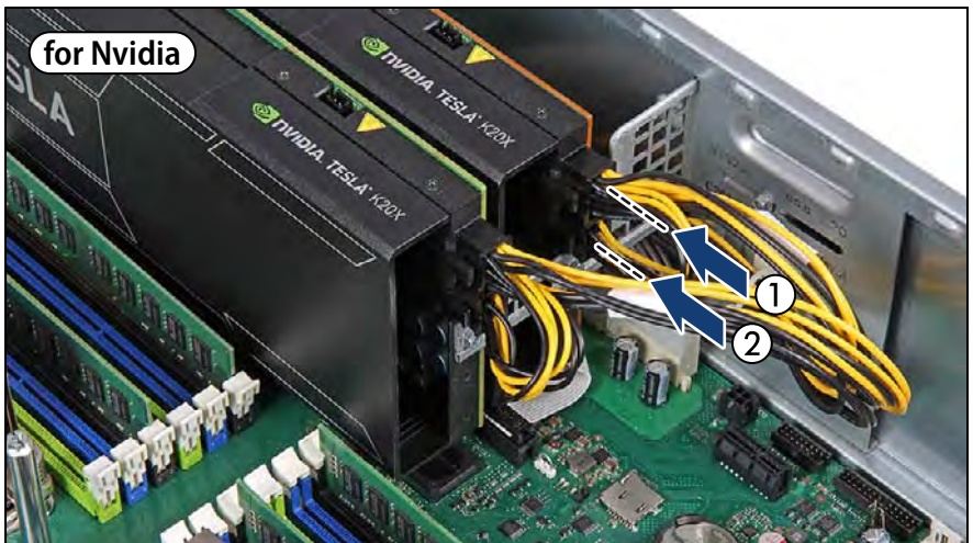
Figure 297: Cabling the secondary GPGPU card (Nvidia)
