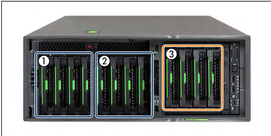
Figure 147: 3.5-inch SAS backplanes - Tower version with 4x 3.5-inch HDD extension box
