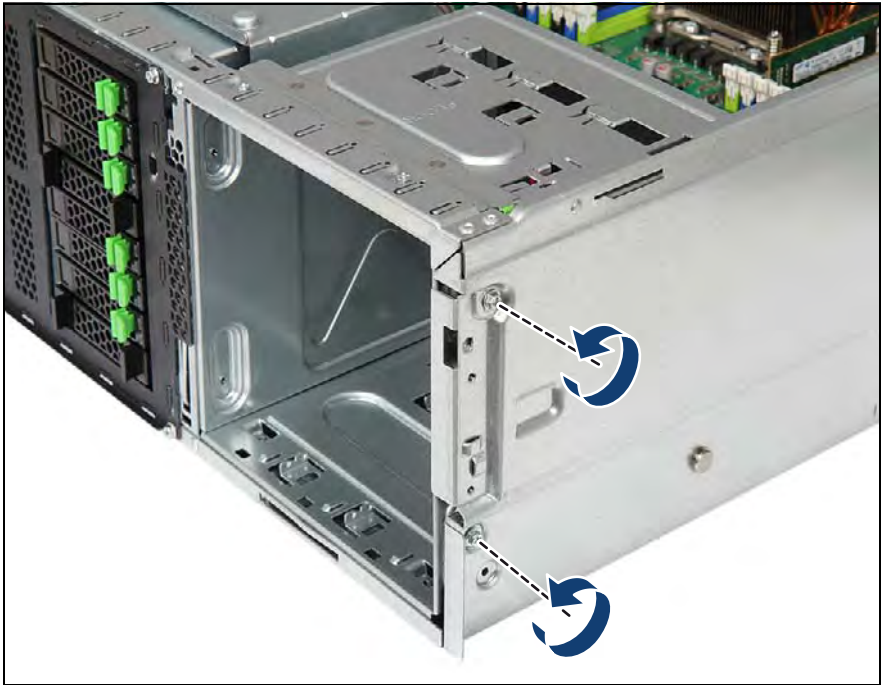
Figure 558: Detaching the accessible drive cage (B)
