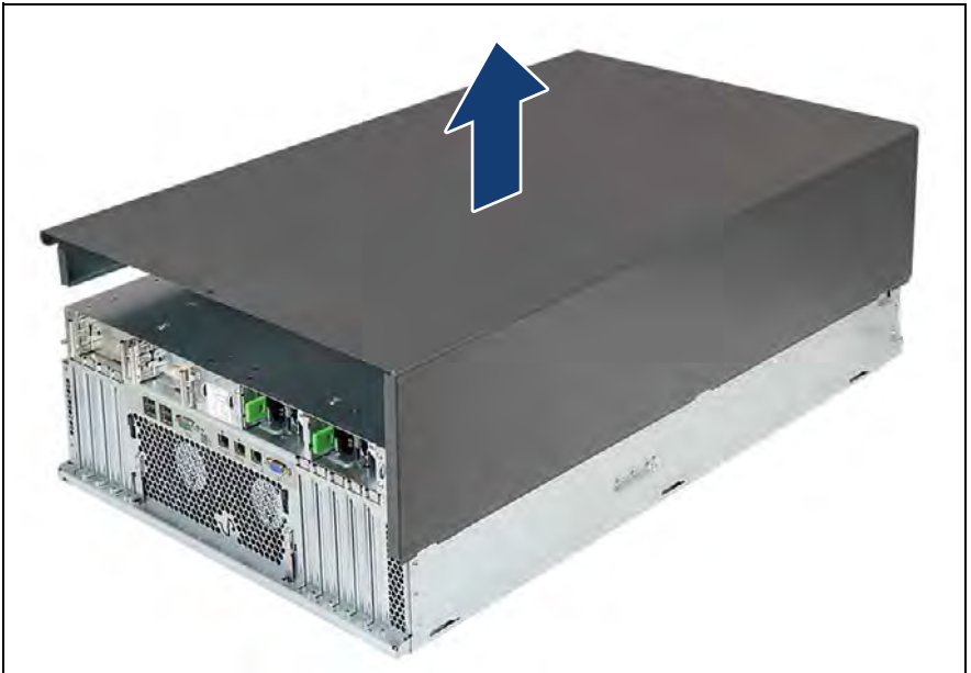
Figure 556: Removing the right side cover (D)
