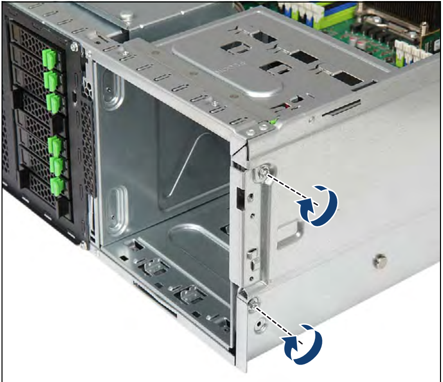
Figure 568: Securing the accessible drive cage (B)
