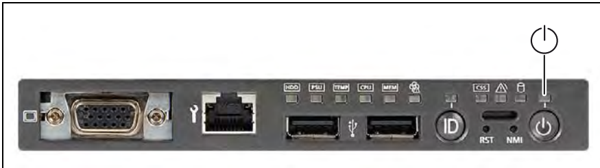
Figure 6: On / Off button on the front panel
