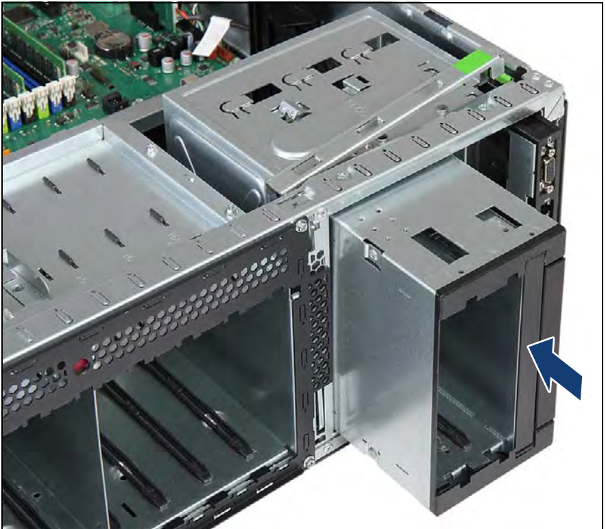
Figure 199: Inserting the 2x 3.5-inch HDD extension box
