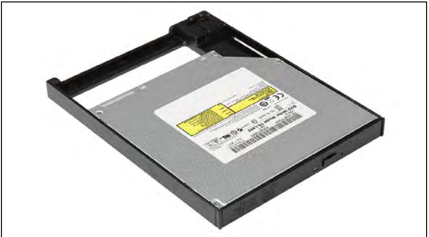
Figure 421: Mounting the slimline ODD in the installation frame (B)
