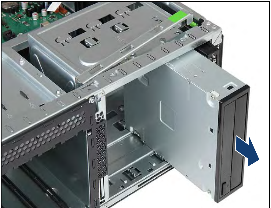
Figure 418: Removing the accessible drive
