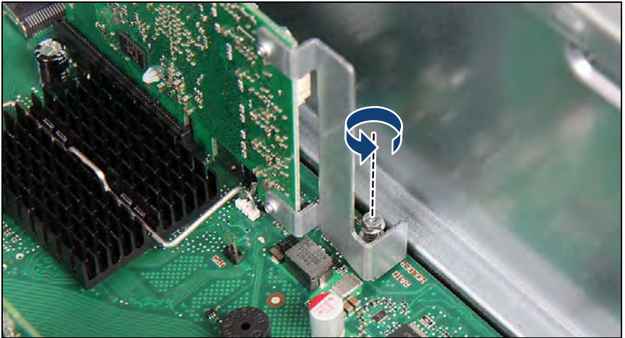
Figure 325: Removing the SAS RAID controller (A)
