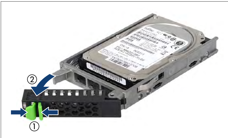
Figure 109: Opening the 2.5-inch HDD / SSD module locking lever
