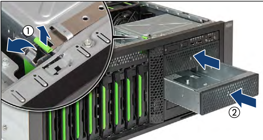
Figure 319: Installing perforated drive cover modules (A)
