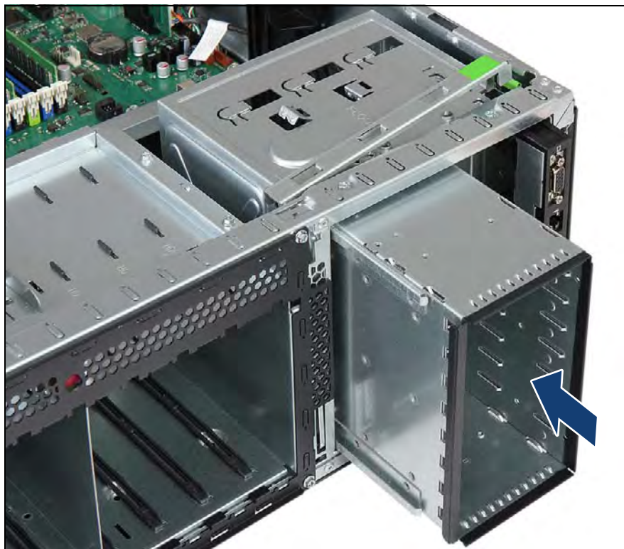
Figure 205: Inserting the HDD extension box
