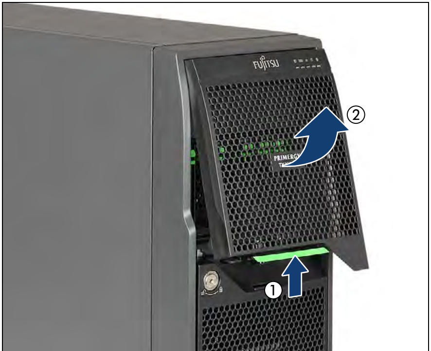
Figure 24: Removing the accessible drive bay cover
