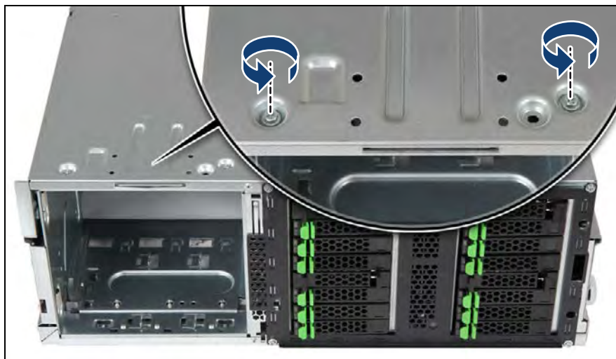
Figure 557: Detaching the accessible drive cage (A)
