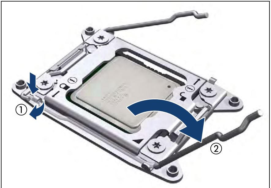
Figure 386: Opening socket release lever 2
