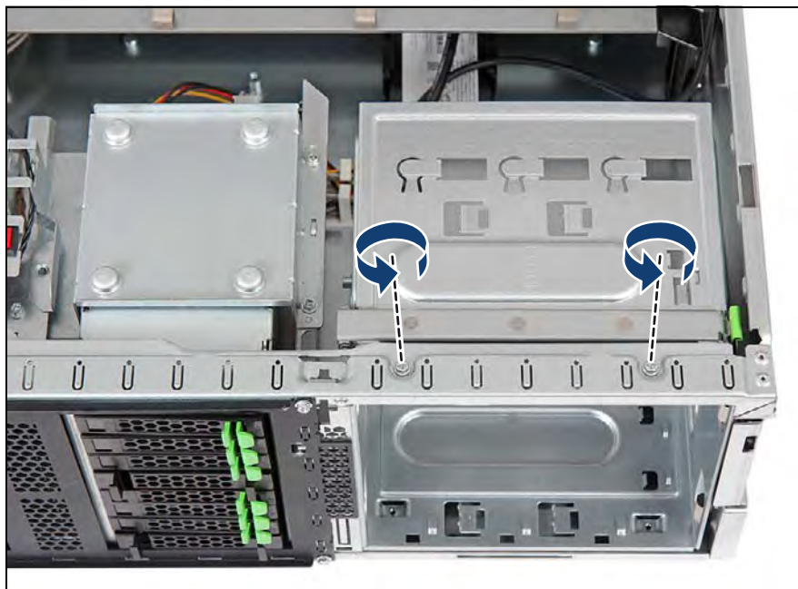
Figure 559: Detaching the accessible drive cage (C)
