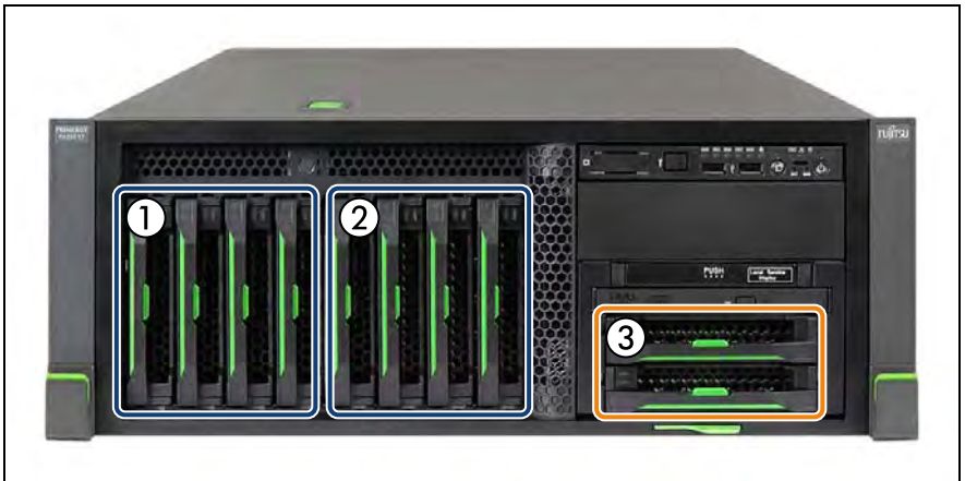
Figure 146: 3.5-inch SAS backplanes - Rack version with 2x 3.5-inch HDD extension box
