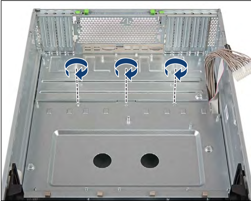
Figure 37: Mounting the system board carrier (C)
