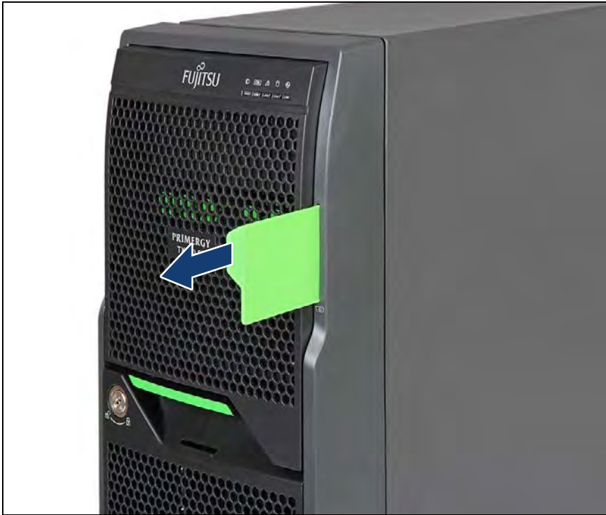
Figure 23: Removing the ID card (tower server)
