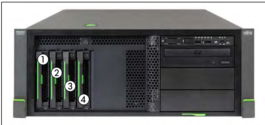
Figure 148: Mounting order: up to 4x 3.5-inch HDDs
