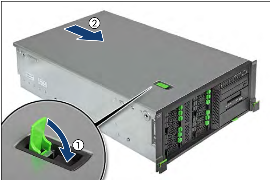
Figure 50: Mounting the top cover (rack server) (B)
