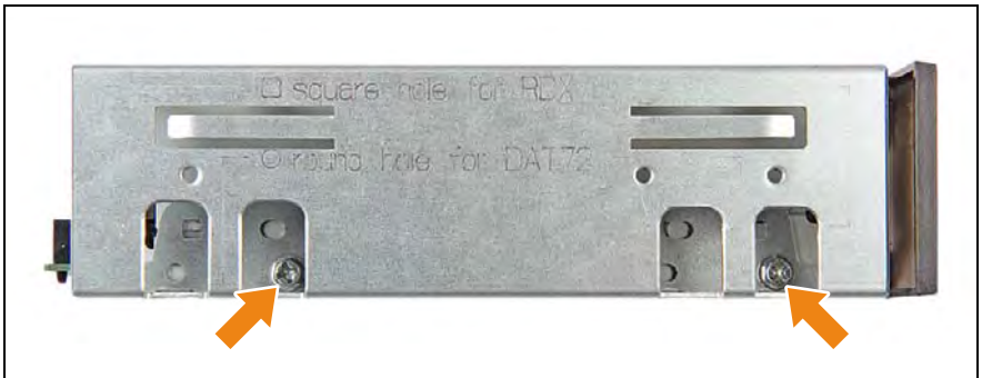
Figure 411: Securing mounting brackets to a DAT72 backup drive
