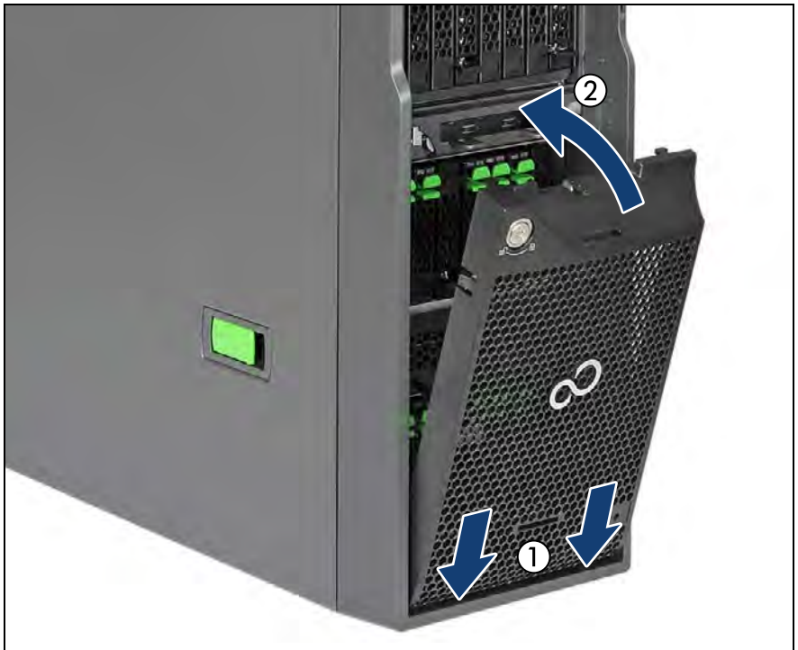
Figure 53: Installing the HDD bay cover
