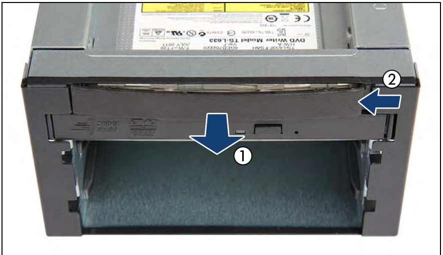
Figure 443: Removing the LSD dummy cover plate (A)
