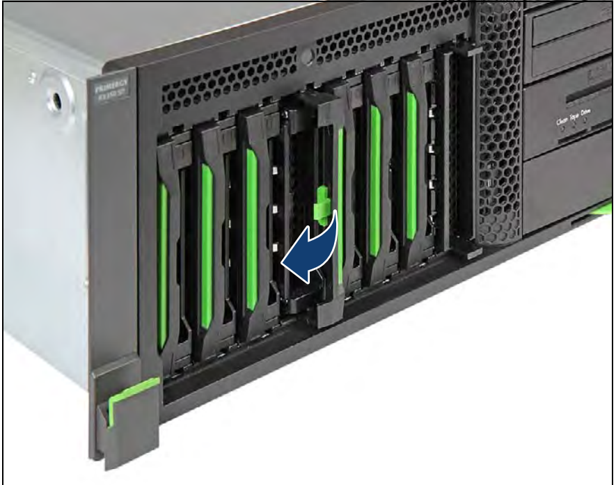
Figure 164: Closing the 3.5-inch HDD module locking lever
