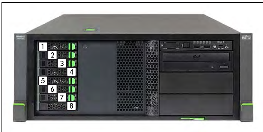
Figure 98: Naming scheme: 8x 2.5-inch HDDs / SSDs (2 SAS backplanes)
