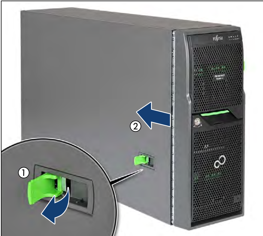
Figure 21: Removing the side cover (tower server)
