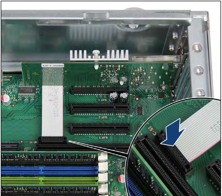
Figure 257: Connecting the NCSI sideband cable to the system board
