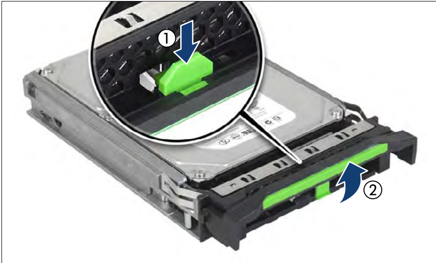
Figure 162: Opening the 3.5-inch HDD module locking lever
