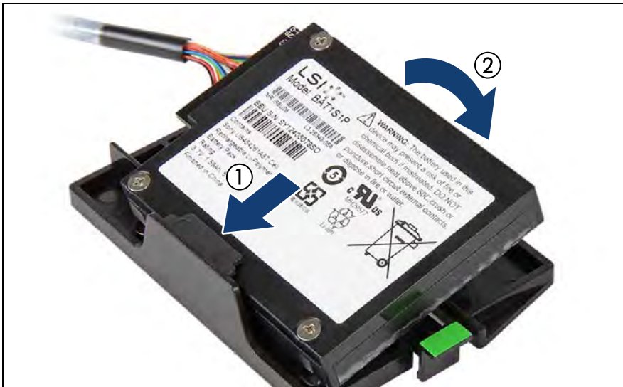
Figure 329: Installing the BBU in the BBU holder
