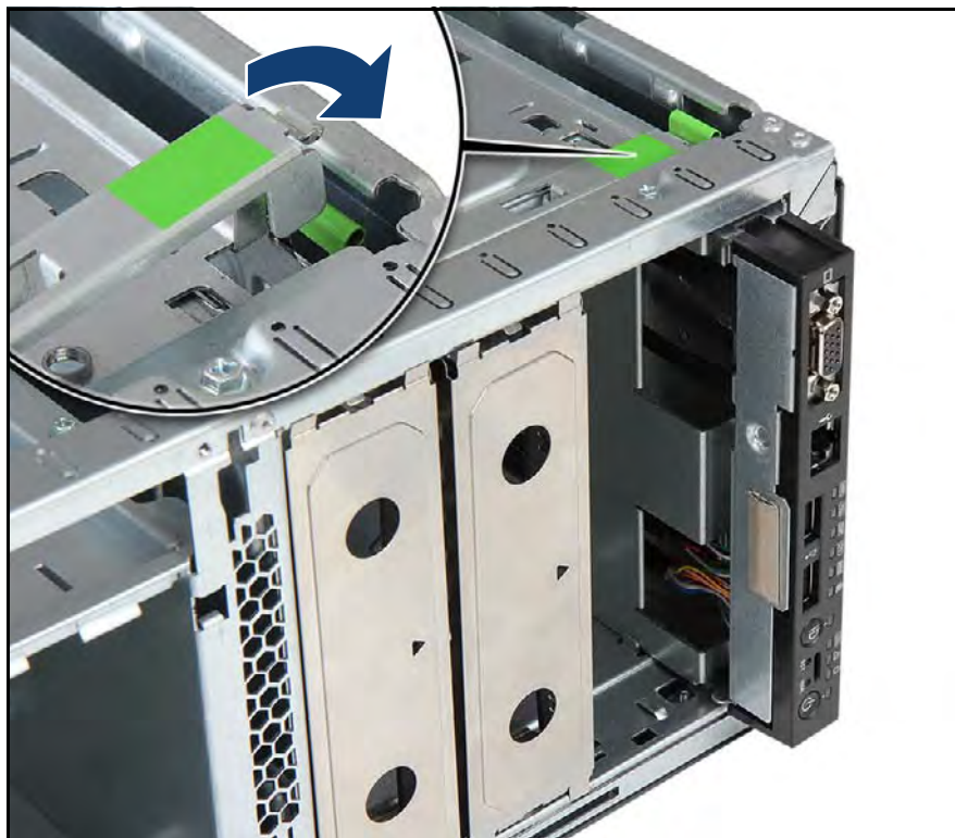
Figure 478: Securing the front panel module
