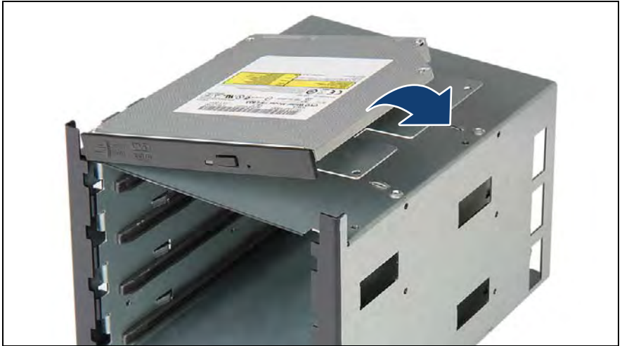
Figure 458: Installing the slimline ODD on the HDD extension box (B)
