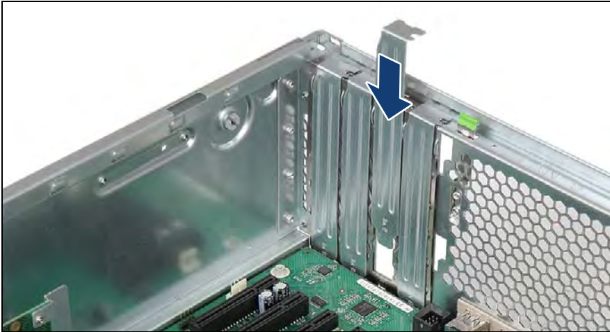
Figure 246: Installing a PCI slot bracket (A)
