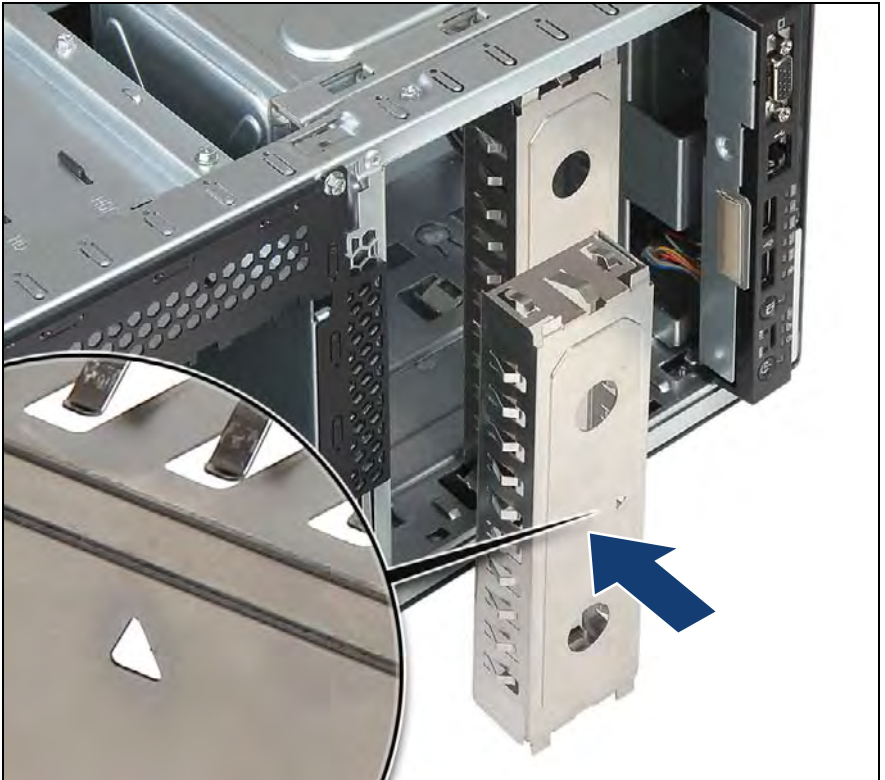
Figure 43: Installing an accessible drive filler cover
