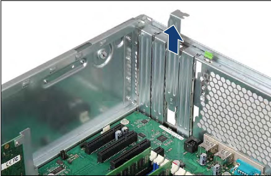
Figure 241: Removing the PCI slot bracket (B)
