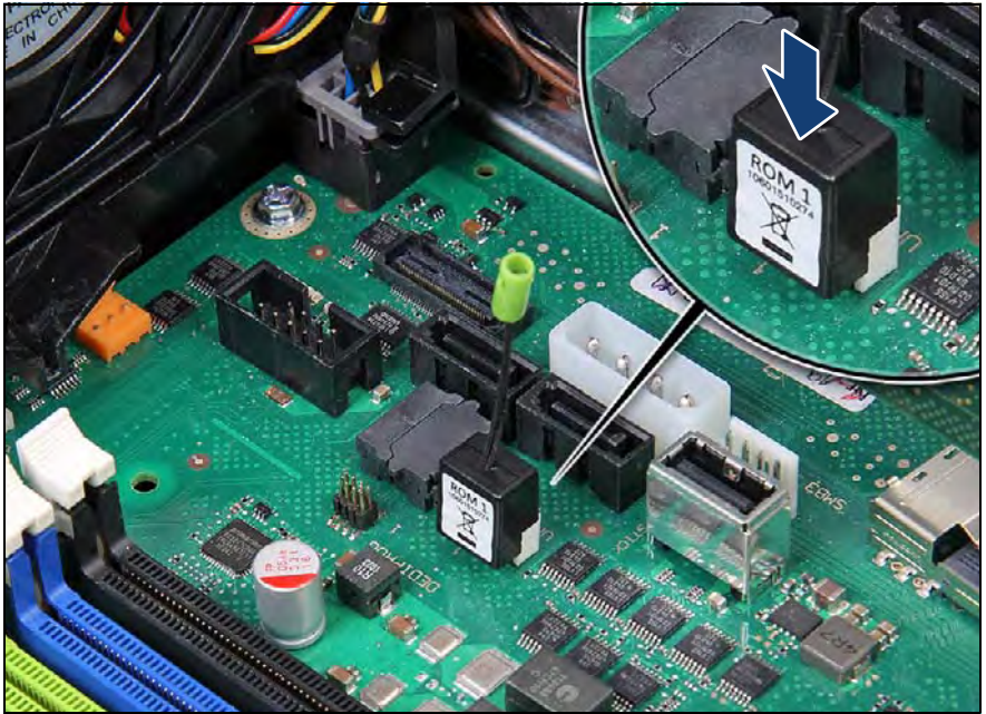
Figure 528: Onboard SAS enabling key mounting location
