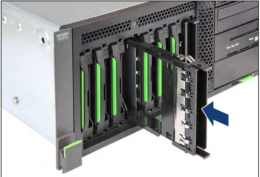
Figure 167: Installing a 3.5-inch HDD dummy module
