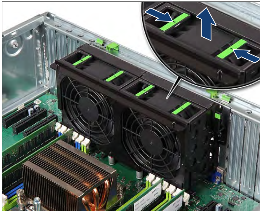
Figure 227: Removing a rear fan module (A)
