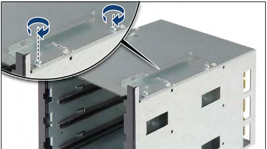
Figure 465: Reinstalling the slimline ODD mounting frame on the HDD expansion box
