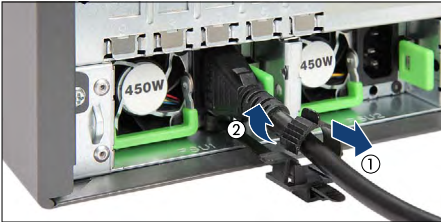
Figure 9: Removing the power cord from the PSU cable bracket (B)
