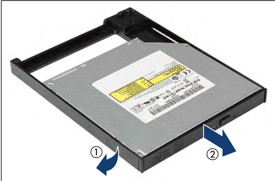
Figure 432: Removing the slimline ODD from its installation frame
