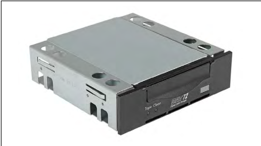
Figure 413: DAT72 backup drive with mounting brackets
