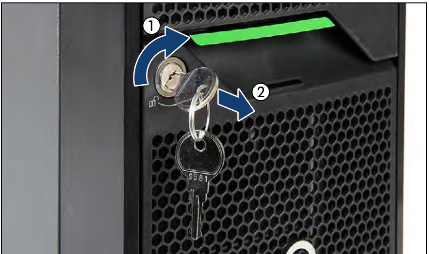
Figure 20: Unlocking the server
