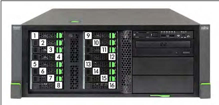
Figure 101: Naming scheme: 16x 2.5-inch HDDs / SSDs (4 SAS backplanes)
