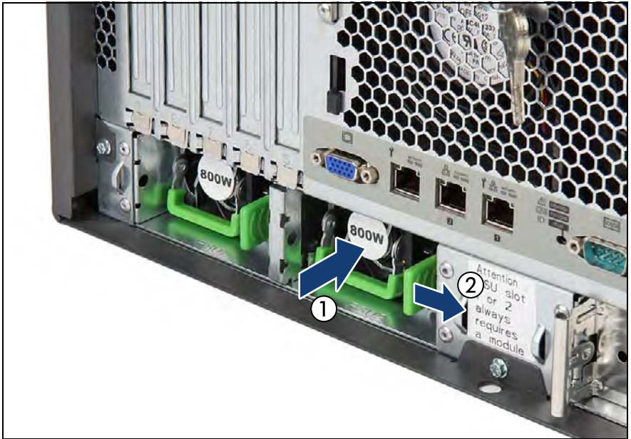
Figure 79: Installing a PSU module
