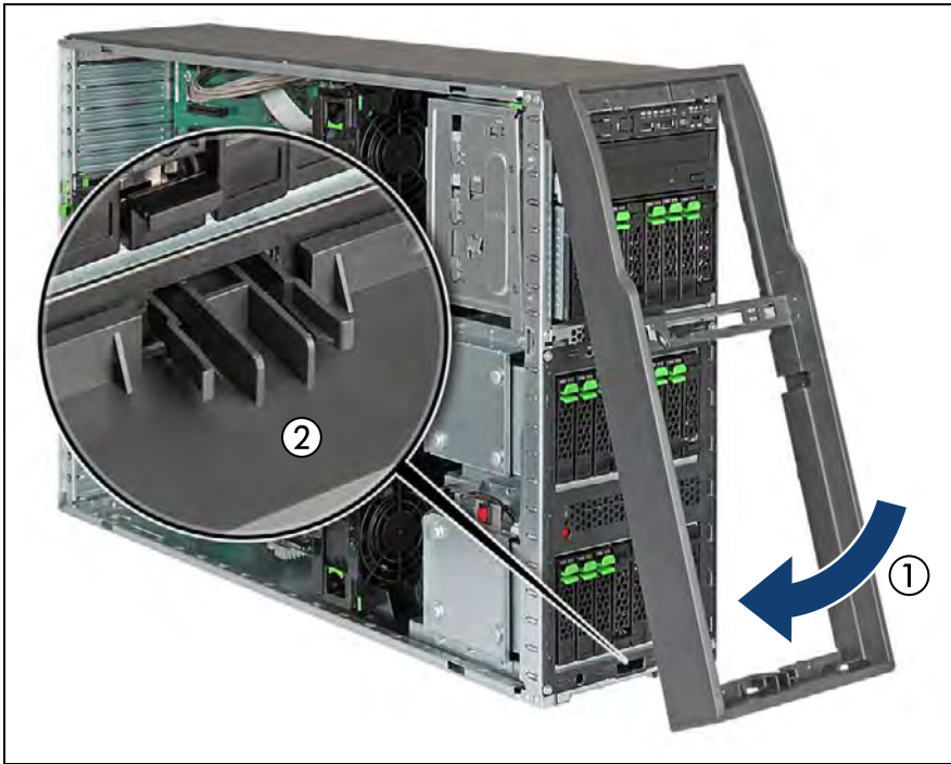
Figure 52: Mounting the front cover (tower server) (B)
