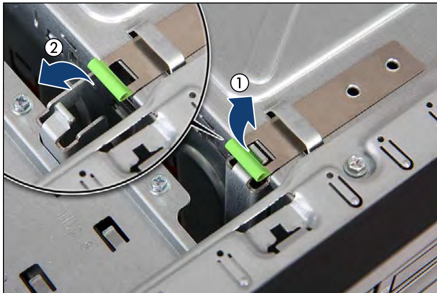
Figure 39: Opening the accessible drive locking bar (rack systems)
