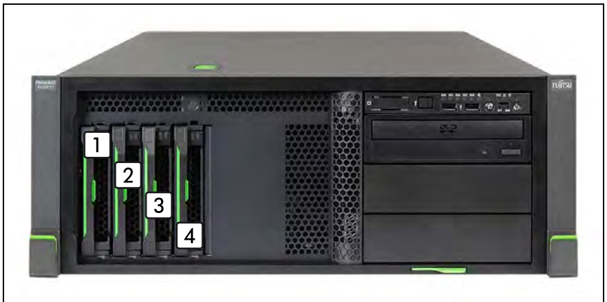
Figure 149: Naming scheme: 4x 3.5-inch HDDs (1 SAS backplane)
