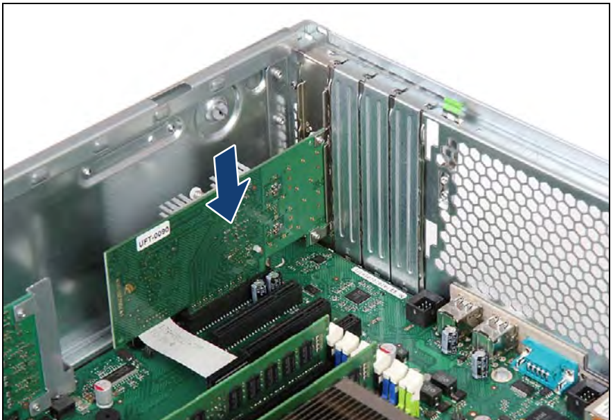
Figure 255: Installing the Modular LAN controller
