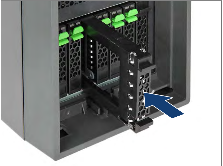
Figure 114: Installing a 2.5-inch HDD / SSD dummy module
