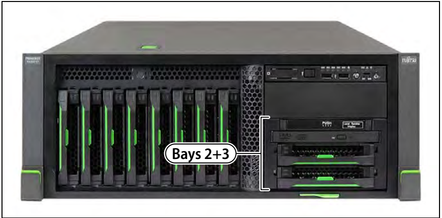
Figure 194: 2x 3.5-inch HDD extension box - Rack version
