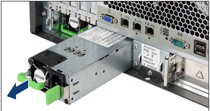
Figure 81: Removing a PSU module (B)
