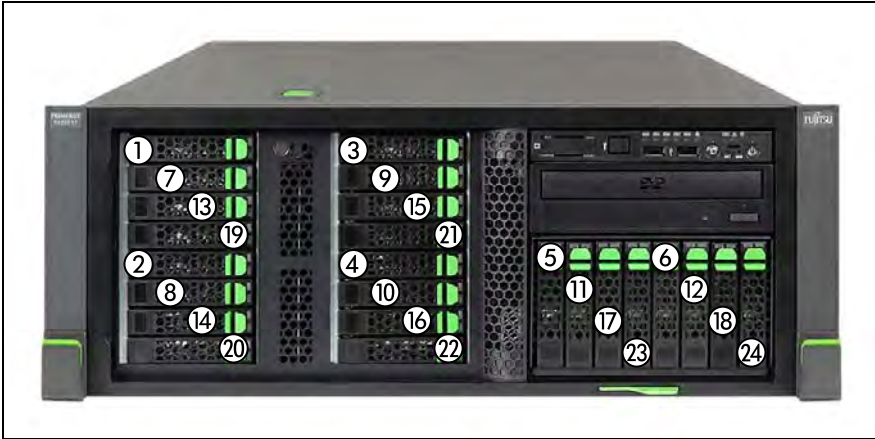
Figure 102: Mounting order: up to 24x 2.5-inch SAS 2.0 HDDs / SSDs (Rack)
