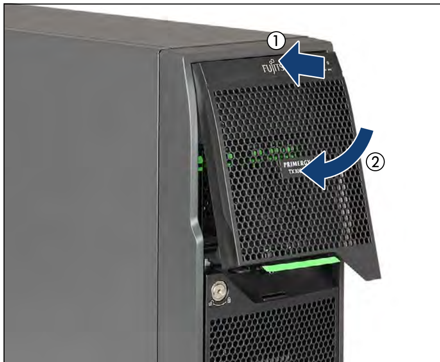
Figure 54: Installing the accessible drive bay cover
