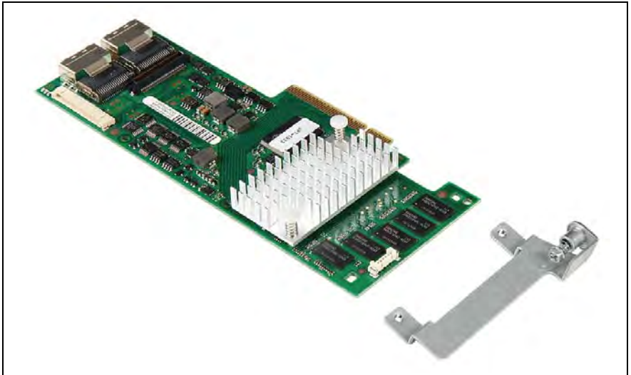
Figure 321: SAS RAID controller with RAID card holder (C26361-K644-B944)
