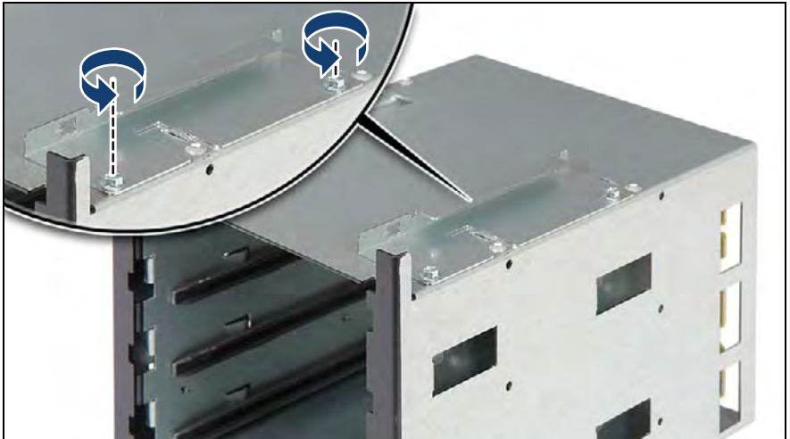
Figure 454: Removing the slimline ODD mounting bracket
