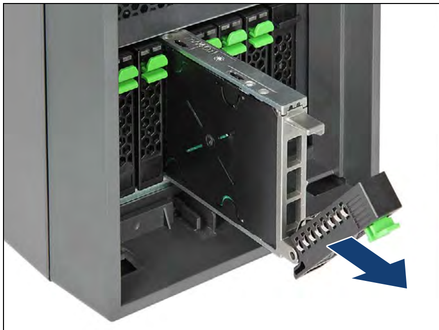
Figure 113: Removing a 2.5-inch HDD / SSD module
