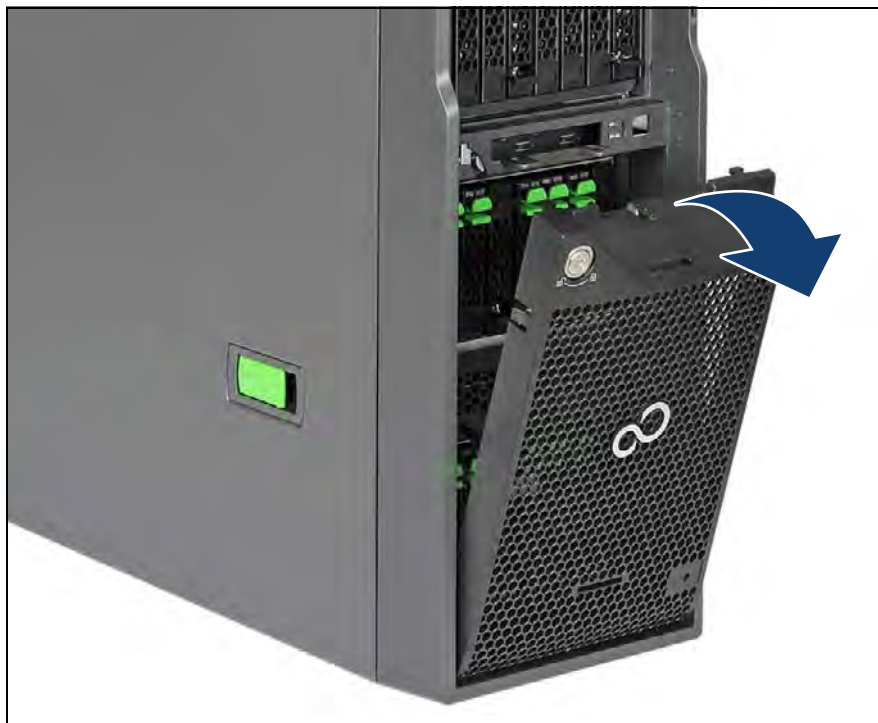
Figure 25: Removing the HDD bay cover
