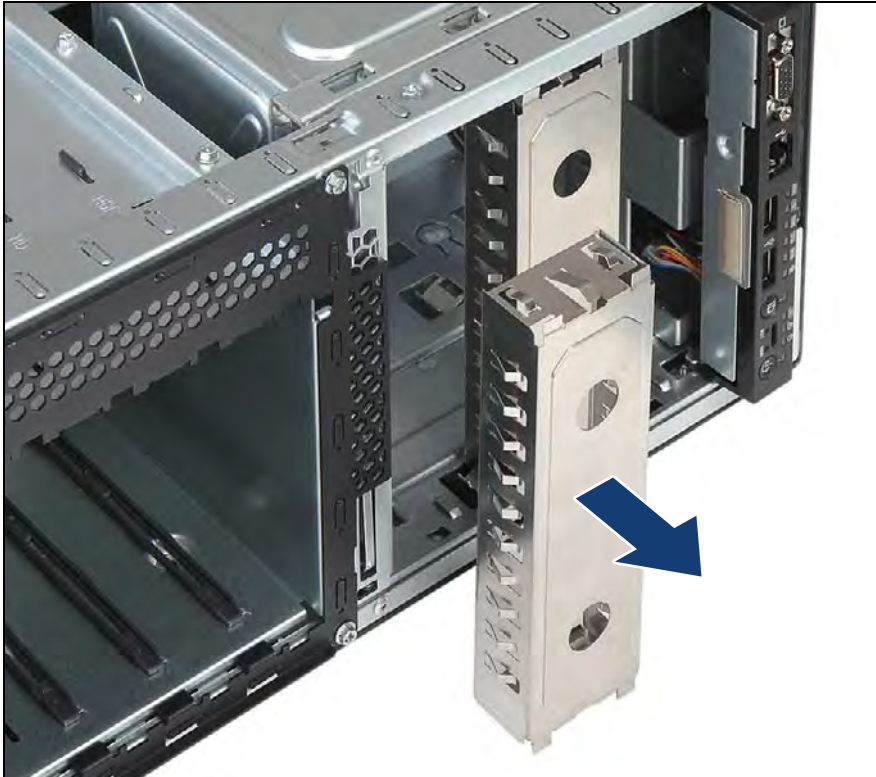
Figure 42: Removing an accessible drive filler cover
