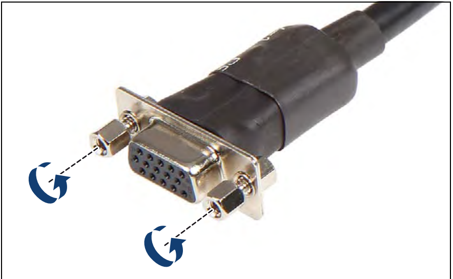
Figure 498: Preparing the front VGA cable
