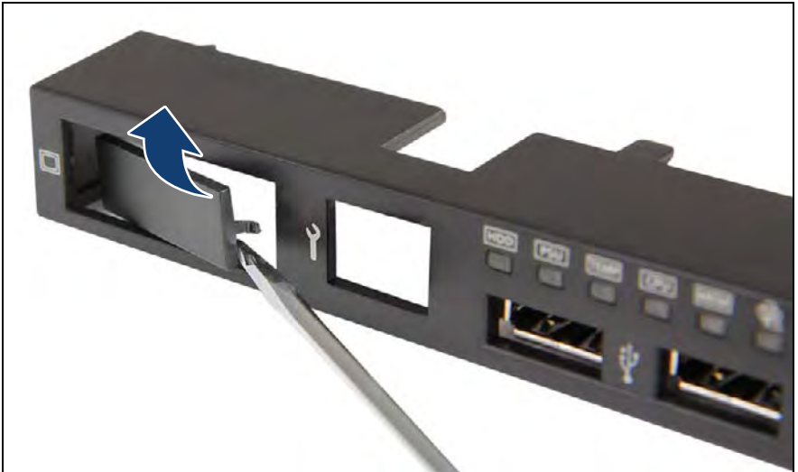
Figure 496: Breaking out the front VGA cover plate
