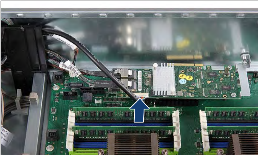
Figure 332: Connecting the BBU cable to the controller
