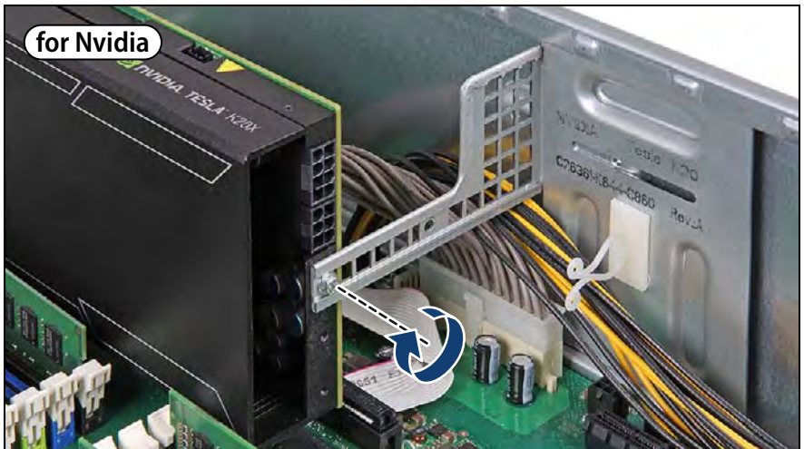
Figure 288: Securing the GPGPU card (Nvidia) (C)
