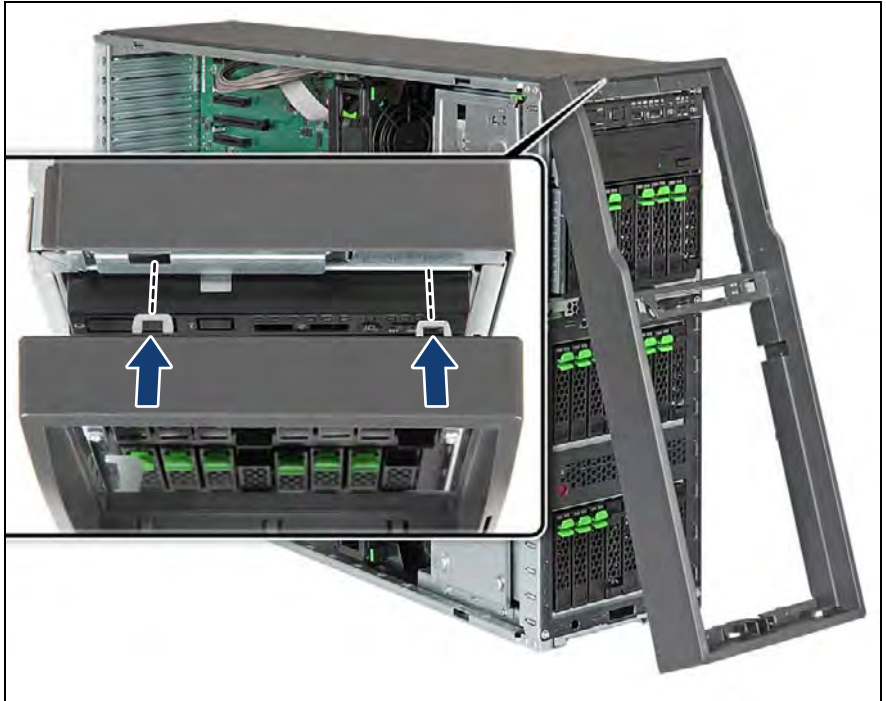
Figure 51: Mounting the front cover (tower server) (A)
