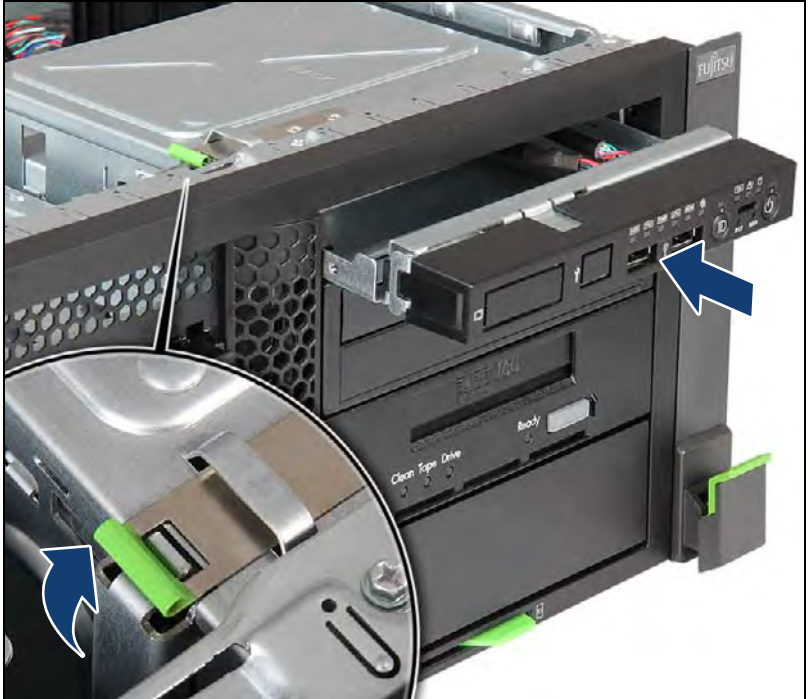
Figure 479: Securing the front panel module (rack systems)
