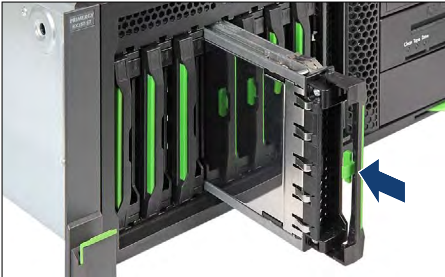
Figure 163: Inserting the 3.5-inch HDD module
