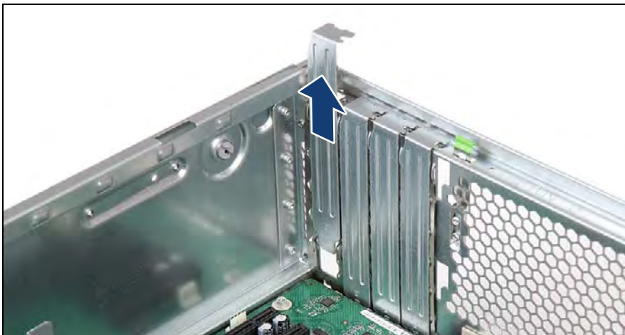
Figure 254: Removing the PCI slot bracket (B)
