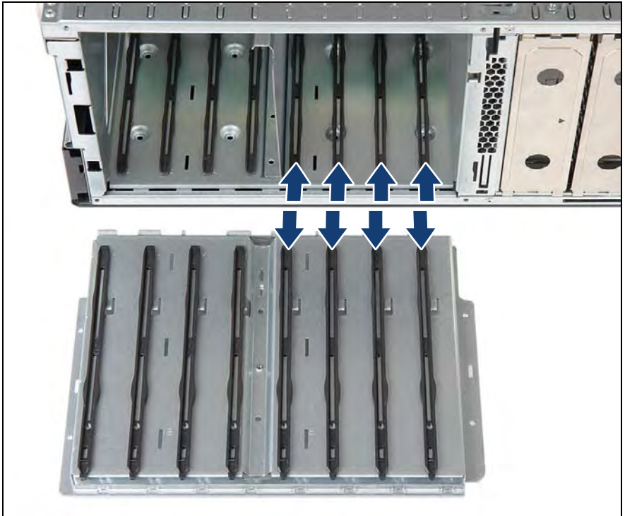
Figure 183: Adding HDD mounting rails
