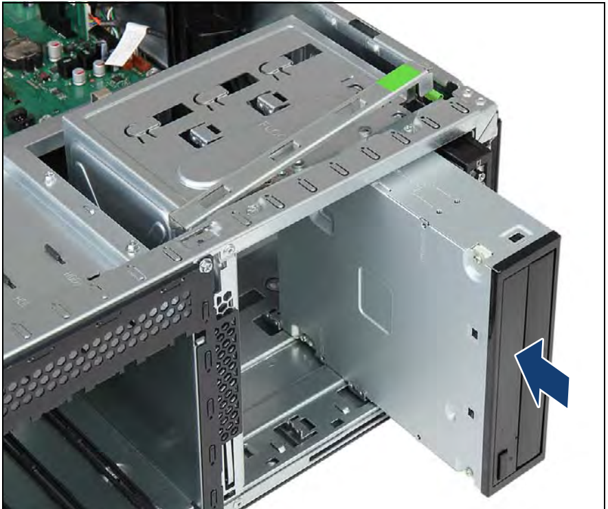
Figure 407: Inserting the accessible drive
