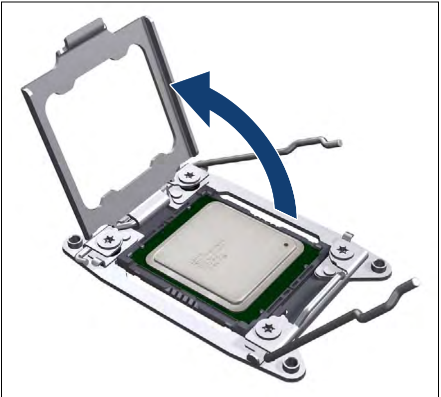
Figure 388: Opening the load plate (B)
