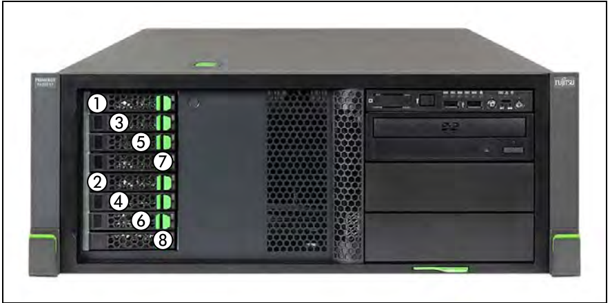
Figure 97: Mounting order: up to 8x 2.5-inch HDDs / SSDs
