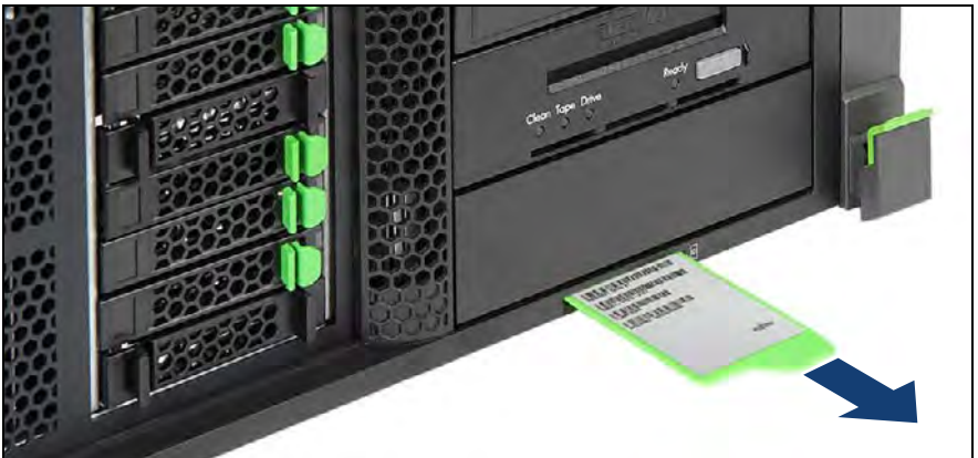
Figure 14: Removing the ID card (rack server)
