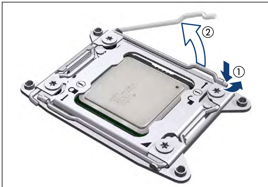
Figure 385: Opening socket release lever 1
