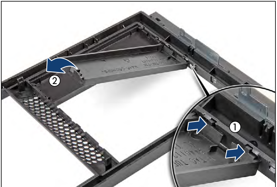
Figure 575: Installing accessible drive dummy covers
