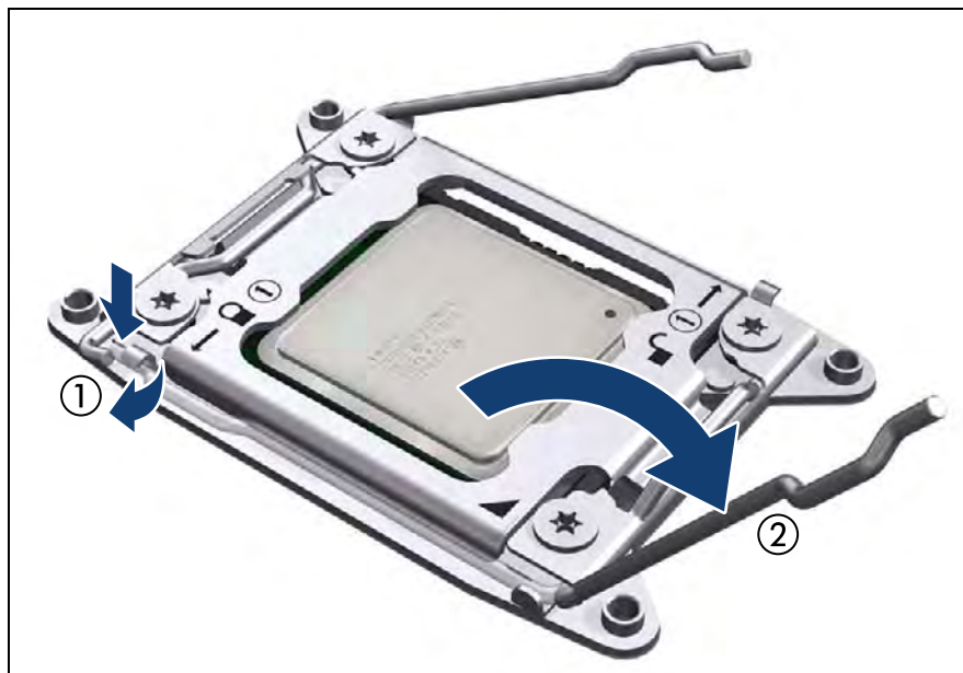
Figure 376: Opening socket release lever 2
