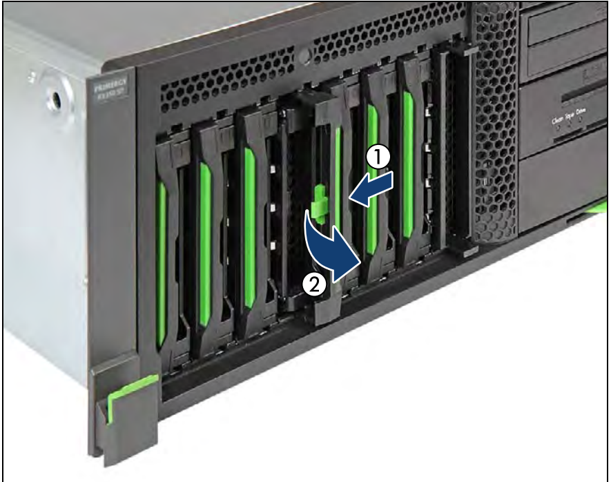
Figure 165: Disconnecting a 3.5-inch HDD module
