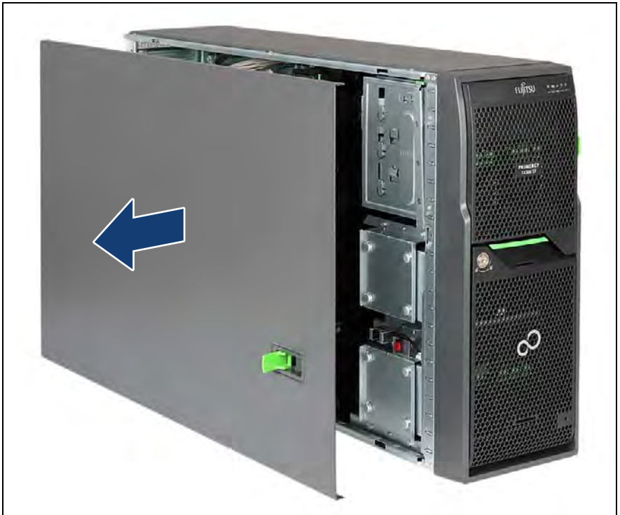
Figure 22: Removing the side cover (tower server)
