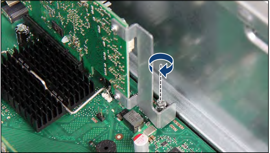
Figure 324: Securing the SAS RAID controller
