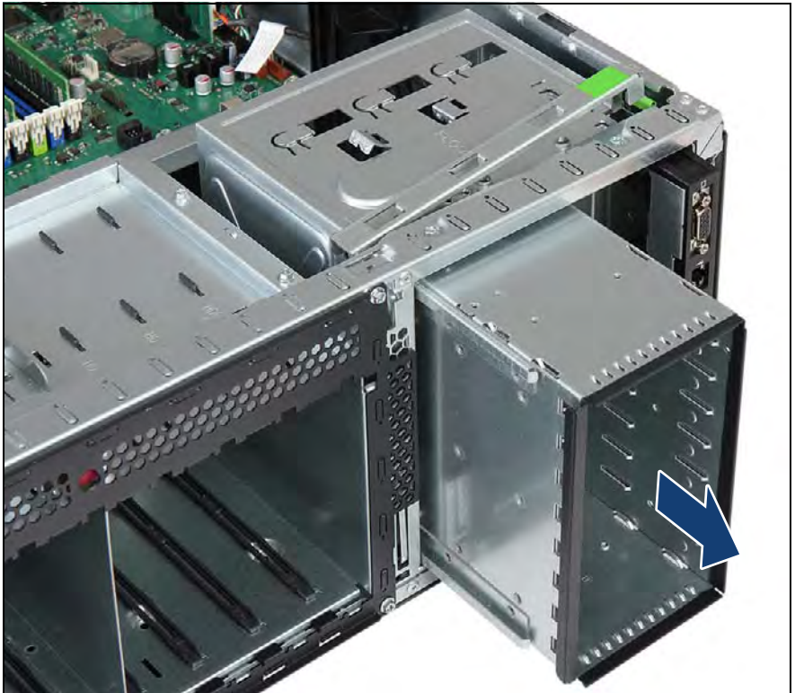
Figure 206: Removing the HDD extension box
