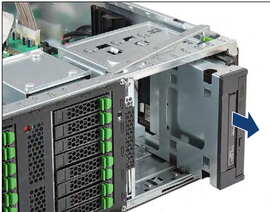
Figure 430: Removing the Multibay box
