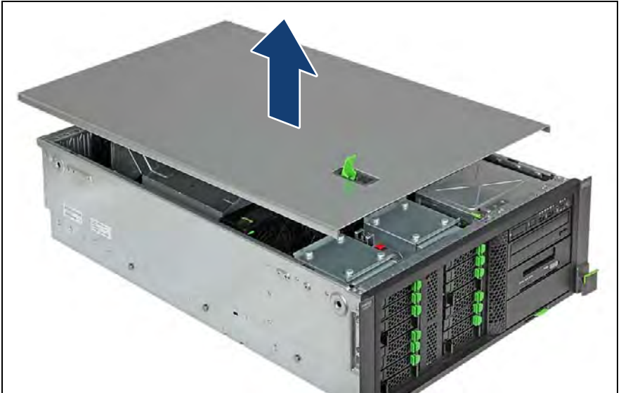
Figure 13: Removing the top cover (rack server)
