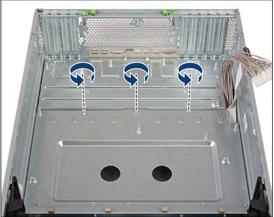
Figure 32: Removing the system board carrier (A)
