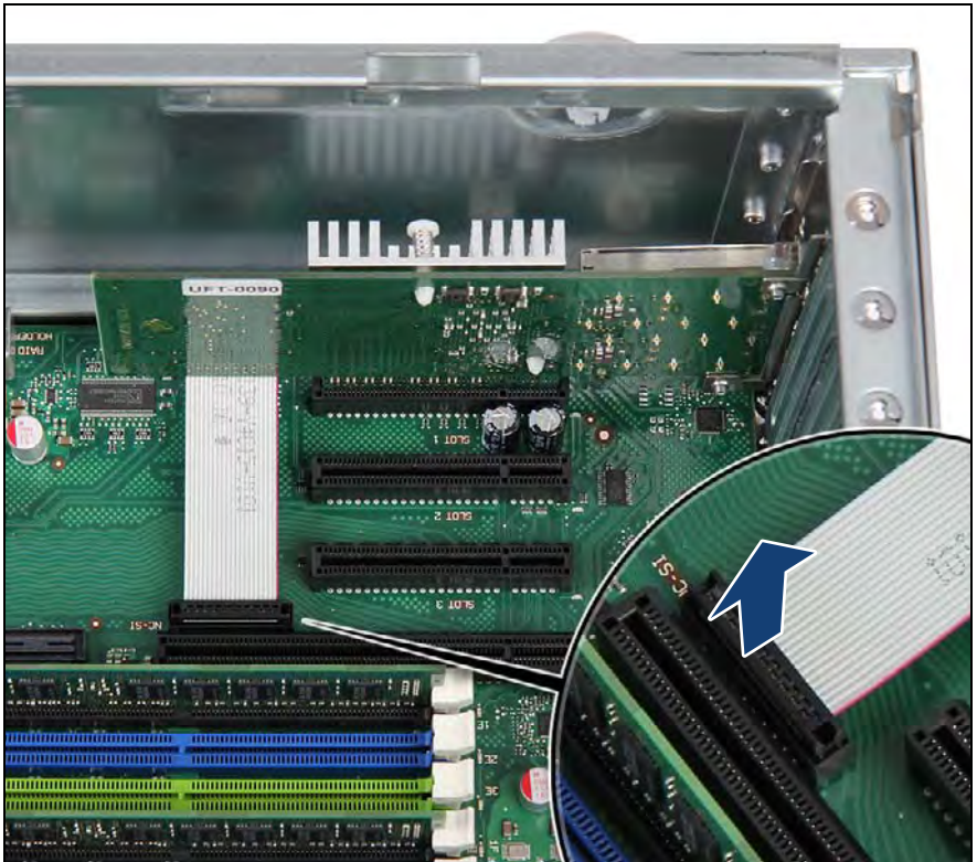
Figure 259: Disconnecting the NCSI sideband cable
