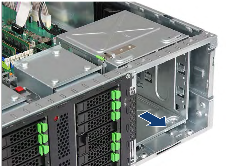
Figure 565: Mounting the accessible drive cage (B)
