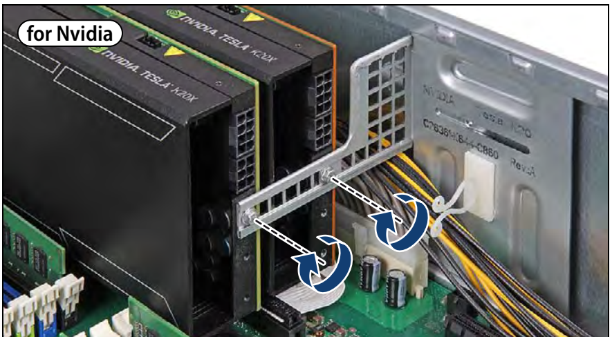
Figure 292: Installing the secondary GPGPU card (Nvidia)
