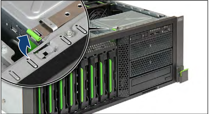
Figure 320: Installing perforated drive cover modules (B)
