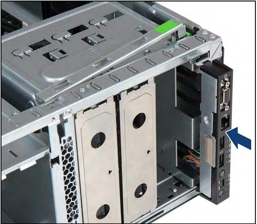
Figure 477: Installing the front panel module
