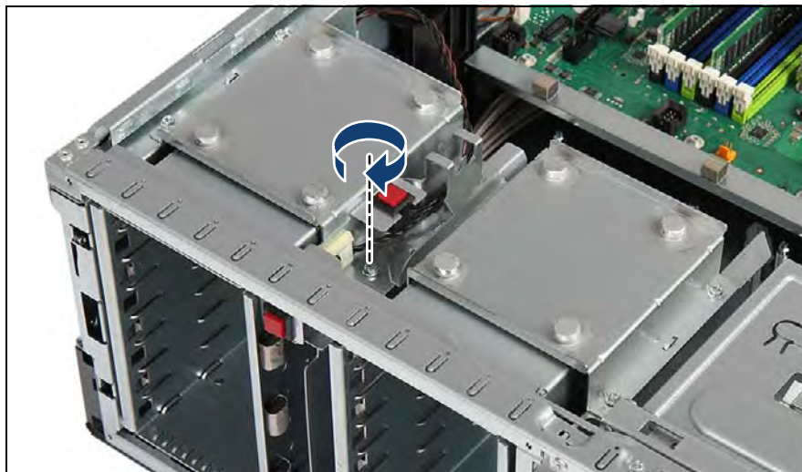
Figure 131: Installing the intrusion switch holder (B)
