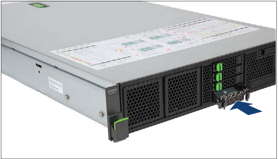
Figure 49: Installing a 2.5-inch dummy module
