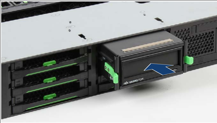
Figure 195: Installing the drive cage with the tape/RDX drive
