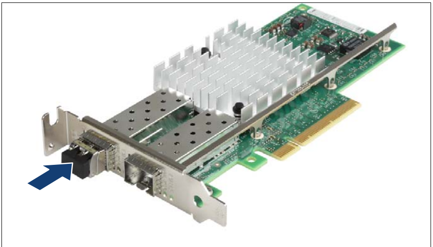
Figure 131: Attaching the protective optical port plug
