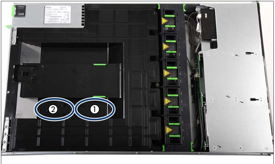
Figure 101: BBU / FBU mounting positions
