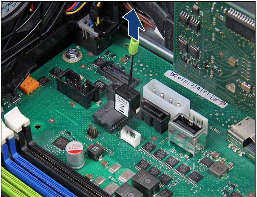
Figure 290: onboard SAS enabling key mounting location
