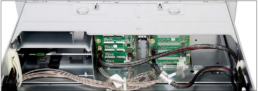
Figure 60: Reconnecting cables to the 4x 2.5-inch HDD SAS 3.0 backplane
