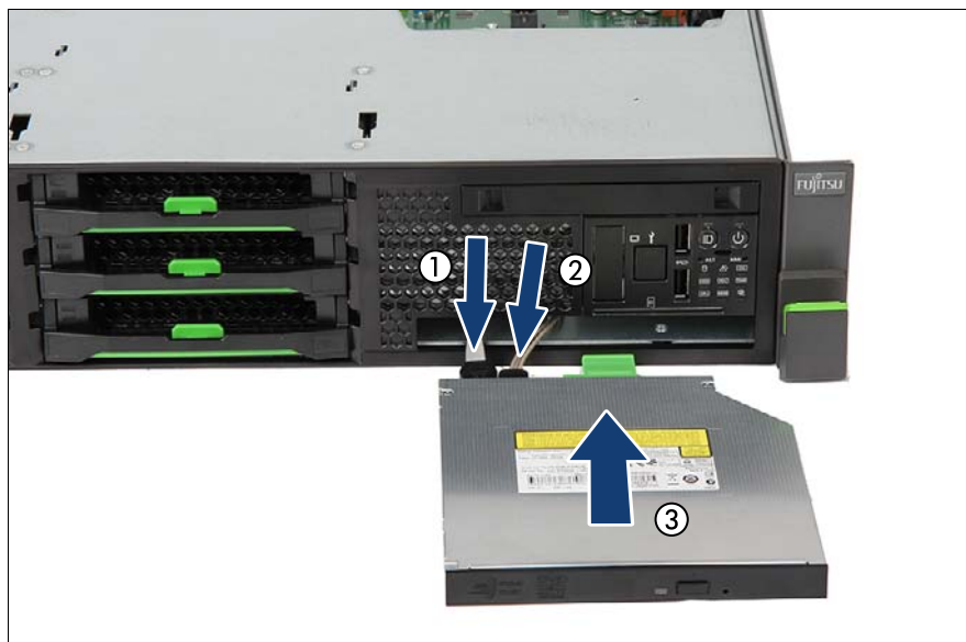
Figure 186: Installing the ODD
