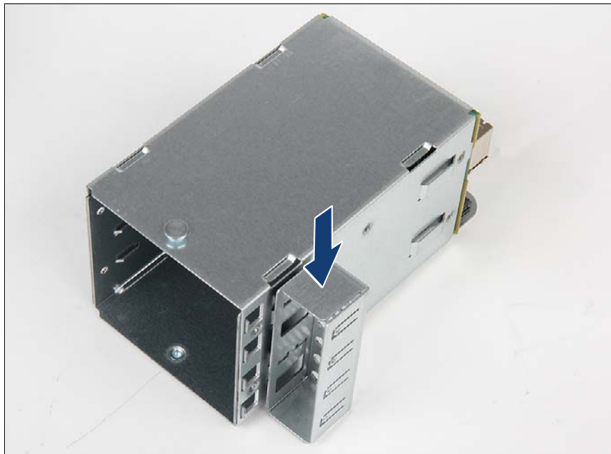
Figure 313: Installing the cover plate to a HDD cage.
