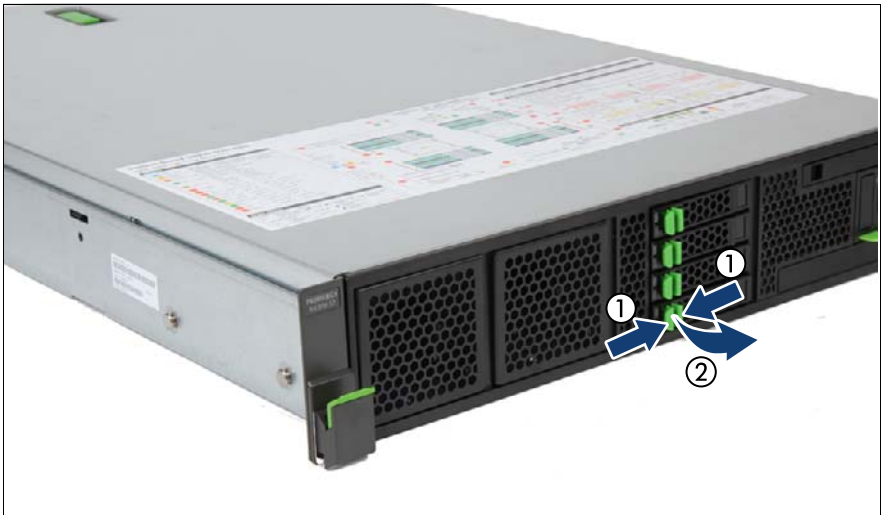
Figure 47: Disconnecting a 2.5-inch HDD / SSD module
