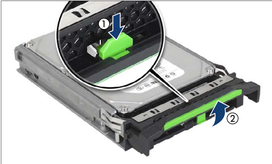
Figure 34: Opening the 3.5-inch HDD module locking lever
