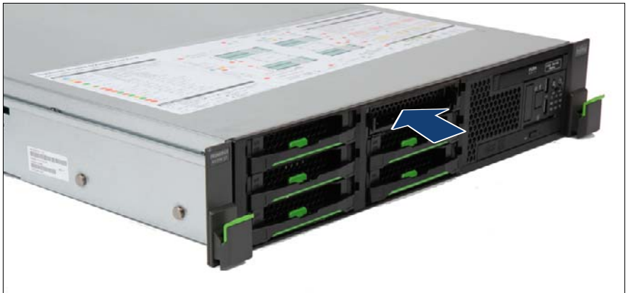
Figure 37: Installing a 3.5-inch dummy module
