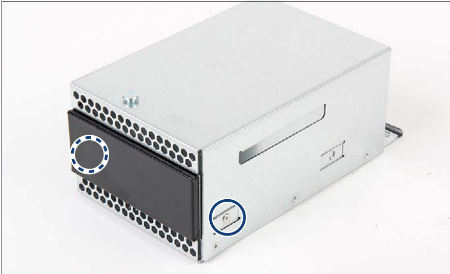
Figure 214: Installing tape drive dummy module
