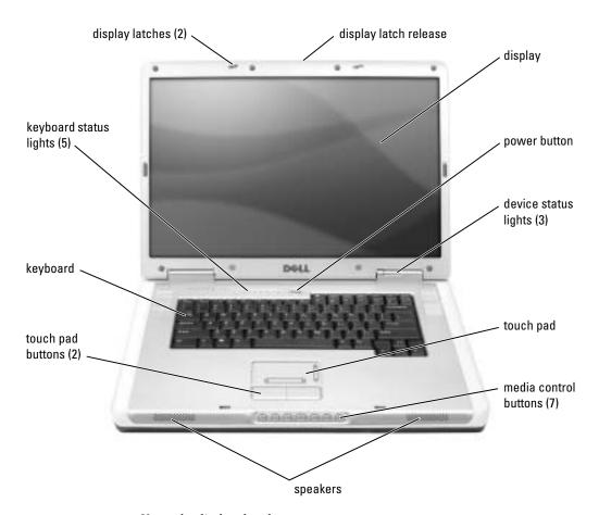
**DISPLAY LATCHES** — Keeps the display closed.
