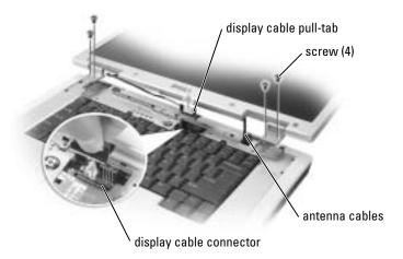
7 Lift the display away from the computer at a 90-degree angle. Ensure that the antenna cables and display cable are free from the routing channels and that the cables move freely when you lift the display.
