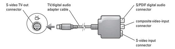
Your TV has either an S-video input connector or a composite video-input connector. Depending on what type of connector is available on your TV, you can use a commercially available S-video cable or composite video cable to connect your computer to your TV. For audio devices without support for S/PDIF digital audio, you can use the audio connector on the side of the computer to connect the computer to your audio device.
