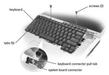
NOTICE: To avoid scratching the palm rest when replacing the keyboard, hook the five tabs along the front edge of the keyboard into the palm rest, and then secure the keyboard in place.
