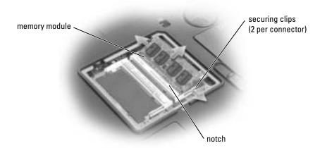
NOTICE: If you need to install memory modules in two connectors, install a memory module in the connector labeled "DIMMA" before you install a module in the connector labeled "DIMMB." Insert memory modules at a 45-degree angle to avoid damaging the connector.
