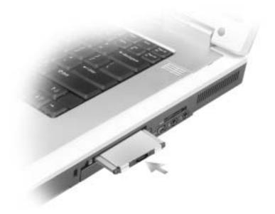
The computer recognizes most PC Cards and automatically loads the appropriate device driver. If the configuration program tells you to load the manufacturer's drivers, use the floppy disk or CD that came with the PC Card.
