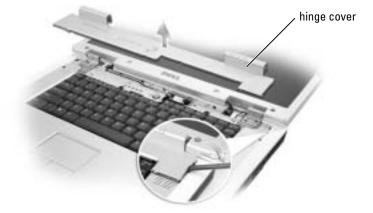
When replacing the hinge cover, first insert the left edge and then press from left to right until the cover snaps into place.
