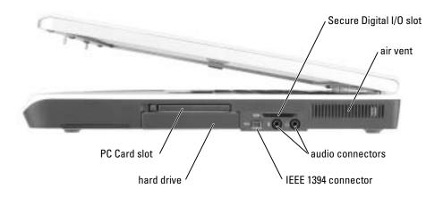
**SECURE DIGITAL I/O SLOT** — The Secure Digital I/O slot supports one Secure Digital memory card or other SDI/O device. Use Secure Digital memory cards to save or back up data.
