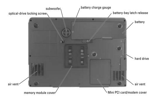
**BATTERY CHARGE GAUGE** — Provides information on the battery charge. For more information, see "Checking the Battery Charge" on page 30.
