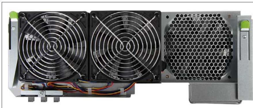
Figure 113: System fan holder with three system fans (fan 1-3)
