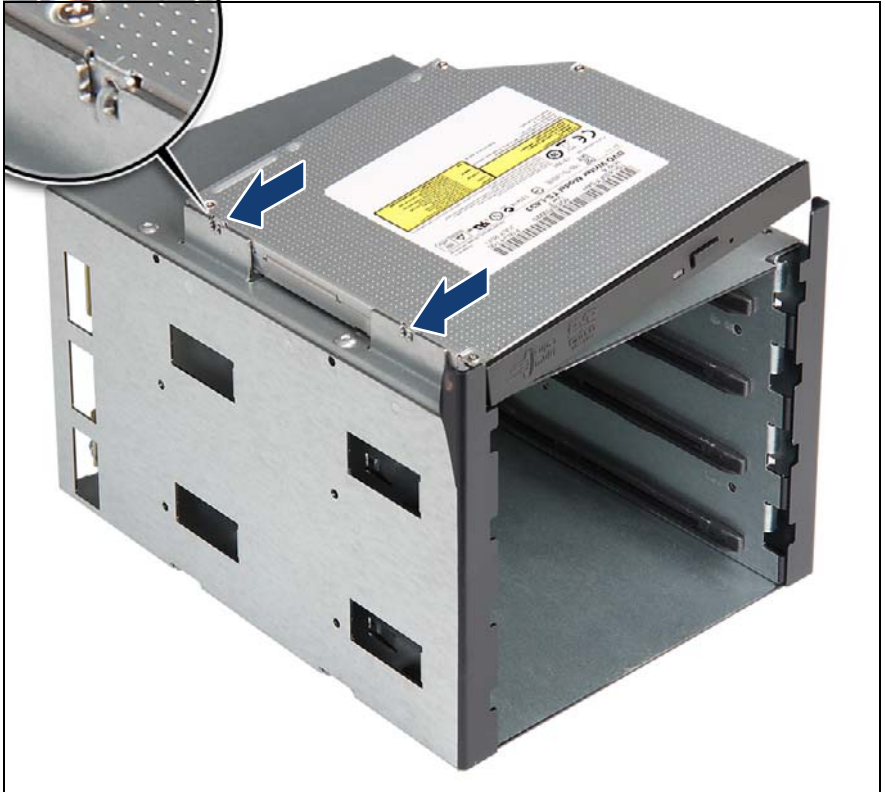
Figure 237: Installing the slimline ODD on the HDD extension box
