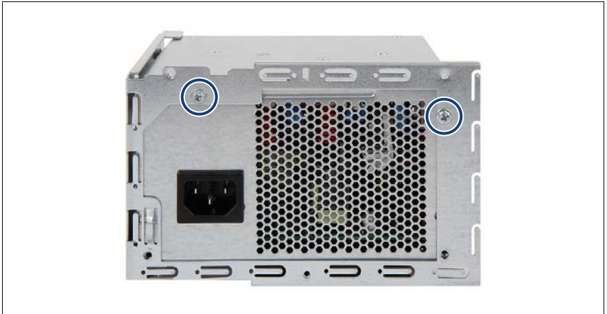
Figure 42: Removing the power supply unit from the installation frame (A)
