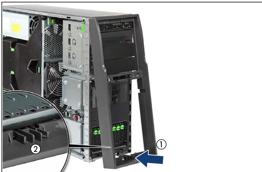
Figure 23: Installing the front cover (tower server) (B)
