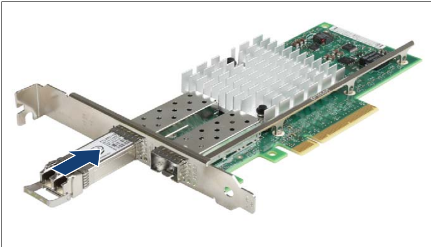
Figure 134: Inserting the SFP+ transceiver module
