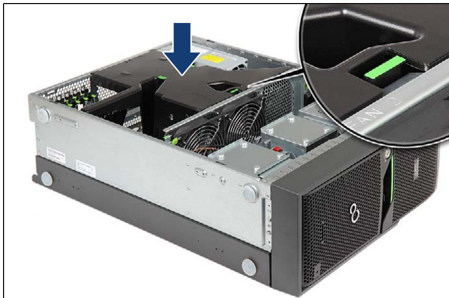
Figure 17: Installing the system air duct
