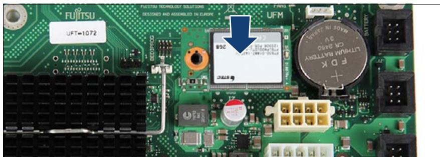
Figure 272: Installing the UFM (A)
