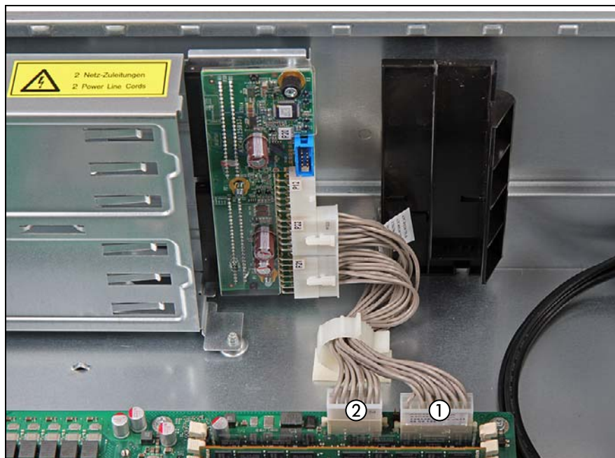
Figure 58: Connecting cables (A)
