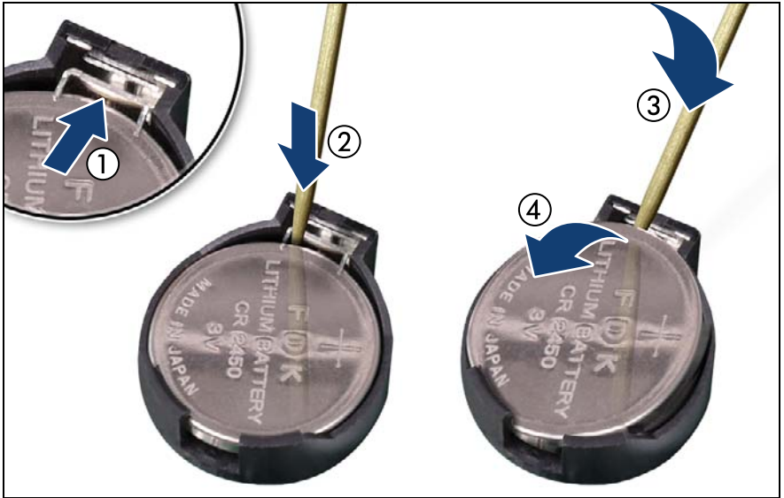
Figure 264: Replacing the CMOS battery
