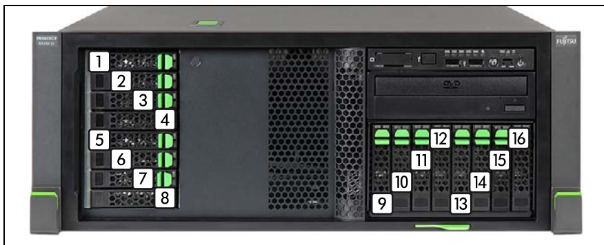
Figure 66: Naming scheme with 16 2.5-inch HDDs (4 SAS backplanes)
