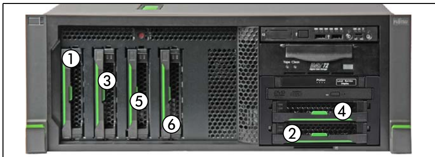
Figure 77: Mounting order with up to 6 3.5-inch HDDs (2 SAS backplanes) - Rack version
