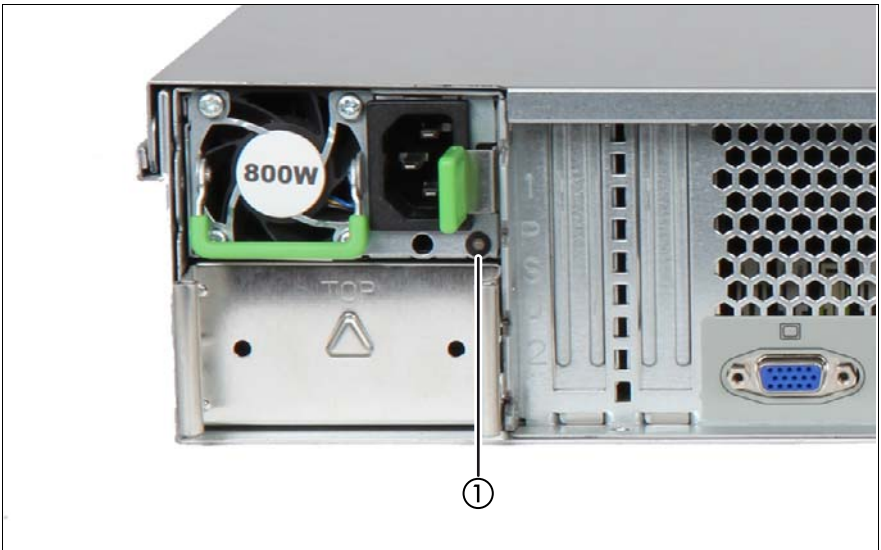
Figure 11: Indicator on hot-plug power supply unit (example AC power supply unit)
