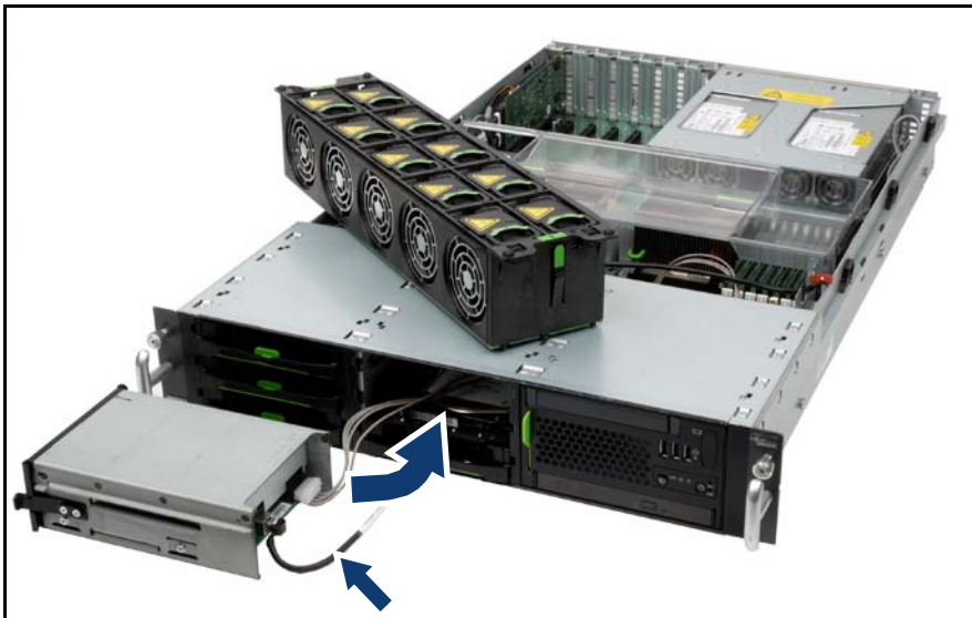
Figure 44: Pushing the USB tape drive into the server
