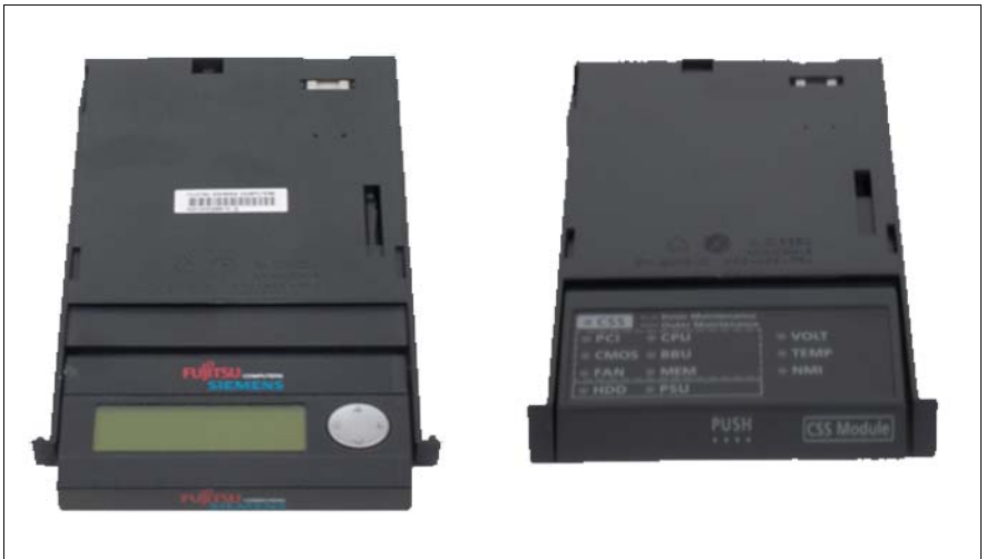
Figure 25: ServerView Local Service Display and ServerView Local Service Panel
