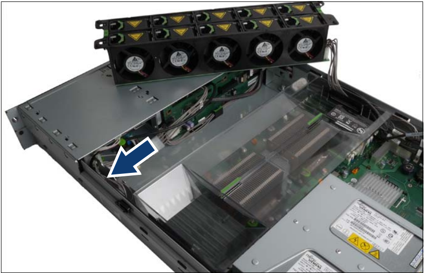
Figure 53: Routing the USB cable and power supply cable through the fan box holder and air duct holder
