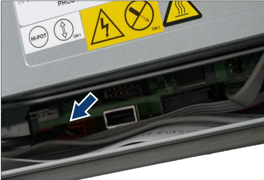
Figure 64: Connecting the USB cable for the tape drive to the system board
