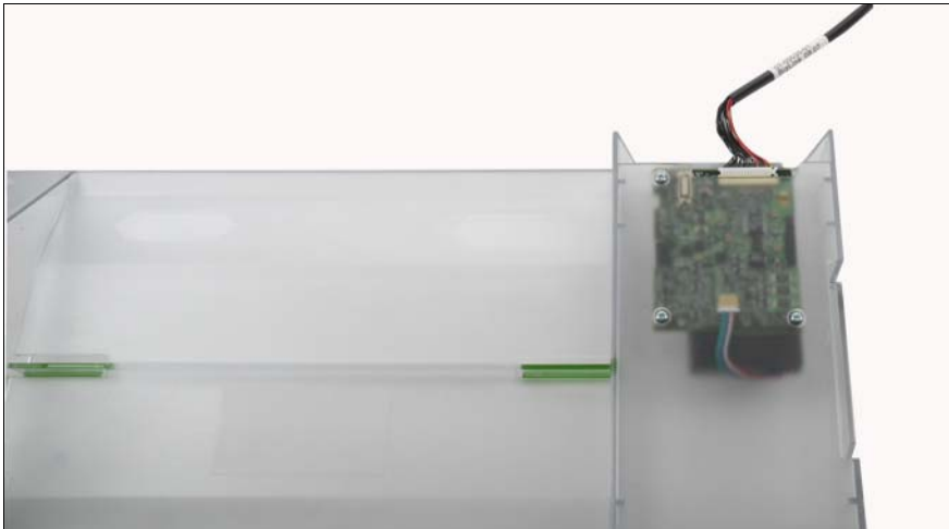
Figure 73: Screwing the BBU to the air duct
