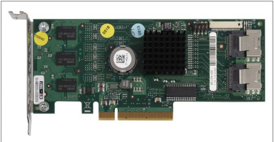
Figure 68: SAS RAID controller with a low profile rear cover
