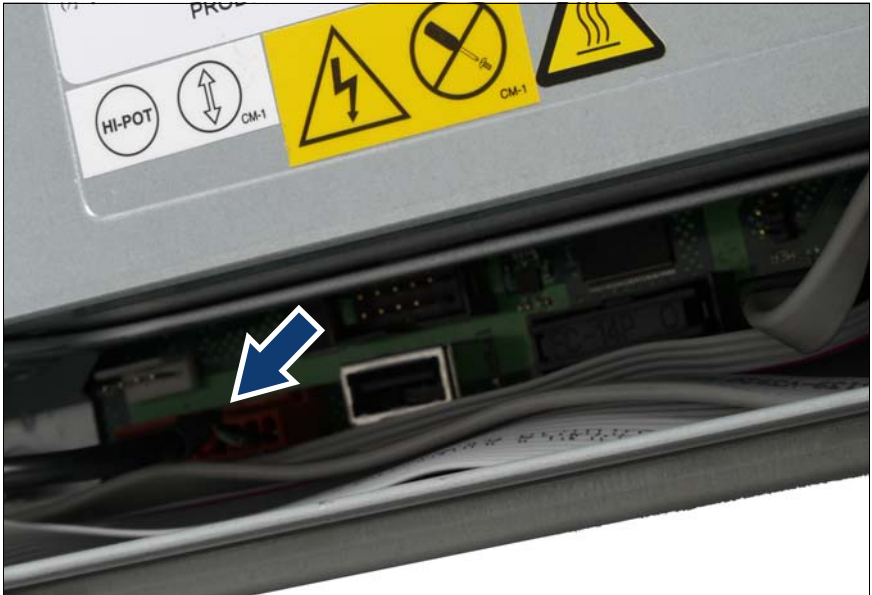
Figure 60: Connecting the USB cable for the tape drive to the system board
