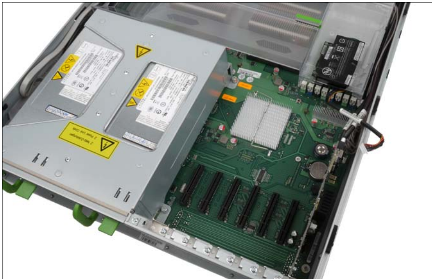
Figure 74: Inserting the air duct
