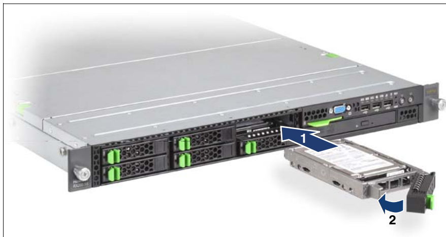
Figure 22: Installing the 2.5-inch HDD module
