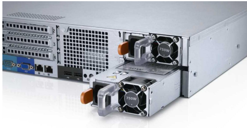
Figure 7. 750W power supply unit
