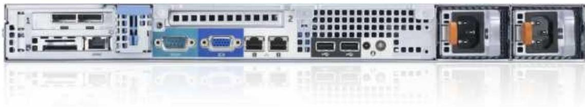
The chassis design of the R320 is optimized for easy access to components and for airflow for effective and efficient cooling. The R320 supports up to 6 DIMMs, 1 processor, hot-plug redundant power supplies, and many other components and features described in this guide.
