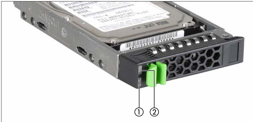
Figure 15: Indicators on the 2.5 inch HDD modules
