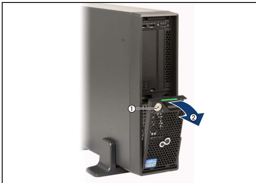
Figure 12: Removing the HDD cover
