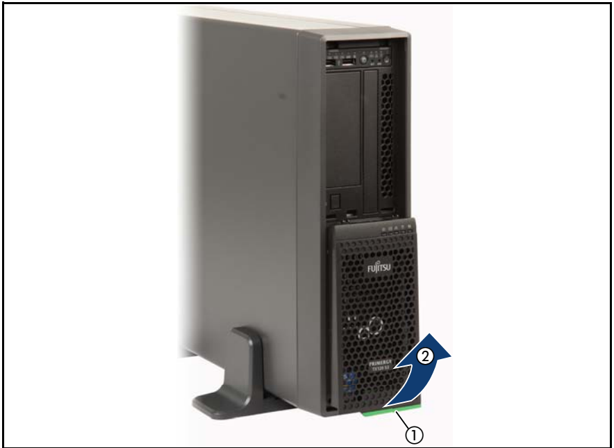
Figure 11: Removing the drive cover from the HDD cover
