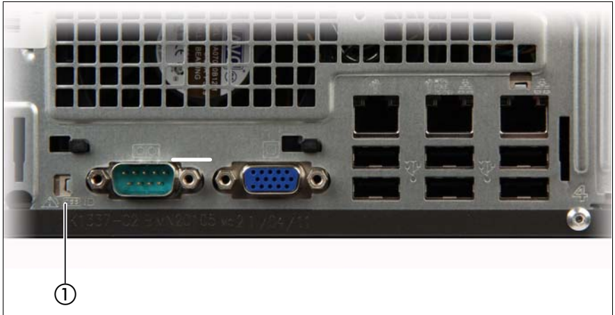
Figure 16: Indicators on the connector panel: CSS, Global Error and ID indicators
