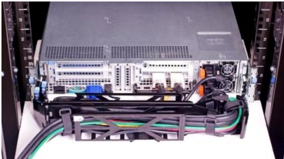
Figure 23. R810 CMA Mounted on the Side Opposite the Power Supplies (Recommended)
