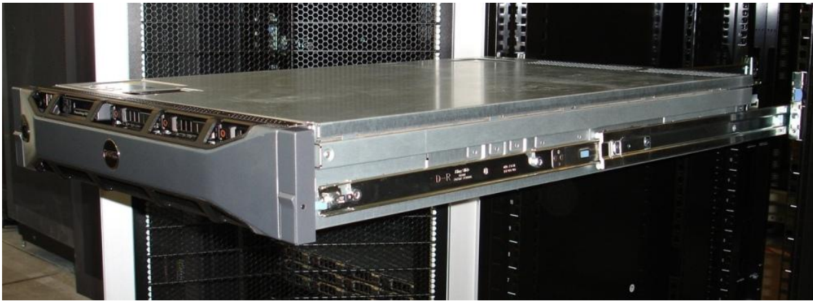
Figure 22. R810 Mounted in the B2 Sliding Rails
