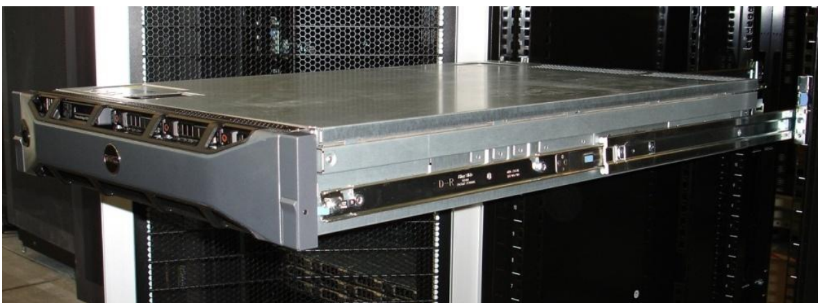
Figure 12. R715 Mounted in the B2 Sliding Rails
