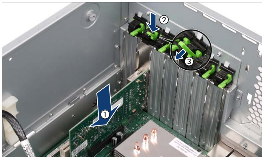
Figure 29: Installing the expansion card
