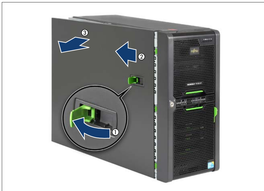
Figure 2: Opening the server
