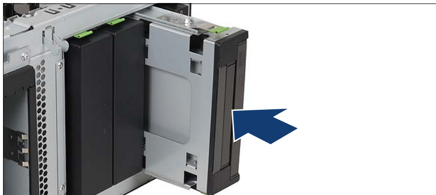
Figure 25: Installing the multibay
