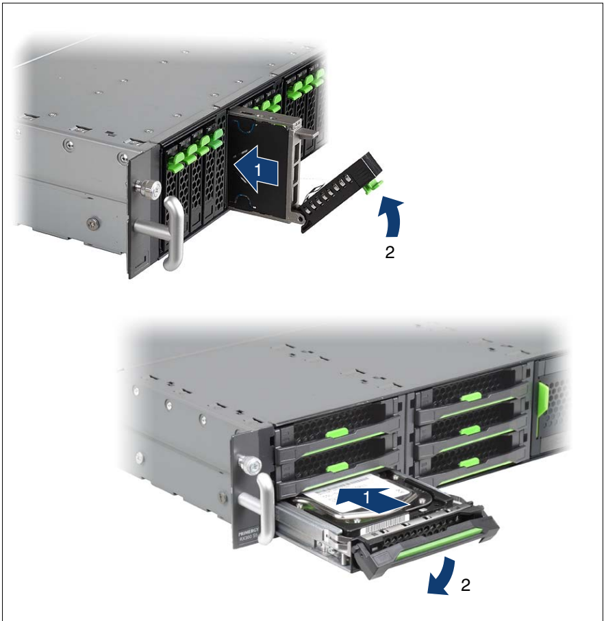
Figure 33: Installing the 2.5-inch and 3.5-inch HDD/SSD modules
