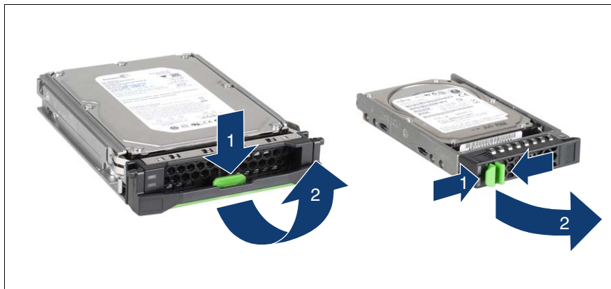
Figure 32: Unlocking the 3.5-inch HDD and 2.5-inch HDD/SSD modules
