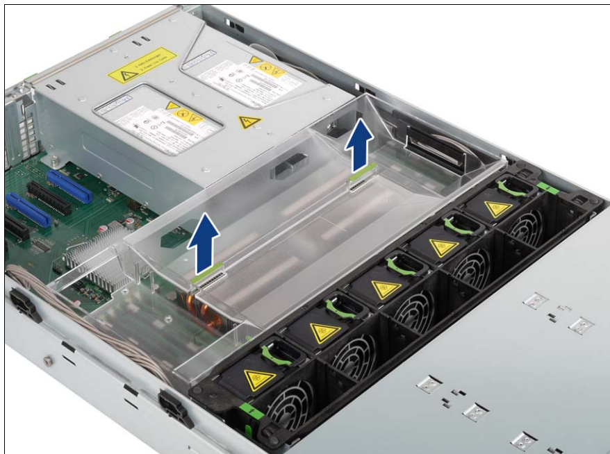
Figure 36: Removing the air duct
