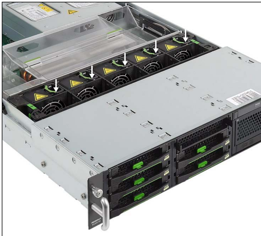
Figure 34: Arrangement of fans and the corresponding indicators
