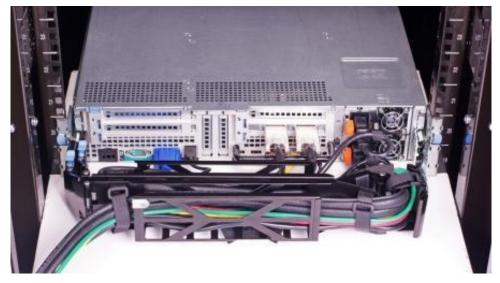
Figure 13. R815 CMA Mounted on the Side Opposite the Power Supplies (Recommended)
