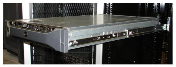
Figure 12. R815 Mounted in the B2 Sliding Rails
