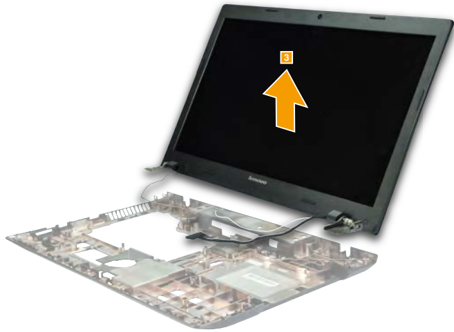
Figure 13. Removal steps of LCD unit (continued)
