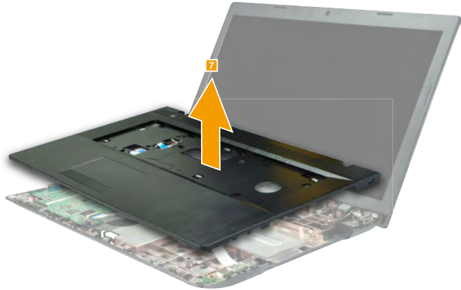
Figure 9. Removal steps of keyboard bezel (continued)
