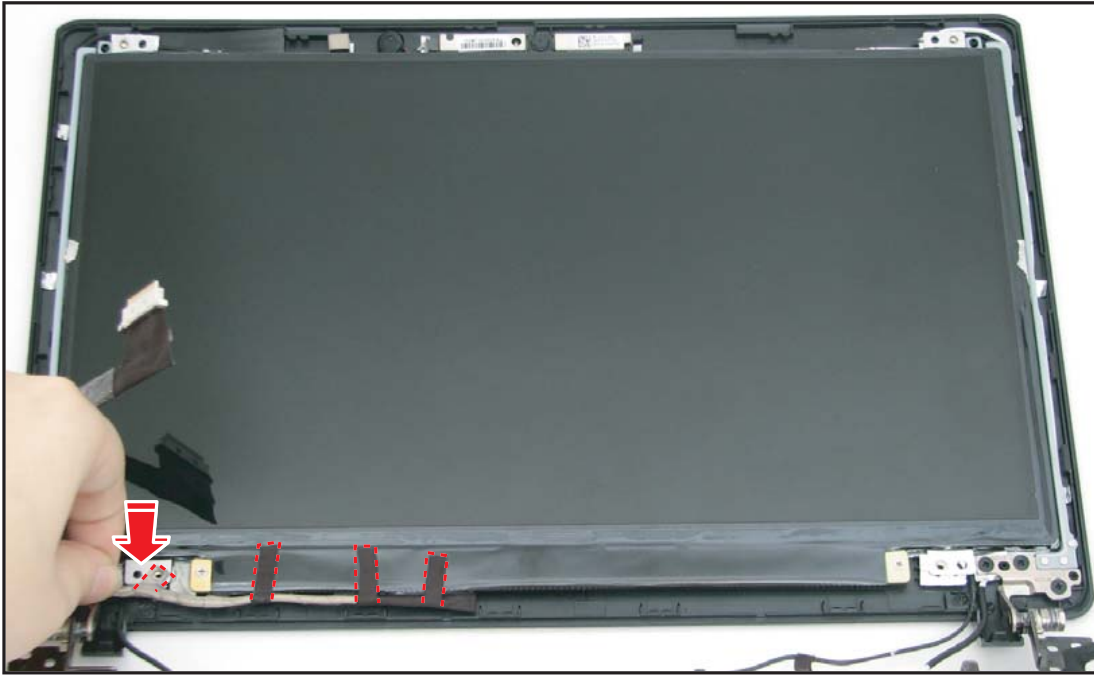
Figure 5:122. Attaching the LVDS Cable Adhesives
