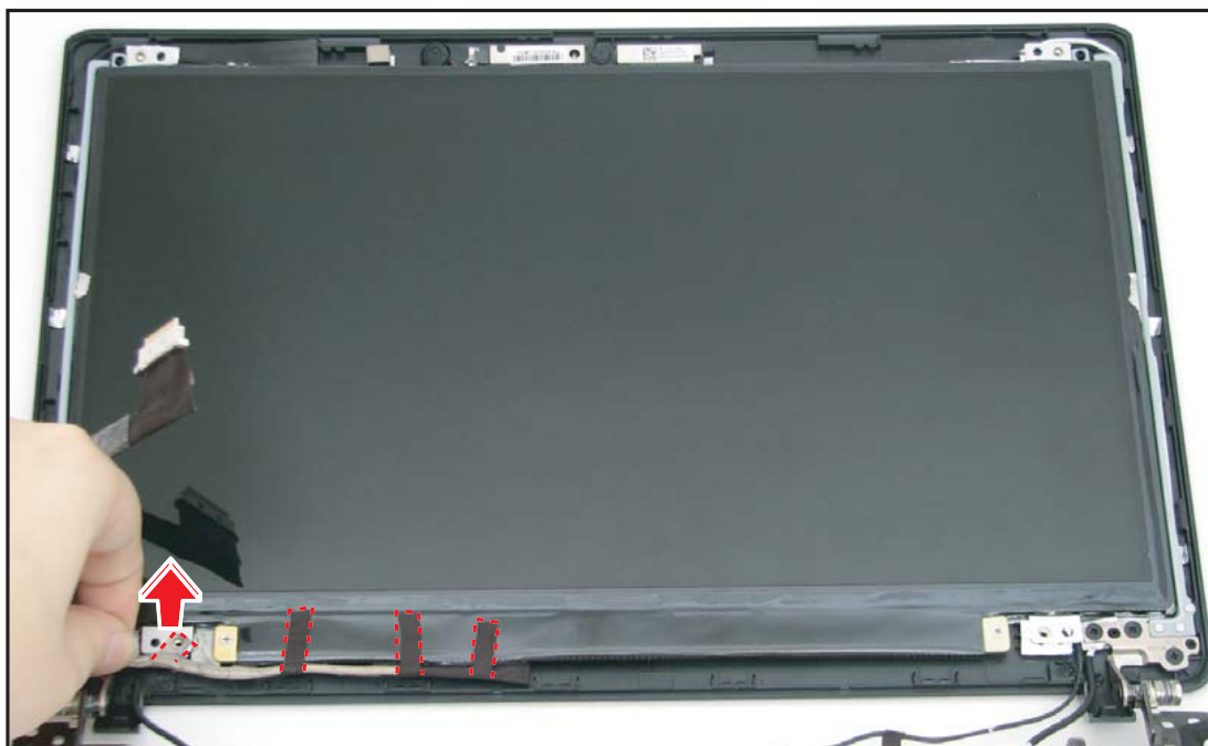
Figure 5:109. Removing the LVDS Cable Adhesives
