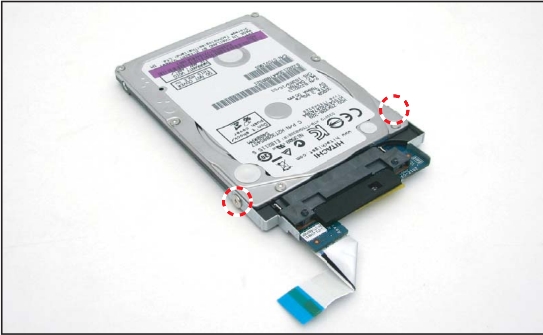
Figure 5:22. Installing the HDD Bracket
