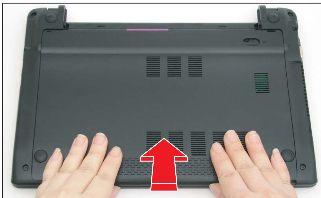
Figure 5:11. Installing the Base Door
