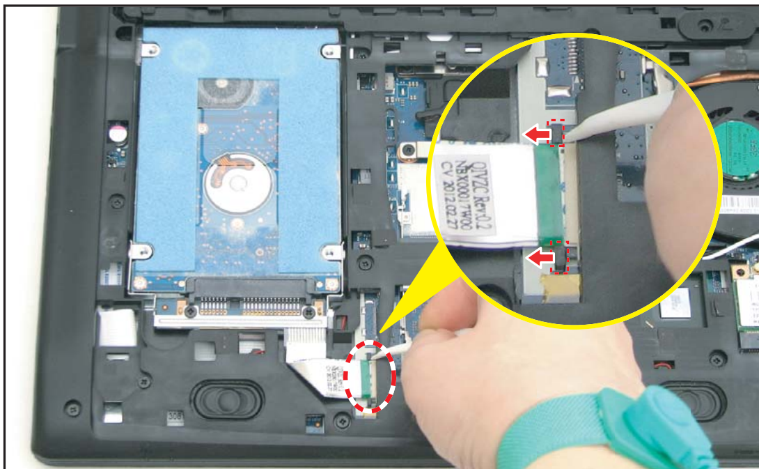
Figure 5:13. Disconnecting the HDD Cable
