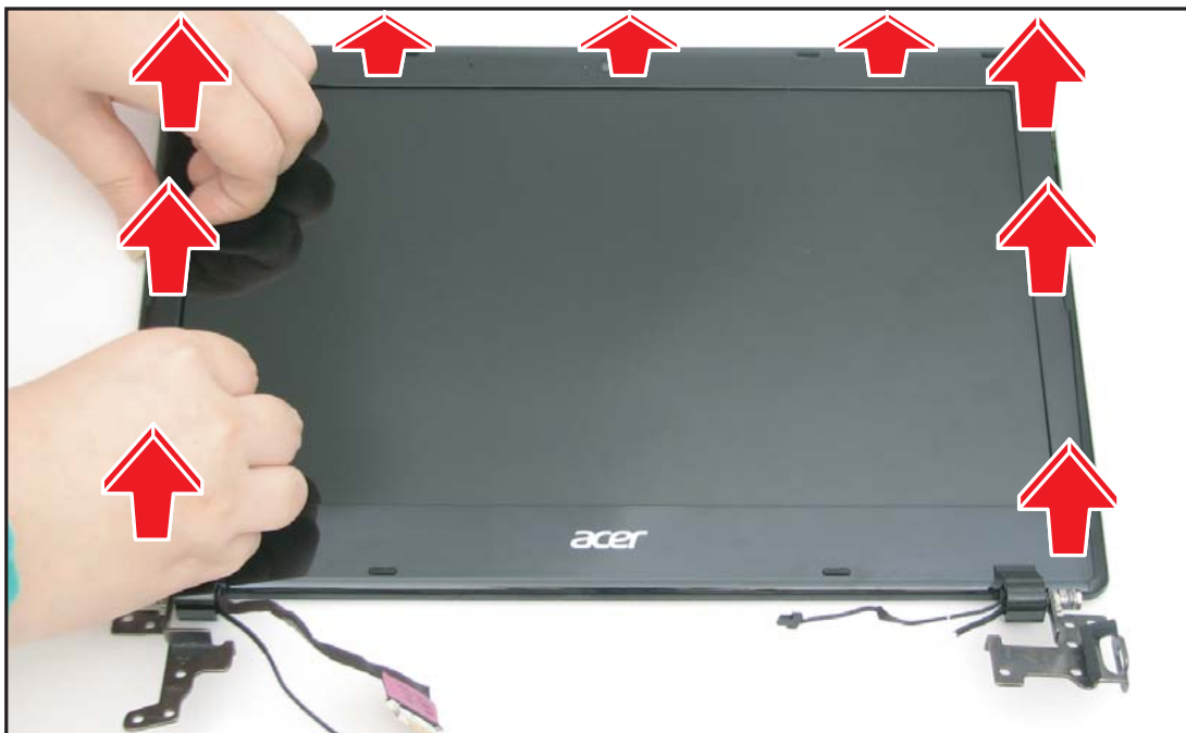
Figure 5:102. Removing the LCD Bezel (1 of 3)
