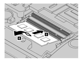
**Note:** If only one memory module is to be installed, install it in the bottom slot.
