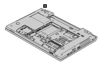
6. Insert a screwdriver into the screw hole, and then push the optical drive 5 to remove it.
