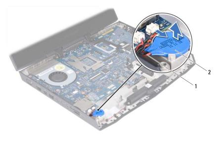
1 coin-cell battery cable 2 coin-cell battery
