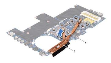
1 thermal cooling assembly 2 captive screws (7)
